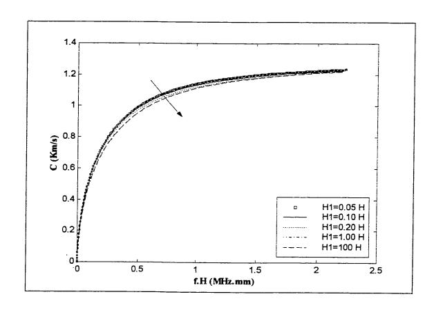
Figure 3.14: Dispersion curves for the 3-ply laminated plate along  $90^{\circ}$  direction for water/plate/water system,  $H_2=100H$ , for various values of  $H_1$
