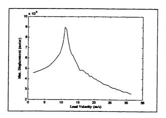
Figure 3.42: Maximum displacement versus the 5 Hz load velocity for the isotropic plate, with elastic foundation stiffness
