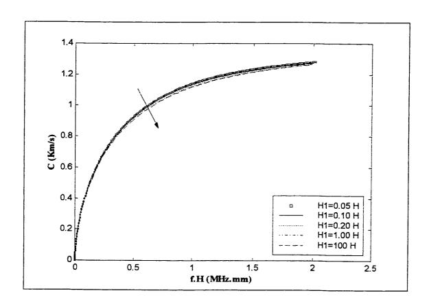
Figure 3.9: Dispersion curves for the 3-ply laminated plate along  $0^{\circ}$  direction for water/plate/water system,  $H_2 = 0.05H$ , for various values of  $H_1$
