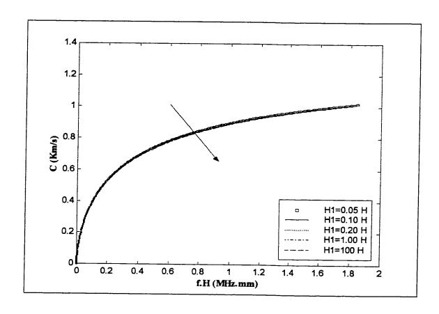
Figure 3.2: Dispersion curves for the 3-ply laminated plate along  $45^{\circ}$  direction for water/plate/mercury system,  $H_2 = 100H$ , for various water depths
