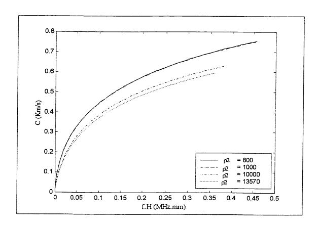
Figure 3.20: Dispersion curves for the 3-ply laminated plate along  $0^{\circ}$  direction for various  $\rho_2$  values ( $\rho_1 = 13,570 \ Kg/m^3$ )
