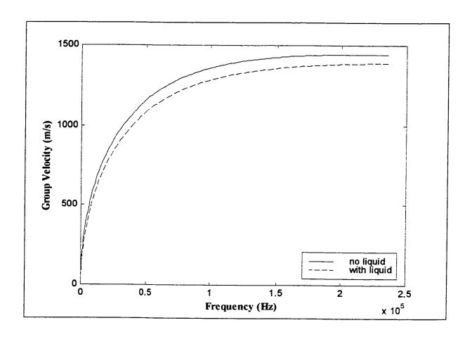
Figure 3.35: The group velocity of the 6-ply plate along the 0° direction with and without the liquid loading
