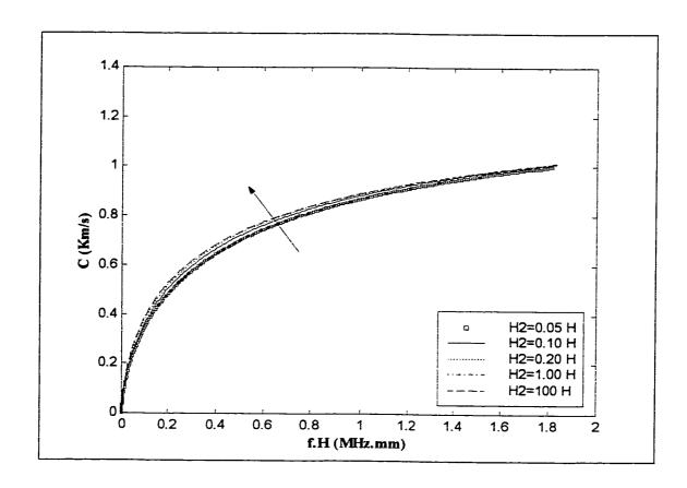
Figure 3.7: Dispersion curves for the 3-ply laminated plate along  $45^{\circ}$  direction for mercury/plate/water system,  $H_1 = 100H$ , for various water depths
