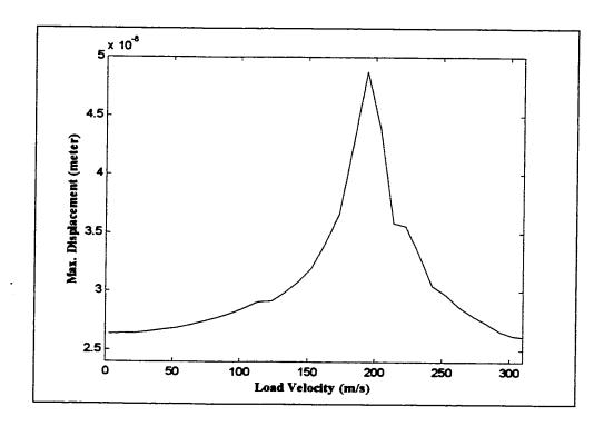
Figure 3.39: Maximum displacement versus load velocity for 150 mm thick plate
