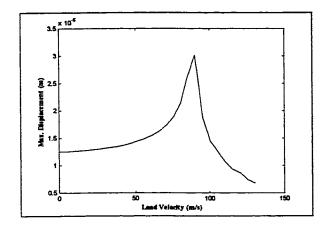
Figure 3.48: Maximum displacement versus the 5 Hz load velocity for the 6-ply laminated plate, with foundation stiffness
