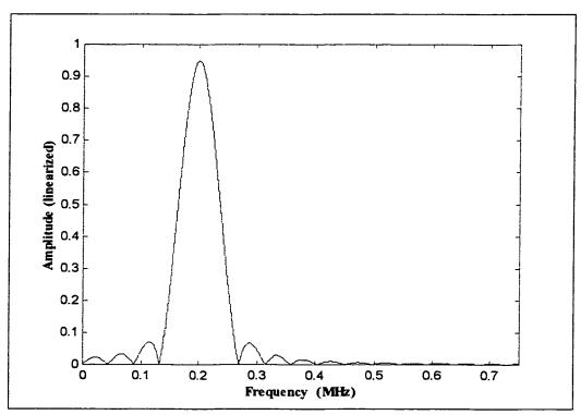
Figure 3.21: The excitation force used with its power spectrum
