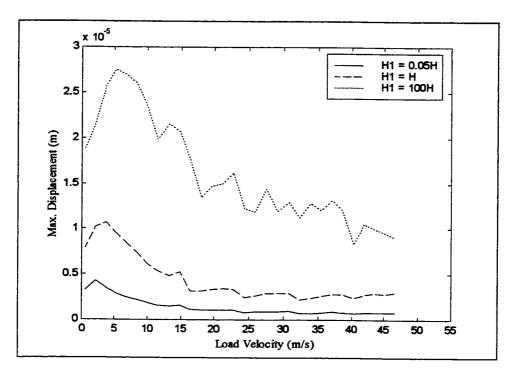
Figure 3.54: The upper liquid depth (H<sub>1</sub>) effect on the maximum displacement versus load velocity curve for the isotropic plate
