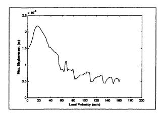
Figure 3.52: Maximum displacement versus the 50 Hz load velocity for the 6-ply laminated plate, with the lower water loading, without foundation stiffness
