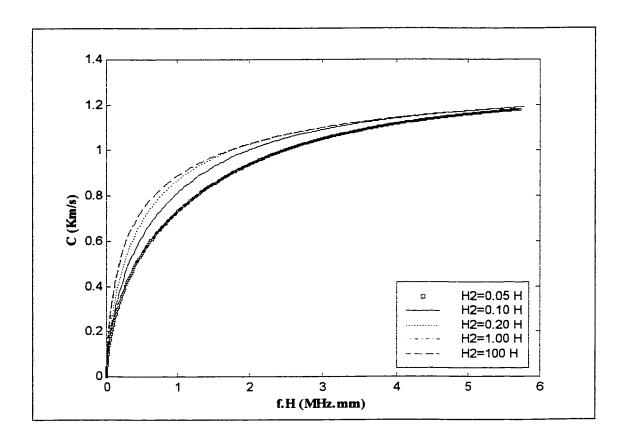
Figure 3.4: Dispersion curves for the 3-ply laminated plate along  $45^{\circ}$  direction for water/plate/mercury system,  $H_1 = 100H$ , for various mercury depths
