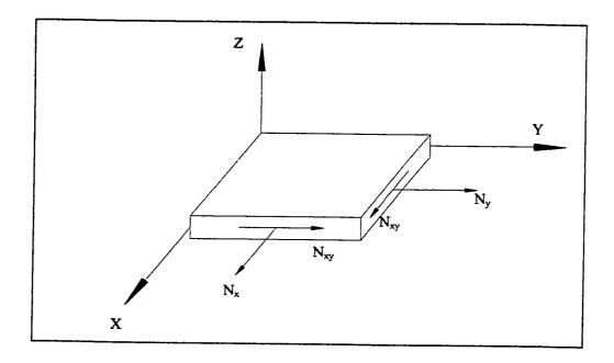
Figure 2.6: Resultant stress on a plate
