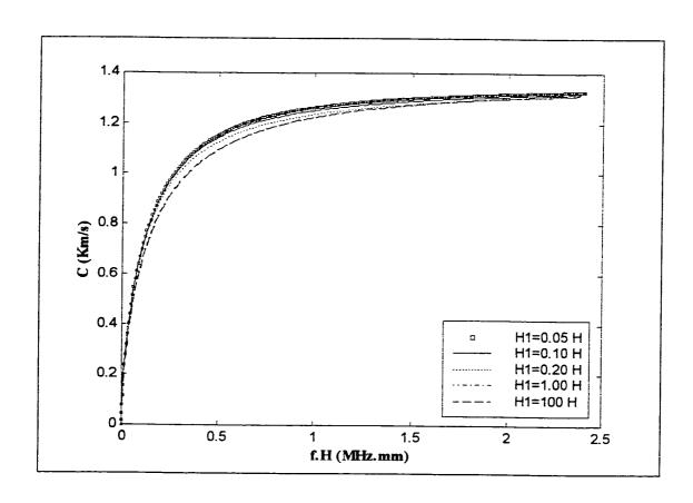
Figure 3.10: Dispersion curves for the 3-ply laminated plate along  $0^{\circ}$  direction for water/plate/water system,  $H_2 = 100H$ , for various values of  $H_1$
