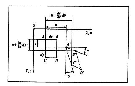
Figure 2.4: Angular distortion.
