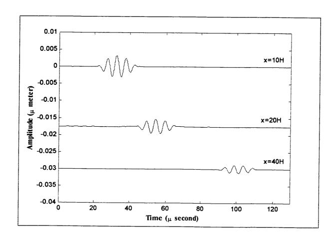
Figure 3.29: The transient response of the 12-ply plate along the 0° direction, at three different locations
