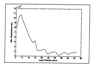
Figure 3.46: Maximum displacement versus the 50 Hz load velocity for the isotropic plate, with the lower water loading, without foundation stiffness
