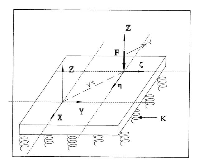
Figure 2.9: Geometric representation of a plate exposed to a moving load on elastic foundation
