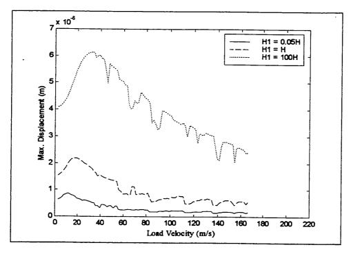
Figure 3.55: The upper liquid depth effect (H<sub>1</sub>) on the maximum displacement versus load velocity curve for the 6-ply laminated plate
