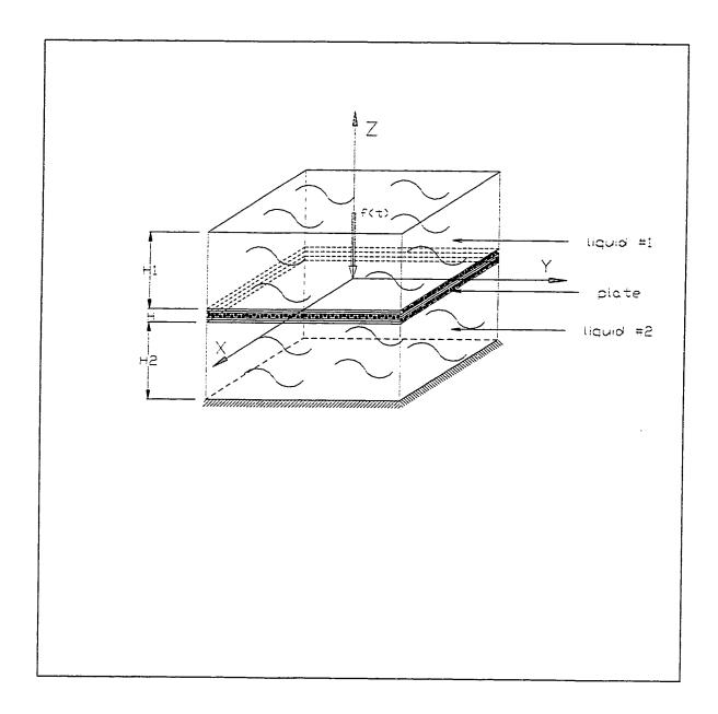
Figure 2.1: Geometric representation of a fluid loaded composite plate
