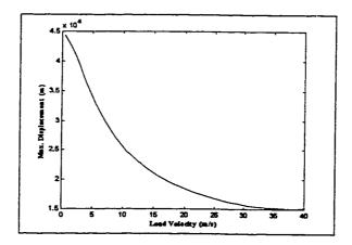
Figure 3.44: Maximum displacement versus the 5 Hz load velocity for the isotropic plate, with both foundation stiffness and water loading
