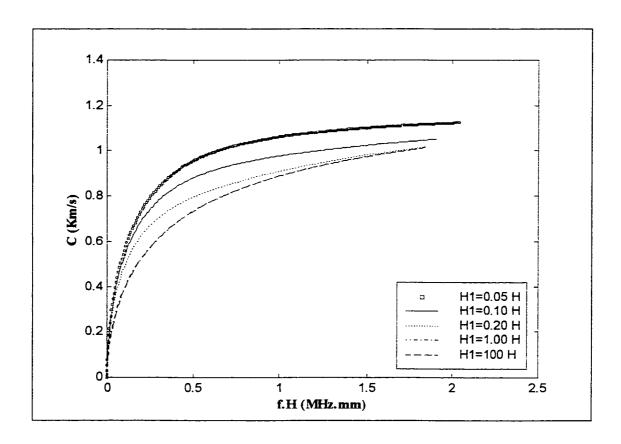
Figure 3.5: Dispersion curves for the 3-ply laminated plate along  $45^{\circ}$  direction for mercury/plate/water system,  $H_2 = 100H$ , for various mercury depths
