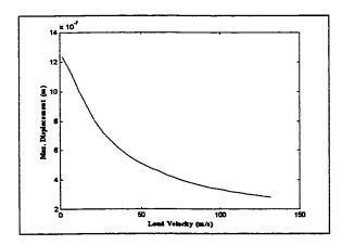
Figure 3.50: Maximum displacement versus the 5 Hz load velocity for the 6-ply laminated plate, with both foundation stiffness and water loading
