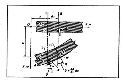
Figure 2.3: Section before and after deflection.
