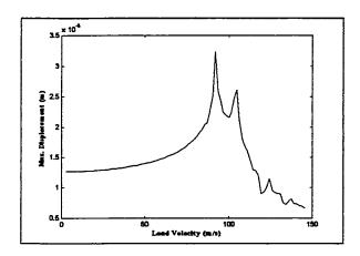
Figure 3.51: Maximum displacement versus the 50 Hz load velocity for the 6-ply laminated plate, with foundation stiffness
