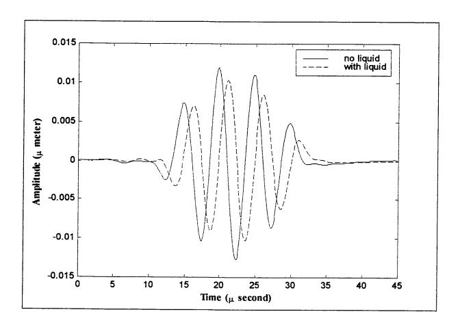
Figure 3.34: The transient response of the 6-ply plate along the 0° direction, with and without the liquid loading
