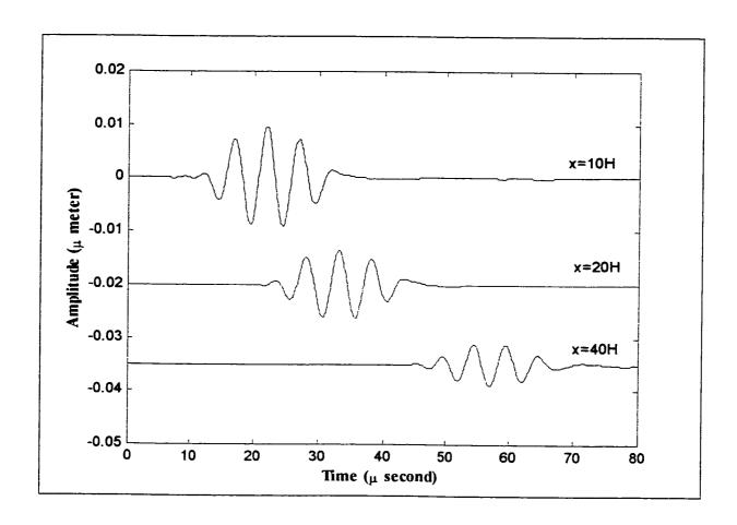
Figure 3.28: The transient response of the 6-ply plate along the 90° direction, at three different locations
