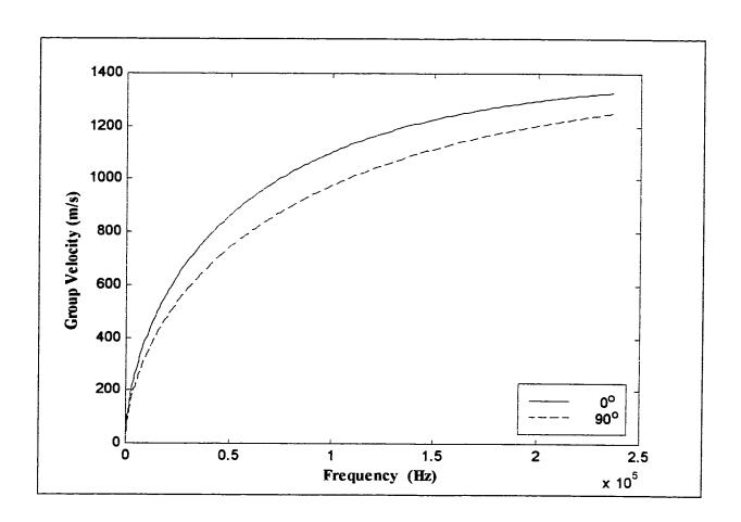
Figure 3.25: The group velocity of the 3-ply plate along the 0° and the 90° directions
