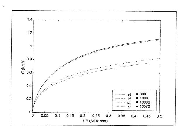
Figure 3.17: Dispersion curves for the 3-ply laminated plate along 0° direction for various  $\rho_1$  values ( $\rho_2 = 800 \ Kg/m^3$ )
