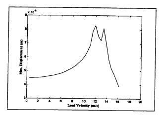
Figure 3.45: Maximum displacement versus the 50 Hz load velocity for the isotropic plate, with foundation stiffness
