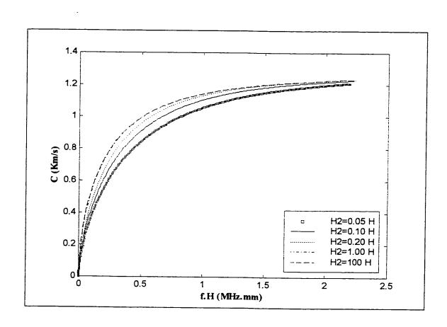
Figure 3.16: Dispersion curves for the 3-ply laminated plate along 90° direction for water/plate/water system,  $H_1 = 0.05H$ , for various values of  $H_2$
