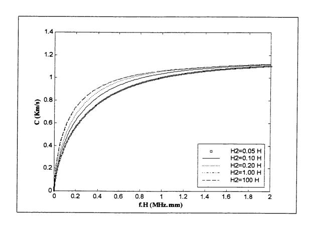
Figure 3.8: Dispersion curves for the 3-ply laminated plate along  $45^{\circ}$  direction for mercury/plate/water system,  $H_1 = 0.05H$ , for various water depths
