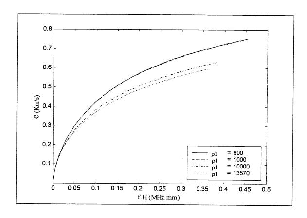
Figure 3.18: Dispersion curves for the 3-ply laminated plate along 0° direction for various  $\rho_1$  values ( $\rho_2 = 13,570 \ Kg/m^3$ )
