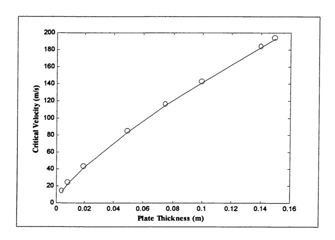
Figure 3.41: Critical velocity versus plate thickness
