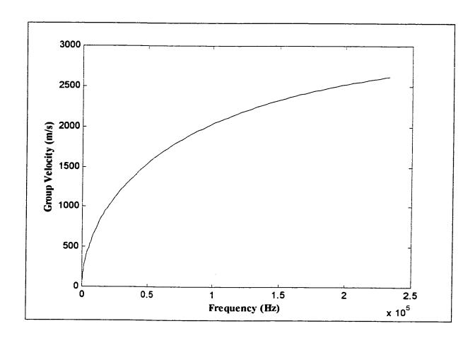
Figure 3.33: The group velocity of the isotropic plate
