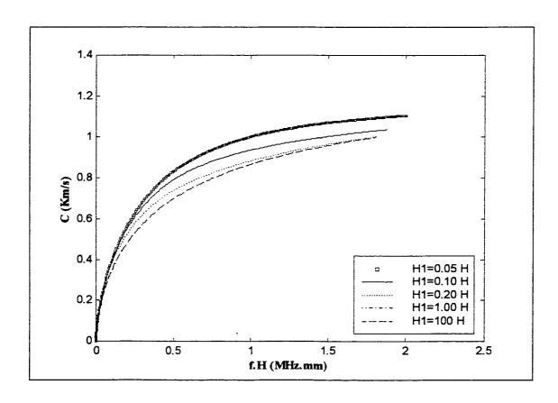
Figure 3.6: Dispersion curves for the 3-ply laminated plate along  $45^{\circ}$  direction for mercury/plate/water system,  $H_2 = 0.05H$ , for various mercury depths
