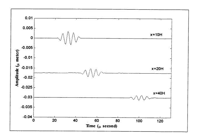
Figure 3.31: The transient response of the 12-ply plate along the 90° direction, at three different locations
