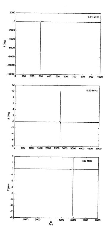
Figure 2.8:  $R\{W_o(\xi_1, 0, \omega)\}$  for a laminated plate for several frequencies
