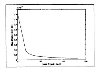
Figure 3.49: Maximum displacement versus the 5 Hz load velocity for the 6-ply laminated plate, with the lower water loading, without foundation stiffness
