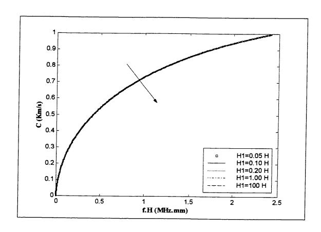
Figure 3.1: Dispersion curves for the 3-ply laminated plate along  $45^{\circ}$  direction for water/plate/mercury system,  $H_2 = 0.05H$ , for various water depths.
