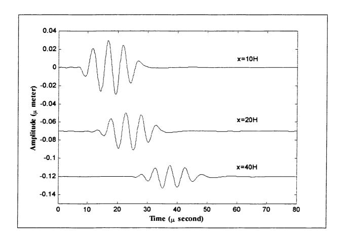
Figure 3.24: The transient response of the 3-ply plate along the 90° direction, at three different locations
