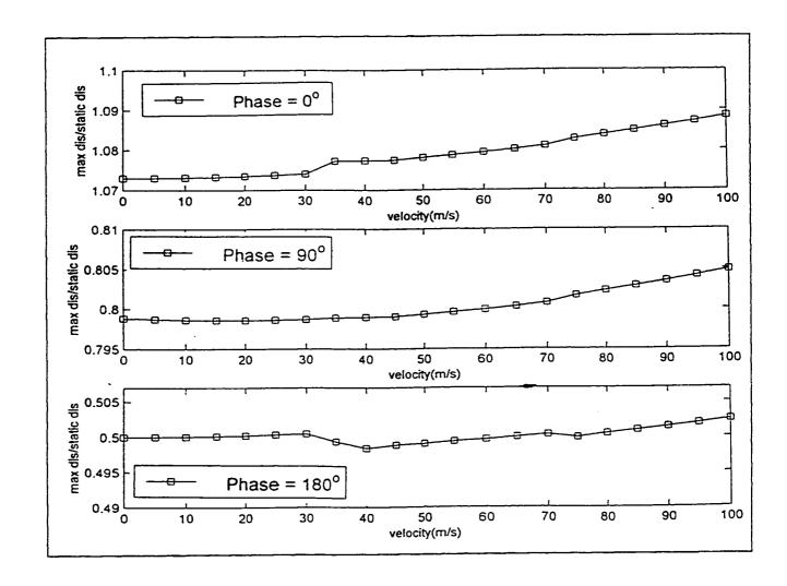
Figure 3.61: Effect of the velocity for 0°, 90° and 180° phase respectively for the 6-ply laminated plate
