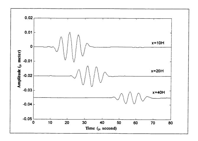
Figure 3.26: The transient response of the 6-ply plate along the 0° direction, at three different locations
