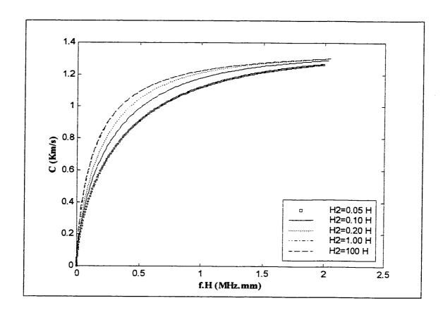
Figure 3.12: Dispersion curves for the 3-ply laminated plate along  $0^{\circ}$  direction for water/plate/water system,  $H_1 = 100H$ , for various values of  $H_2$
