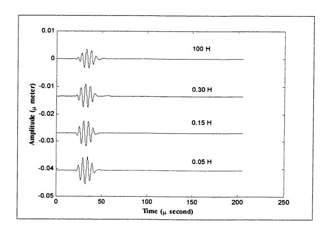
Figure 3.36: The transient response of the 6-ply plate along the  $45^{\circ}$  direction, with several  $H_2$
