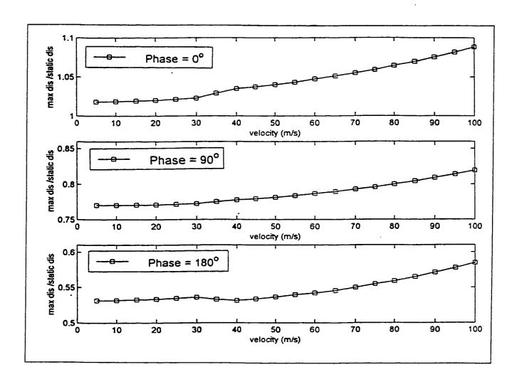
Figure 3.59: Effect of the two moving loads velocity for 0°, 90° and 180° phase respectively for the isotropic plate
