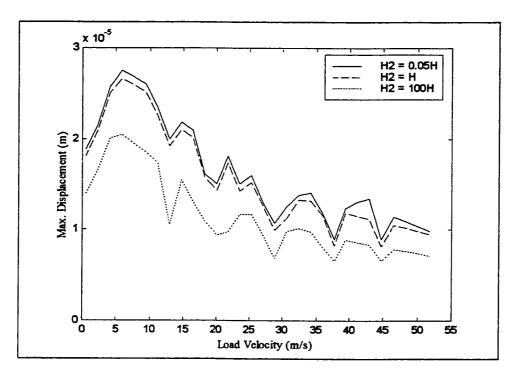
Figure 3.56: The lower liquid depth (H<sub>2</sub>) effect on the maximum displacement versus load velocity curve for the isotropic plate
