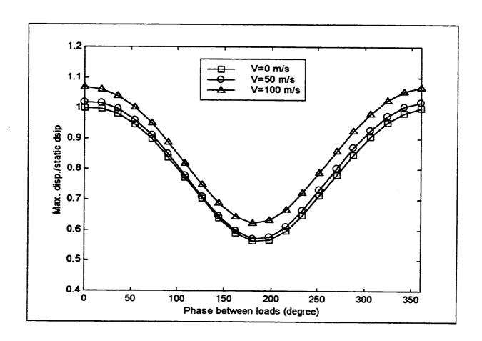
Figure 3.58: Effect of phase difference between the two moving loads on maximum displacement for the isotropic plate
