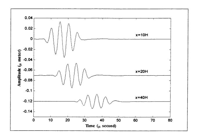
Figure 3.22: The transient response of the 3-ply plate along the 0° direction, at three different locations
