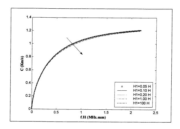
Figure 3.13: Dispersion curves for the 3-ply laminated plate along  $90^{\circ}$  direction for water/plate/water system,  $H_2 = 0.05H$ , for various values of  $H_1$
