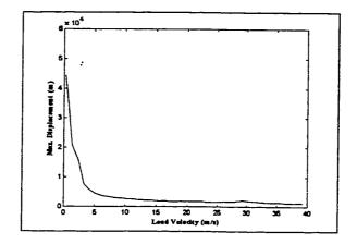
Figure 3.43: Maximum displacement versus the 5 Hz load velocity for the isotropic plate, with the lower water loading, without foundation stiffness
