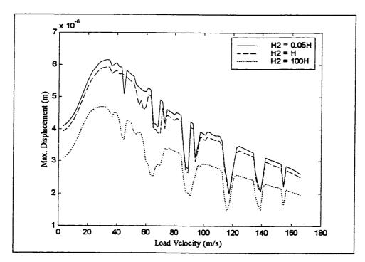
Figure 3.57: The lower liquid depth effect (H<sub>2</sub>) on the maximum displacement versus load velocity curve for the 6-ply laminated plate
