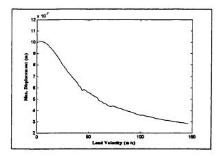
Figure 3.53: Maximum displacement versus the 50 Hz load velocity for the 6-ply laminated plate, with both foundation stiffness and water loading
