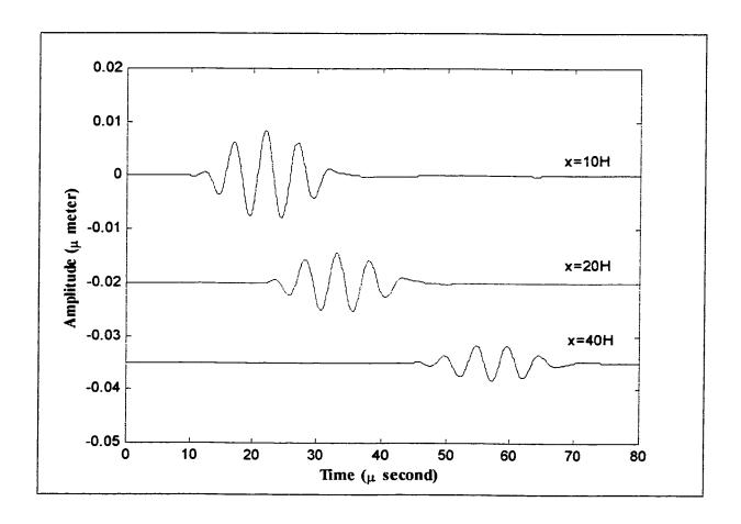
Figure 3.27: The transient response of the 6-ply plate along the 45° direction, at three different locations
