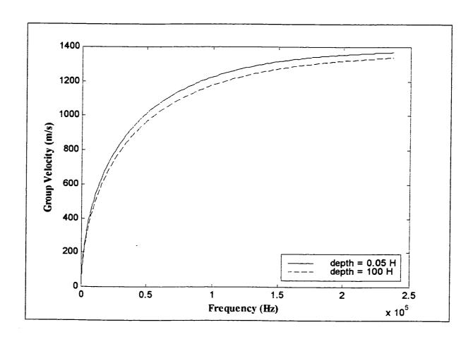
Figure 3.38: The group velocity of the 6-ply plate for  $H_2=0.05H$ , and  $H_2=100H$
