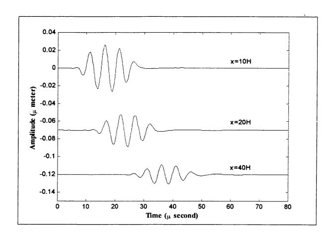
Figure 3.23: The transient response of the 3-ply plate along the 45° direction, at three different locations
