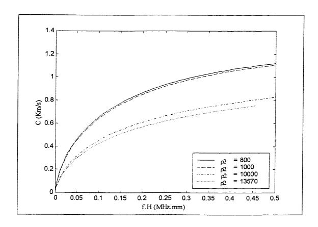
Figure 3.19: Dispersion curves for the 3-ply laminated plate along 0° direction for various  $\rho_2$  values ( $\rho_1 = 800 \text{ Kg/m}^3$ )
