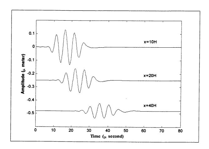
Figure 3.32: The transient response of the isotropic plate at three different locations
