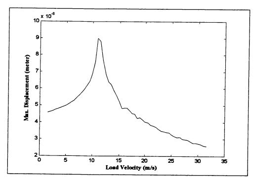
Figure 3.40: Maximum displacement versus load velocity for 4 mm thick plate
