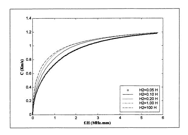
Figure 3.3: Dispersion curves for the 3-ply laminated plate along  $45^{\circ}$  direction for water/plate/mercury system,  $H_1 = 0.05H$ , for various mercury depths
