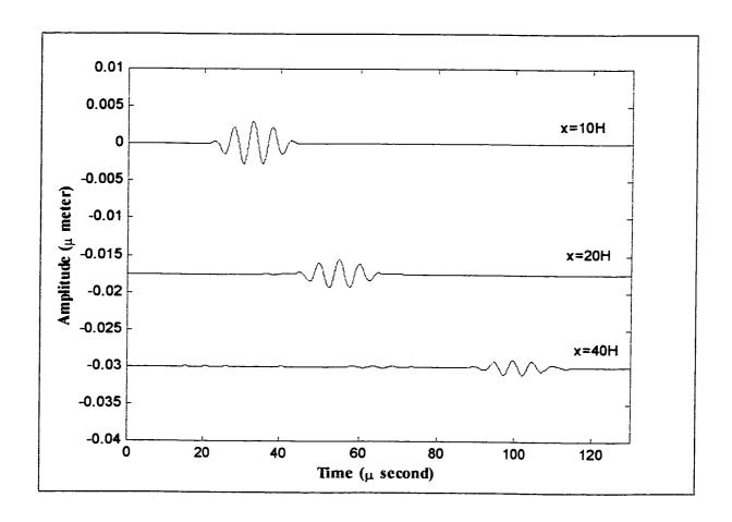
Figure 3.30: The transient response of the 12-ply plate along the 45° direction, at three different locations
