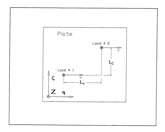
Figure 2.10: Geometric Representation of a plate exposed to two moving loads
