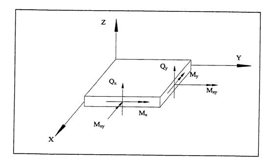
Figure 2.5: Moment and transverse shear resultant on a plate
