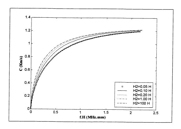
Figure 3.15: Dispersion curves for the 3-ply laminated plate along  $90^{\circ}$  direction for water/plate/water system,  $H_1 = 100H$ , for various values of  $H_2$
