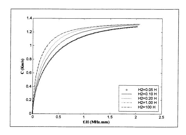
Figure 3.11: Dispersion curves for the 3-ply laminated plate along  $0^{\circ}$  direction for water/plate/water system,  $H_1 = 0.05H$ , for various values of  $H_2$
