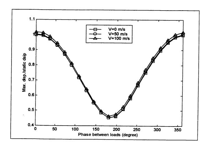
Figure 3.60: Effect of phase between the two loads on maximum displacement for the 6-ply laminated plate
