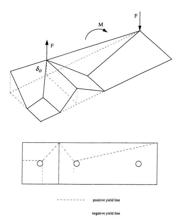
Figure 7.11 Thin-Plate Mode of Failure (Mode 2)
