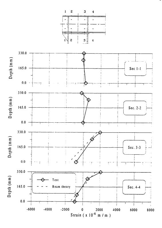
Figure 6.32 Normal Strain Distribution for Specimen C2 at M = 307 kNm
