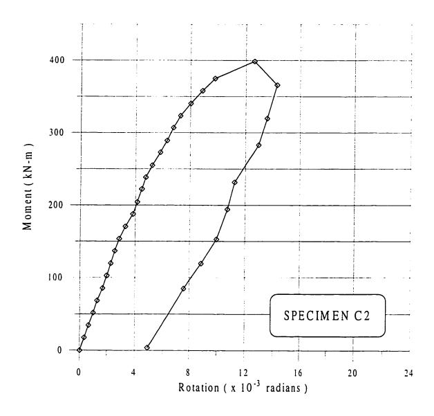
Figure 6.28 Moment-Rotation Relationship for Specimen C2
