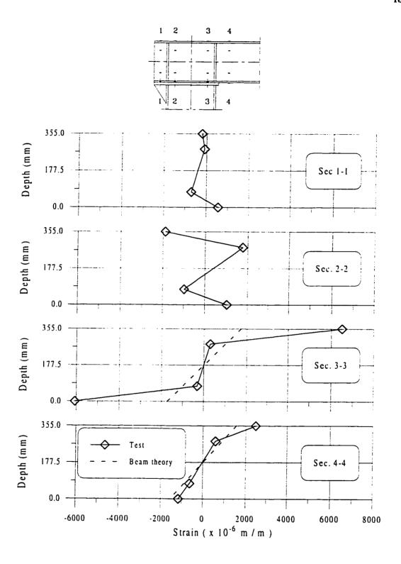
Figure 6.46 Normal Strain Distribution for Specimen C4 at M = 414 kNm
