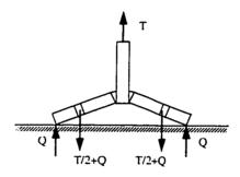
Bolt failure with flange yielding
