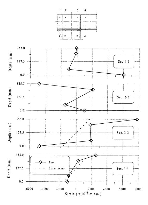
Figure 6.52 Normal Strain Distribution for Specimen C5 at M = 396 kNm
