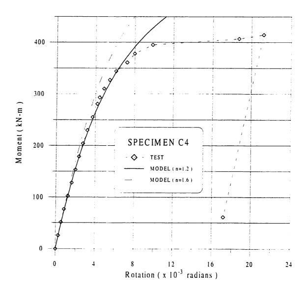
Figure 7.16 Moment - Rotation Model for Specimen C4
