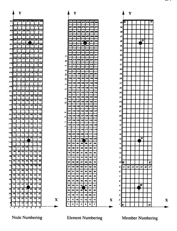
Figure 7.6 Finite Element Mesh for Beam Bottom Flange PL1 (Width = 160 mm)
