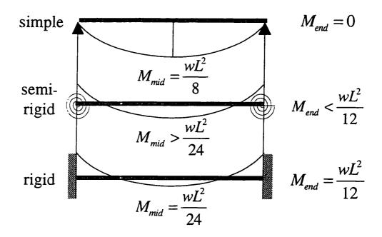
Figure 1.1 Pinned, Semi-Rigid and Rigid Connections
