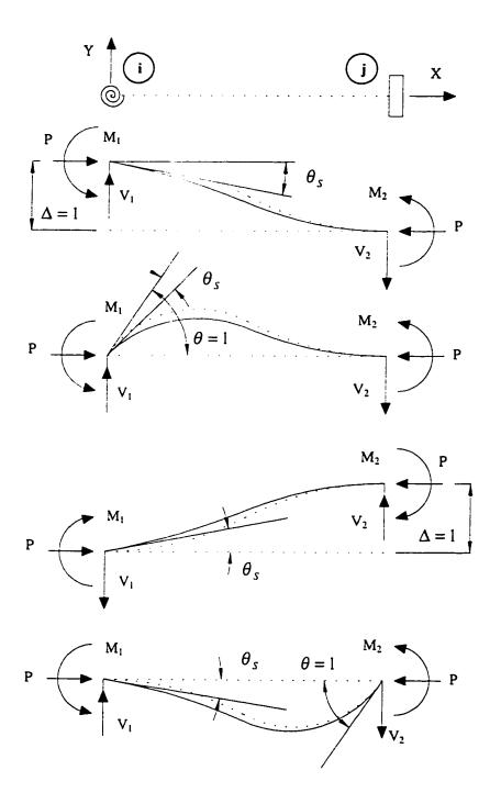
Figure 3.4 Unit Displacements and Rotations at the i and j Ends
