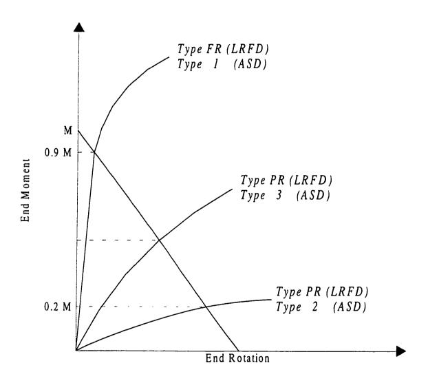
Figure 2.1 Moment-Rotation Characteristics of AISC Connection Types
