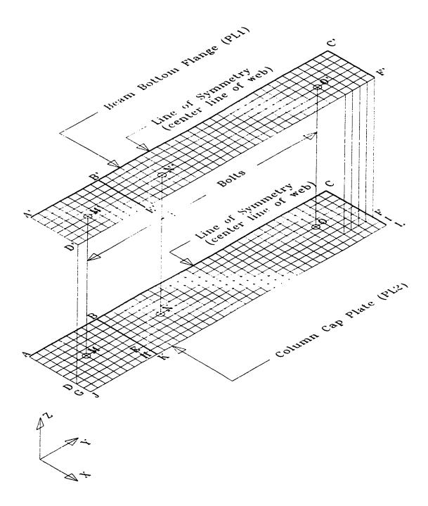
Figure 7.4 Finite Element Model Discretization
