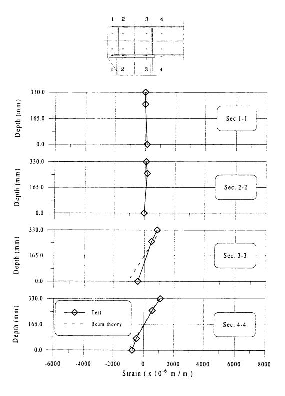
Figure 6.31 Normal Strain Distribution for Specimen C2 at M = 204 kNm
