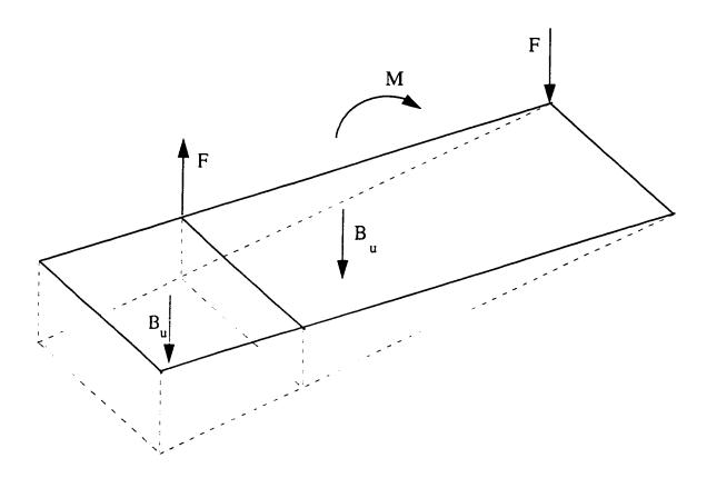
Figure 7.10 Thick-Plate Mode of Failure (Mode 1)
