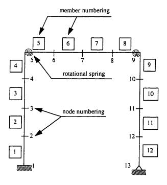
Figure 6.8 Frame Discretization and Numbering
