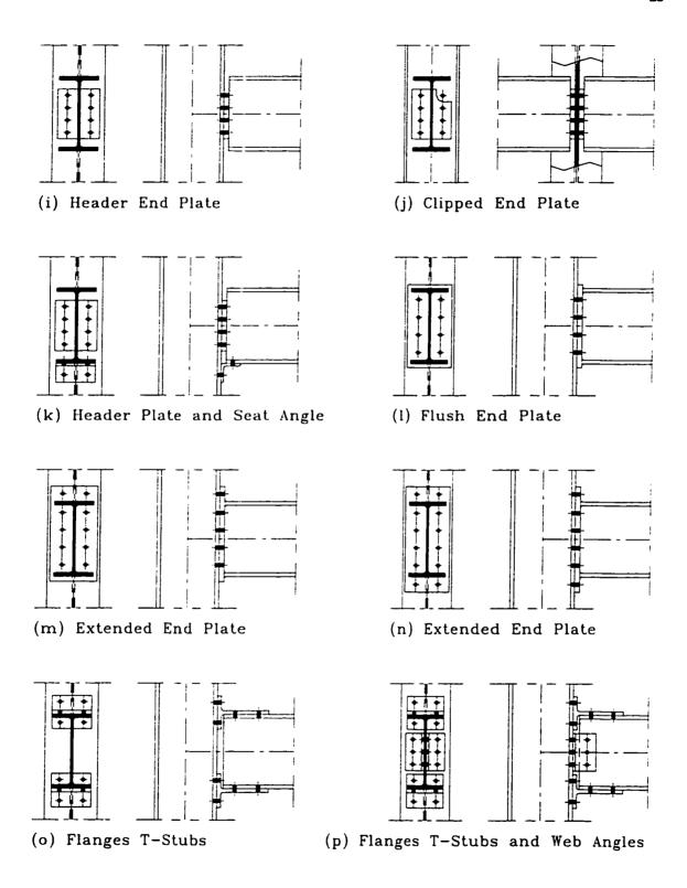
Figure 2.4 Types of Building Beam-Column Connections (cont.)
