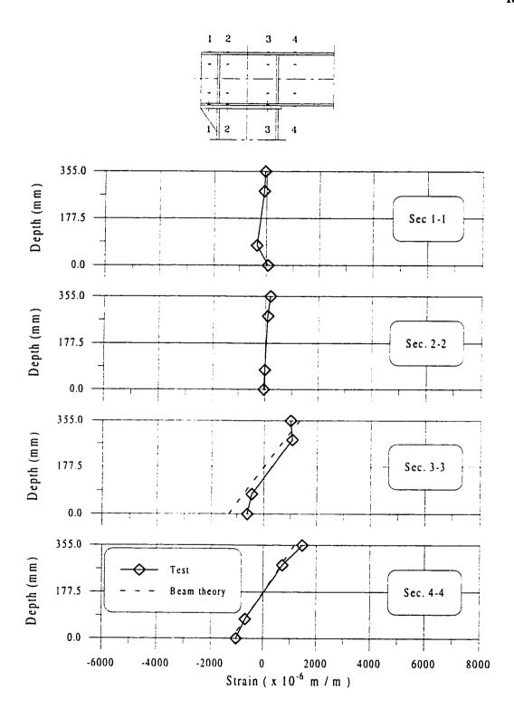
Figure 6.45 Normal Strain Distribution for Specimen C4 at M = 293 kNm
