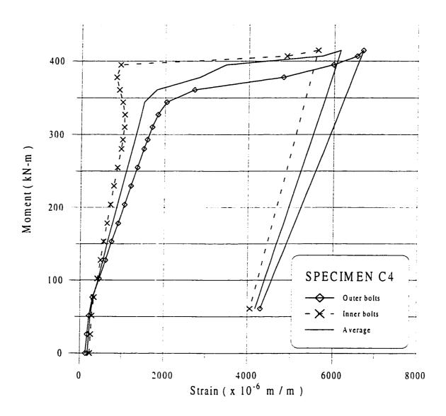
Figure 6.42 Bolts Strains for Specimen C4
