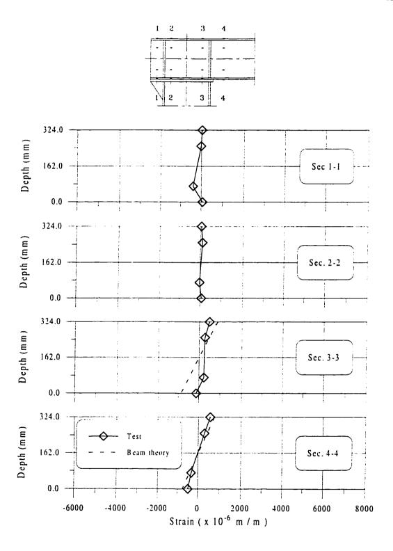
Figure 6.36 Normal Strain Distribution for Specimen C3 at M = 95 kNm
