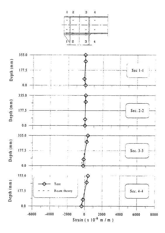
Figure 6.43 Normal Strain Distribution for Specimen C4 at M = 102 kNm
