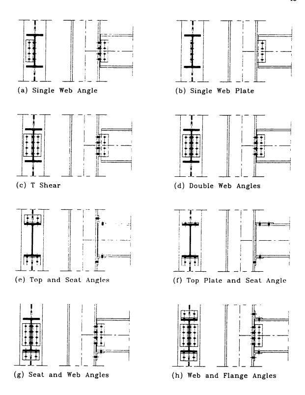
Figure 2.4 Types of Building Beam-Column Connections
