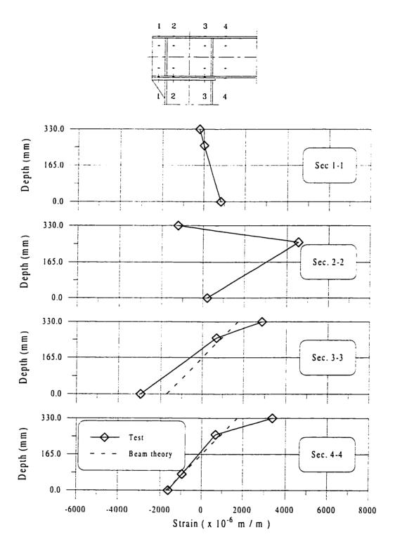
Figure 6.33 Normal Strain Distribution for Specimen C2 at M = 398 kNm
