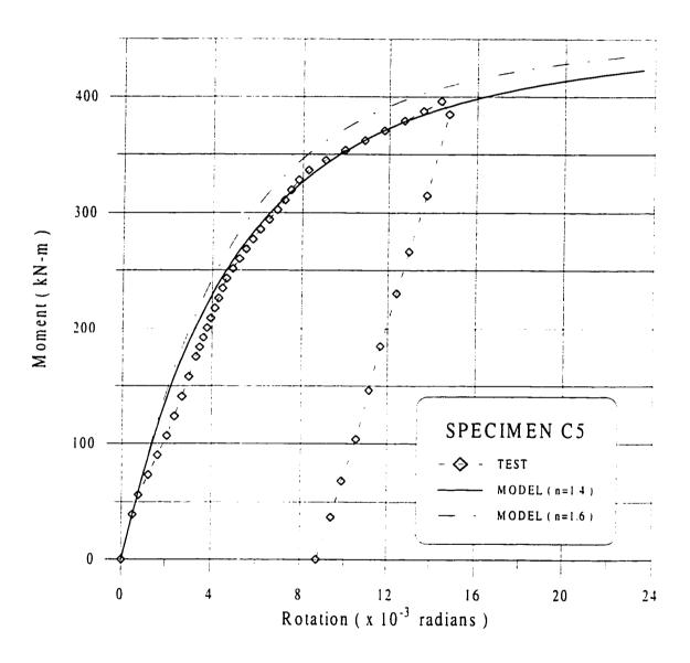
Figure 7.17 Moment - Rotation Model for Specimen C5
