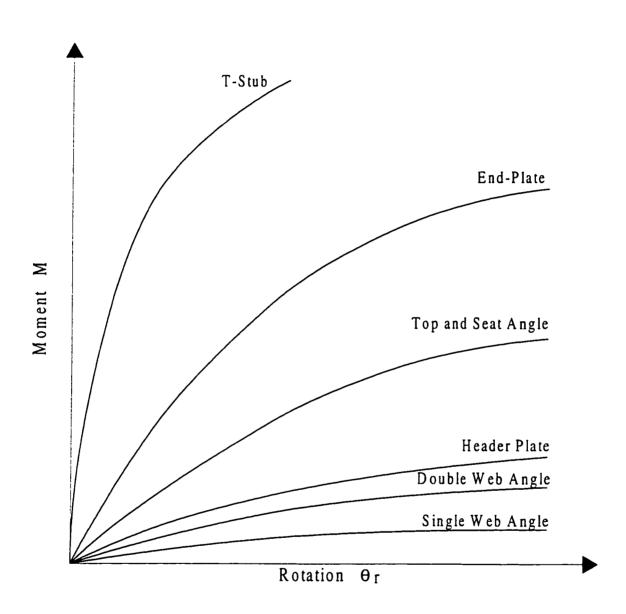
Figure 2.5 Comparison of Moment-Rotation Relation for Different Joints
