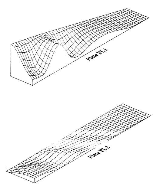
Figure 7.8 Deflected Shapes for Plates PL1 and PL2
