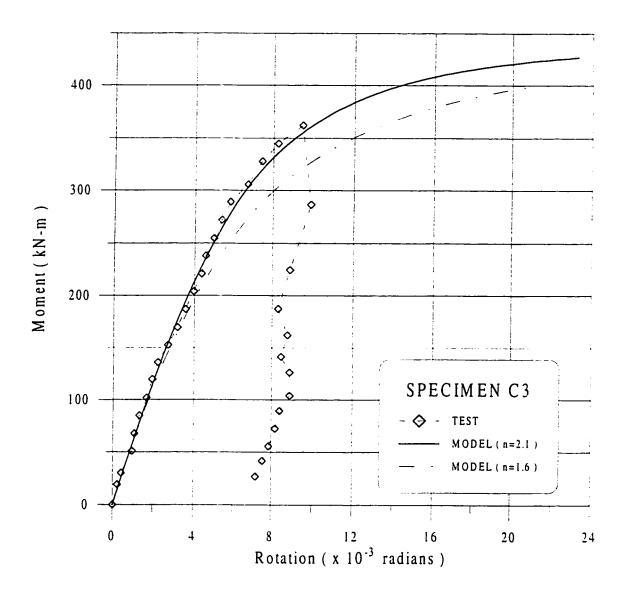
Figure 7.15 Moment - Rotation Model for Specimen C3
