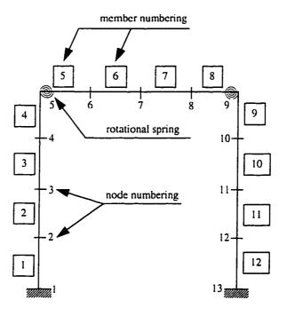
Figure 6.2 Frame Discretization and Numbering
