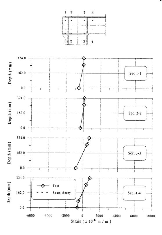
Figure 6.23 Normal Strain Distribution for Specimen C1 at M = 127 kNm
