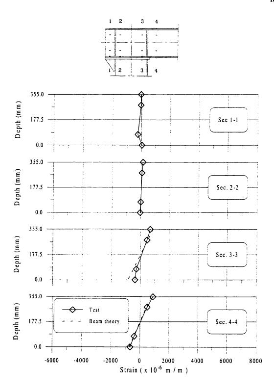
Figure 6.44 Normal Strain Distribution for Specimen C4 at M = 204 kNm
