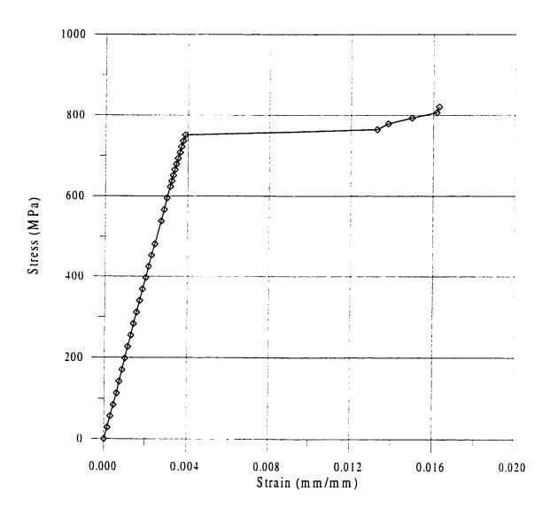
Figure 6.20 Typical Bolt Stress-Strain Relationship
