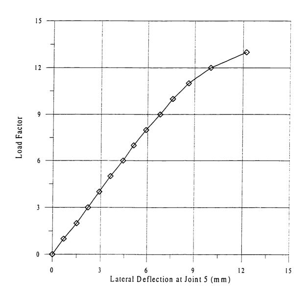
Figure 6.17 Effect of Plastic Hinges Formation on the Load-Deflection
