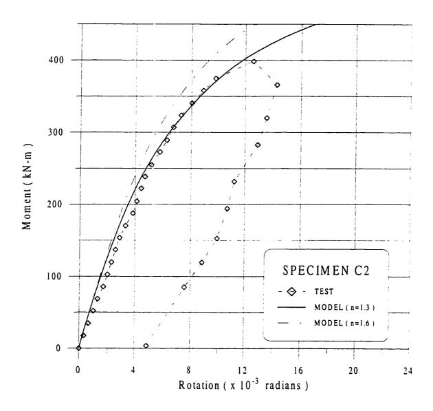
Figure 7.14 Moment - Rotation Model for Specimen C2
