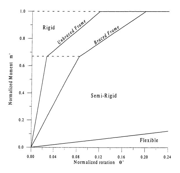
Figure 2.3 Classification of Connections According to Eurocode 3
