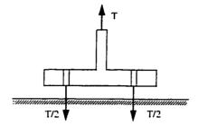
Bolt failure (thick plates / weak bolts)
