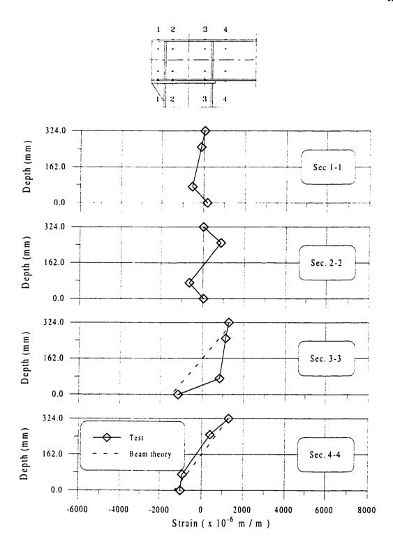
Figure 6.37 Normal Strain Distribution for Specimen C3 at M = 203 kNm
