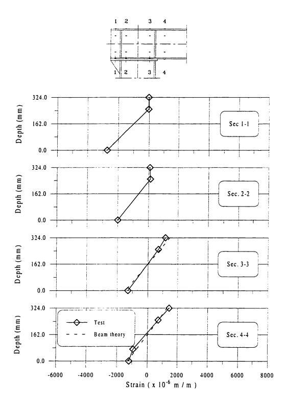
Figure 6.24 Normal Strain Distribution for Specimen C1 at M = 213 kNm
