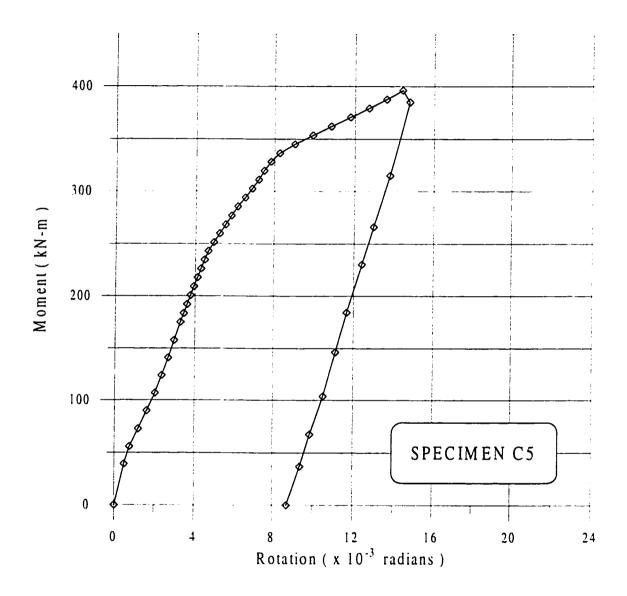
Figure 6.47 Moment-Rotation Relationship for Specimen C5
