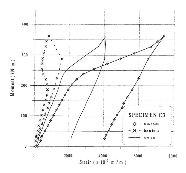
Figure 6.35 Bolts Strains for Specimen C3
