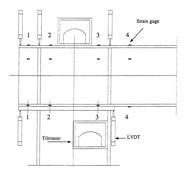
Figure 5.12 Instrumentation Locations
