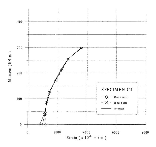
Figure 6.22 Bolts Strains for Specimen C1
