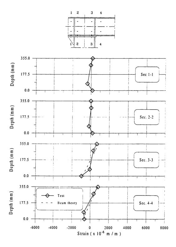
Figure 6.50 Normal Strain Distribution for Specimen C5 at M = 200 kNm
