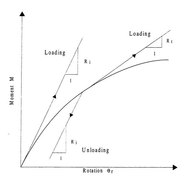
Figure 2.6 Loading and Unloading Paths of Semi-Rigid Connections
