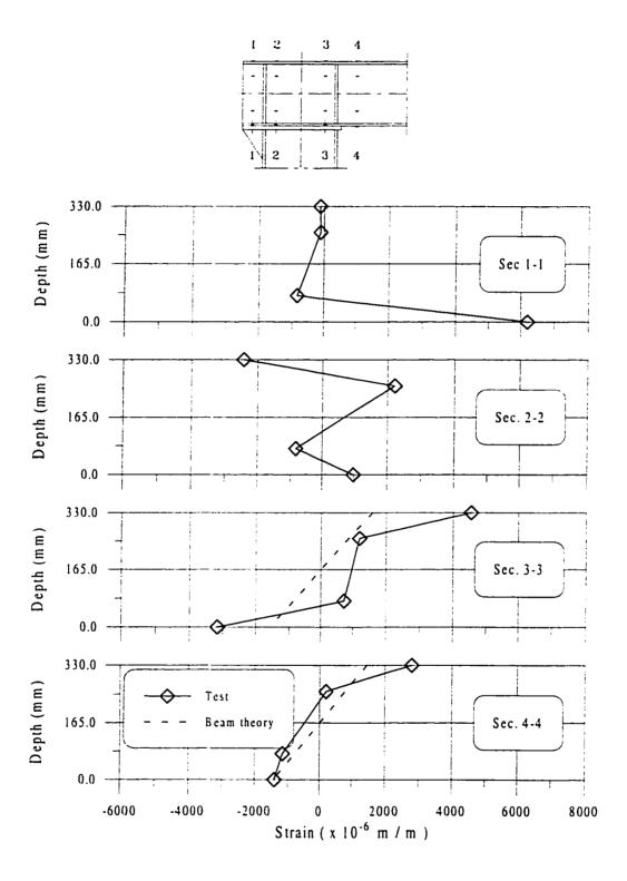
Figure 6.57 Normal Strain Distribution for Specimen C6 at M = 314 kNm
