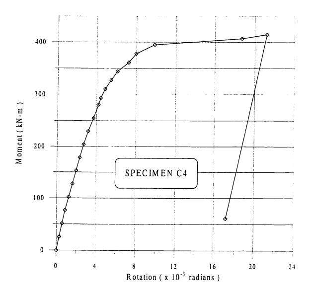
Figure 6.41 Moment-Rotation Relationship for Specimen C4
