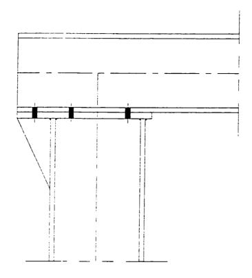
Figure 1.3 Cap Plate Connection
