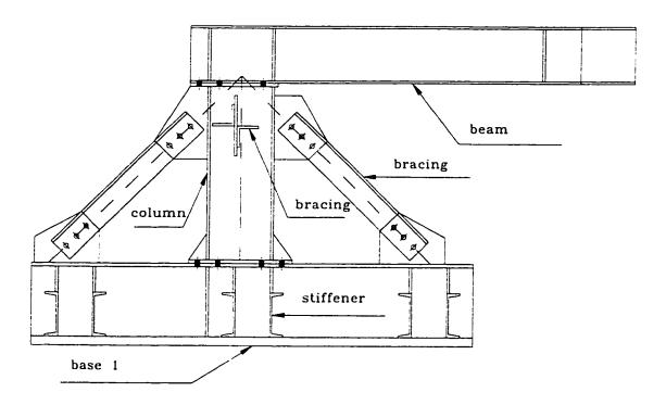
Figure 5.6 Bracing System
