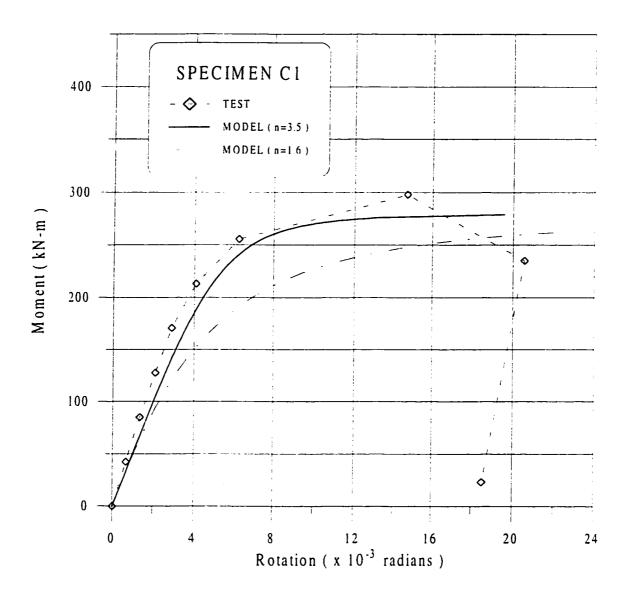
Figure 7.13 Moment - Rotation Model for Specimen C1
