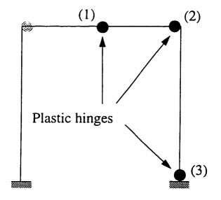
Figure 6.16 Sequence of Plastic Hinges Formation
