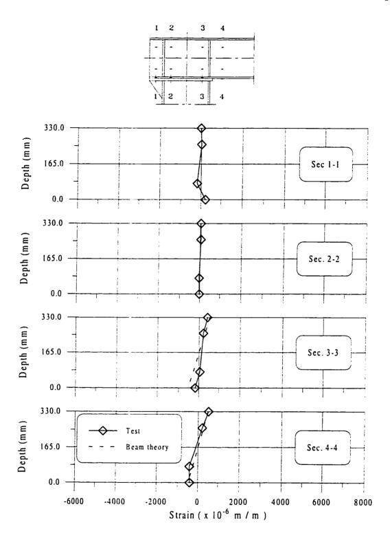
Figure 6.55 Normal Strain Distribution for Specimen C6 at M = 102 kNm
