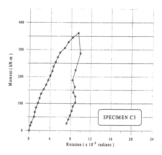
Figure 6.34 Moment-Rotation Relationship for Specimen C3
