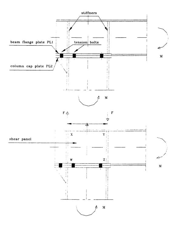
Figure 7.2 Typical Cap-Plate Connection
