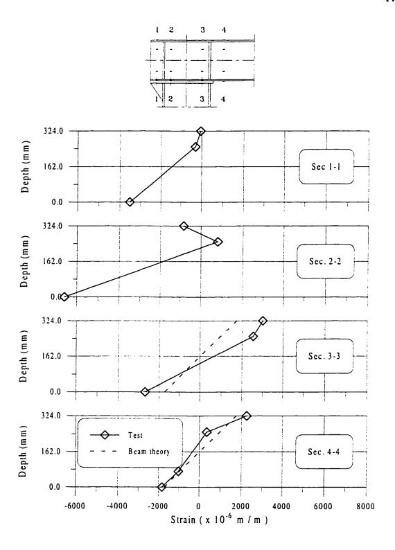
Figure 6.25 Normal Strain Distribution for Specimen C1 at M = 298 kNm
