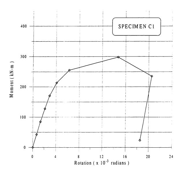
Figure 6.21 Moment-Rotation Relationship for Specimen C1
