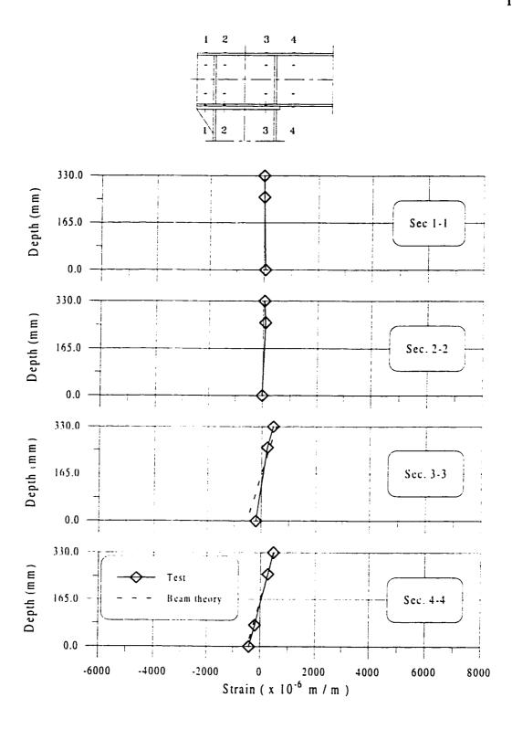
Figure 6.30 Normal Strain Distribution for Specimen C2 at M = 102 kNm
