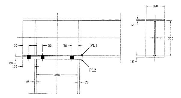
Figure 5.2 Typical Specimen Dimensions
