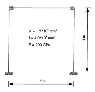
Figure 6.1 Frame Dimensions and Properties
