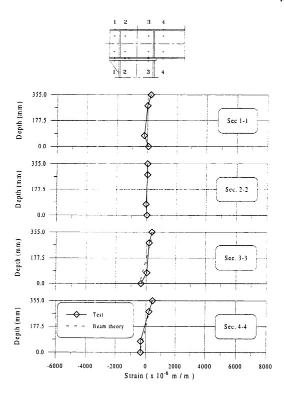
Figure 6.49 Normal Strain Distribution for Specimen C5 at M = 106 kNm
