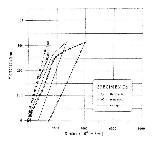
Figure 6.54 Bolts Strains for Specimen C6
