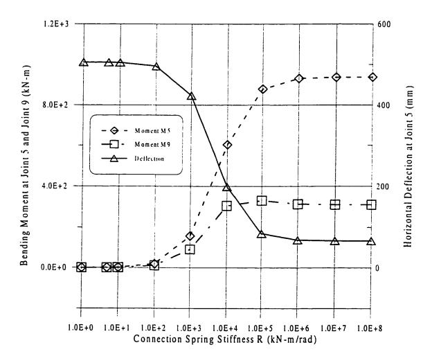
Figure 6.10 Effect of Variation of Connection Spring Stiffness on a Frame
