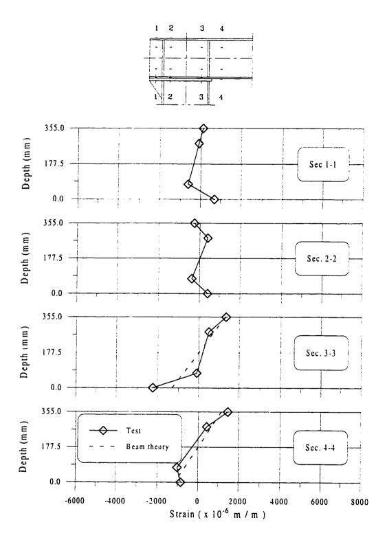
Figure 6.51 Normal Strain Distribution for Specimen C5 at M = 302 kNm
