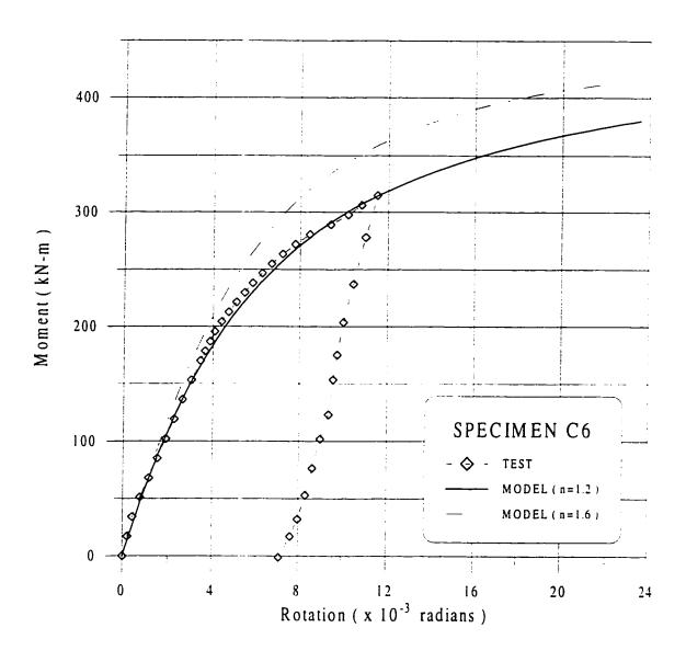
Figure 7.18 Moment - Rotation Model for Specimen C6
