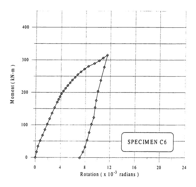
Figure 6.53 Moment-Rotation Relationship for Specimen C6
