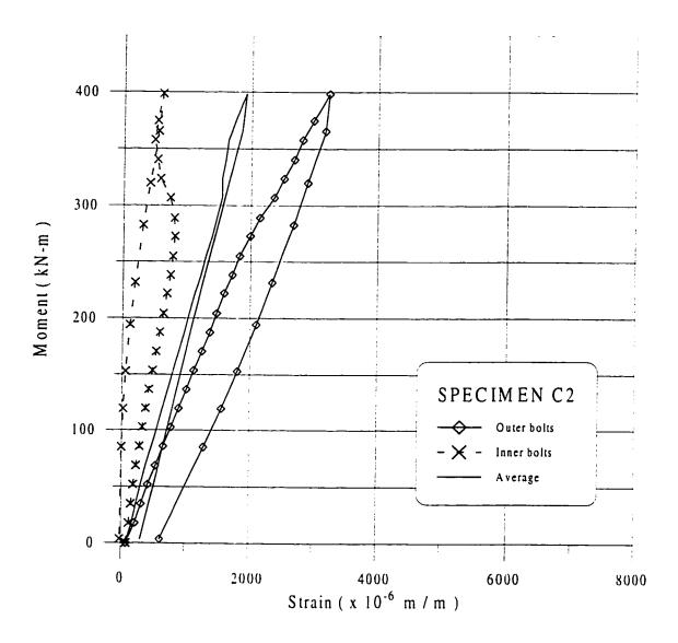
Figure 6.29 Bolts Strains for Specimen C2
