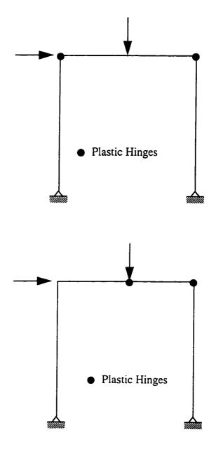
Figure 3.2 Frame Failure by Plastic Mechanism
