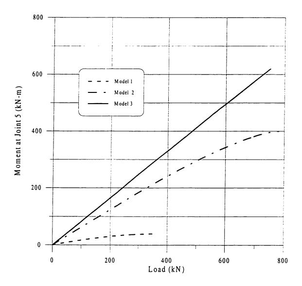
Figure 6.13 Effect of Connection Flexibility on Load-Moment Relationship
