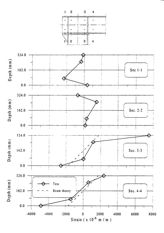
Figure 6.38 Normal Strain Distribution for Specimen C3 at M = 305 kNm
