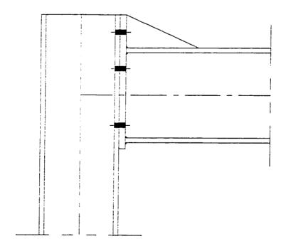
Figure 1.4 Header Plate Connection
