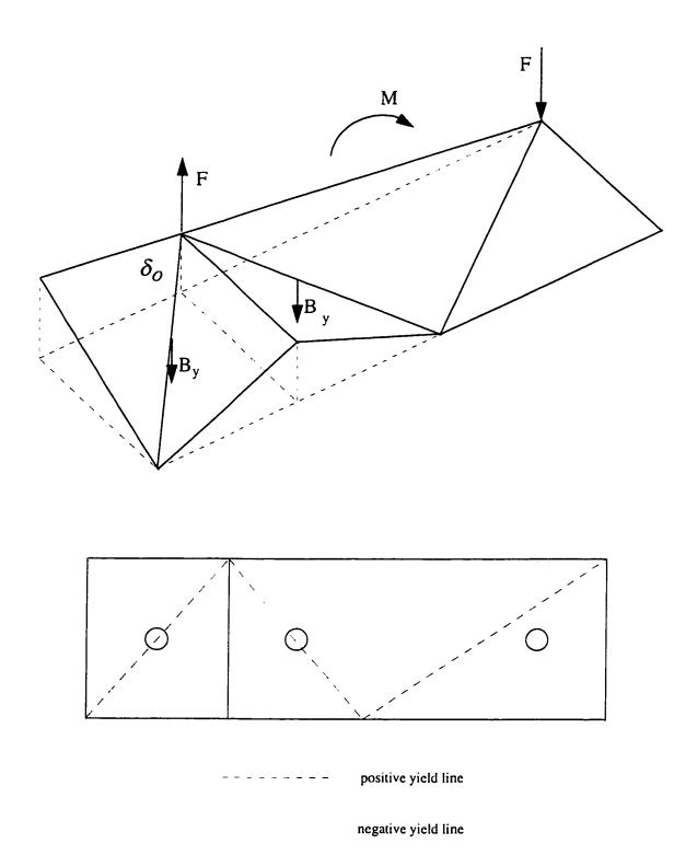
Figure 7.12 Intermediate-Plate Mode of Failure (Mode 3)
