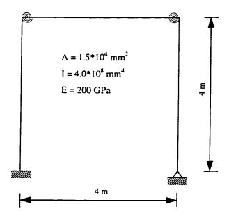
Figure 6.7 Frame Dimensions and Properties
