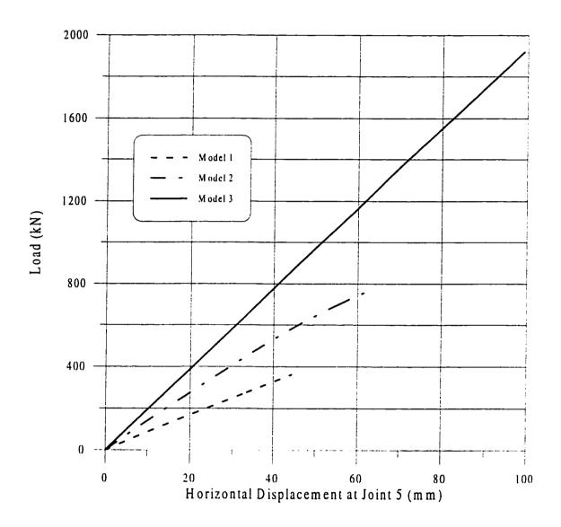
Figure 6.14 Effect of Connection Flexibility on Load-Displacement Relationship
