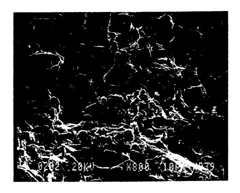
Plate 4.6: Photomicrograph of Sandy Clay Showing Clay Matrix Surrounding Aggregations of Larger Grains. This Sample was compacted at 20% Water Content and allowed to dry.
