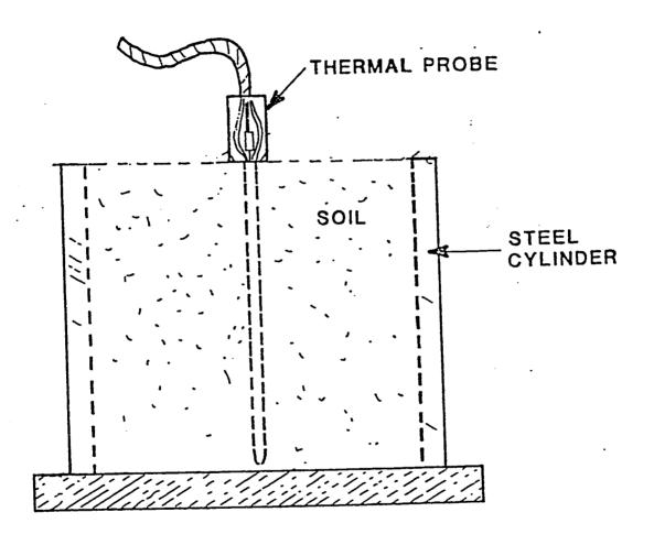
Fig. 3.3: Schematic Diagram of Laboratory Thermal Resistivity Test Arrangement.
