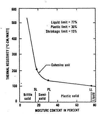
Fig. 2.6: Correlation Between Atterberg Limits and Thermal Resistivity (Salomone and Covax, 1983)
