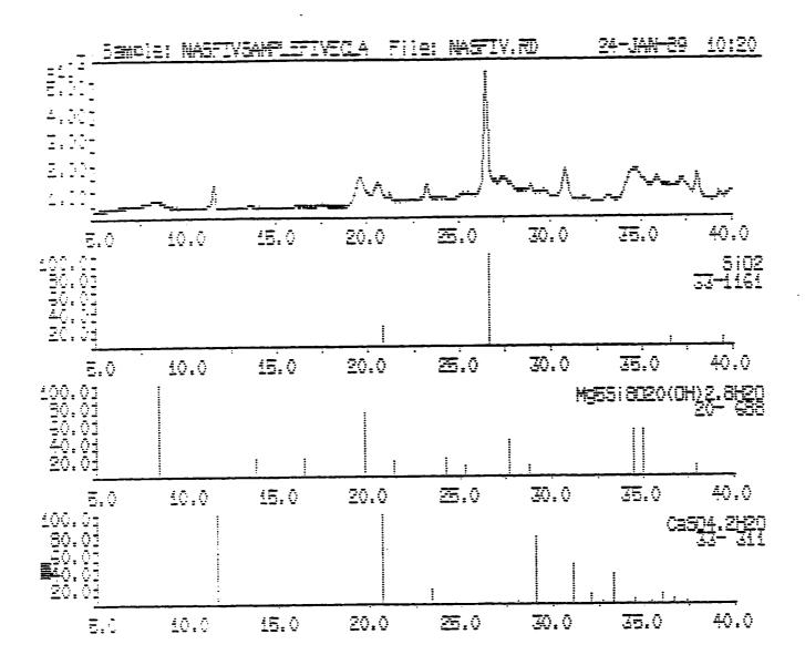
Fig. 6: X-Ray Diffraction Analysis of Sample #9 (Clay)
