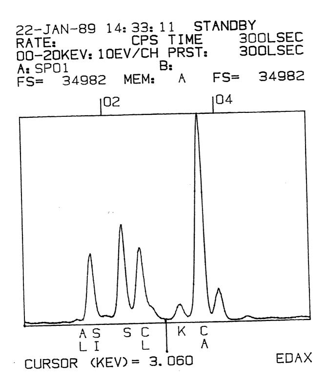
Fig.12: X-Ray Fluorescence Analysis of Sample #7 (Marl)
