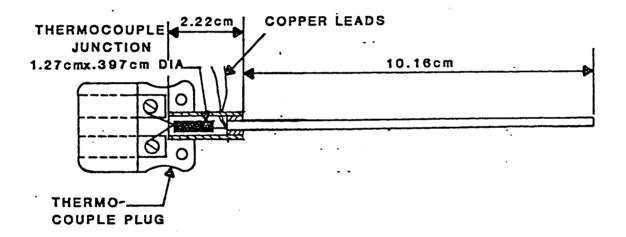
Fig. 3.2: Thermal Probe Construction Details.
