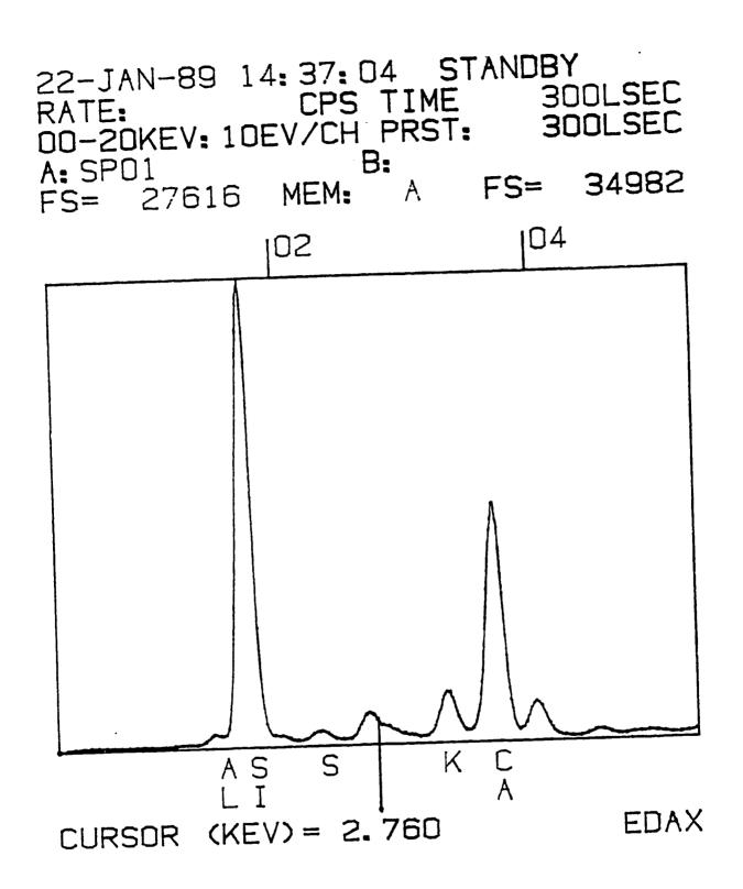
Fig. 8: X-Ray Fluorescence Analysis of Sample #1 (Dune Sand)
