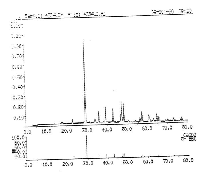
Fig. 7: X-Ray Diffraction of Limestone
