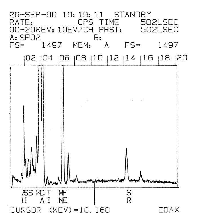
Fig.13: X-Ray Fluorescence Analysis of Sample #8 (Sandy Clay)
