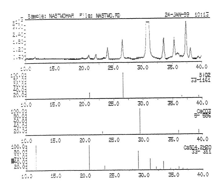
Fig. 4: X-Ray Diffraction Analysis of Sample #7 (Marl) (Continued)
