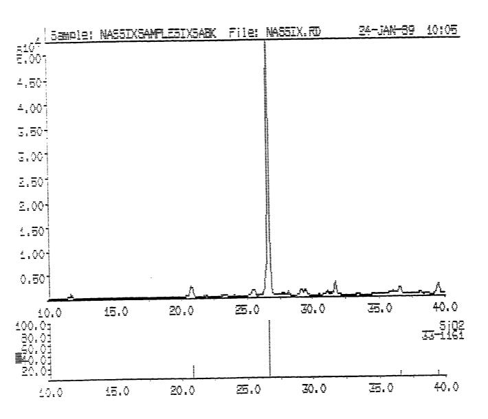
Fig. 3: X-Ray Diffraction Analysis of Sample #6 (Sahkha)
