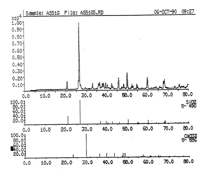
Fig. 2: X-Ray Diffraction Analysis of Sample #4 (Jubail Sand)
