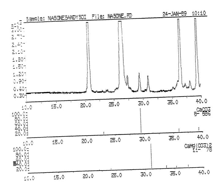
Fig. 1: X-Ray Diffraction Analysis of Sample #1 (Dune Sand) (Continued)
