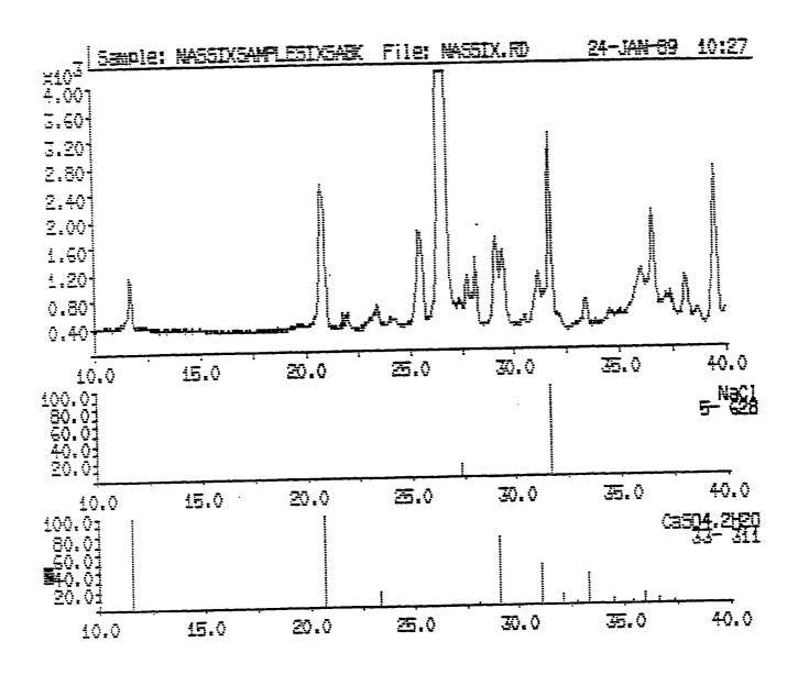
Fig. 3: X-Ray Diffraction Analysis of Sample #6 (Sabkha) (Continued)
