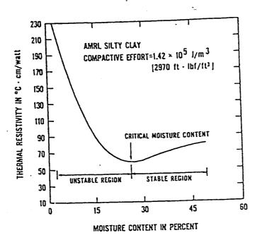
Fig. 2.5: Variation of Thermal Resistivity with Moisture Content Illustrating the Concept of Critical Moisture Content (Salomone, 1984).
