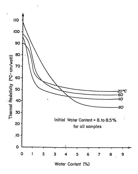
Fig. 2.4: Thermal Resistivity-Moisture Content Relationship for Sand at Four Different Temperatures (Brandon, 1985)
