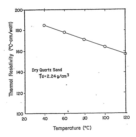
Fig. 2.3: Thermal Resistivity of a dry Quartz Sand as a Function of Temperature (Mitchell et al., 1977)
