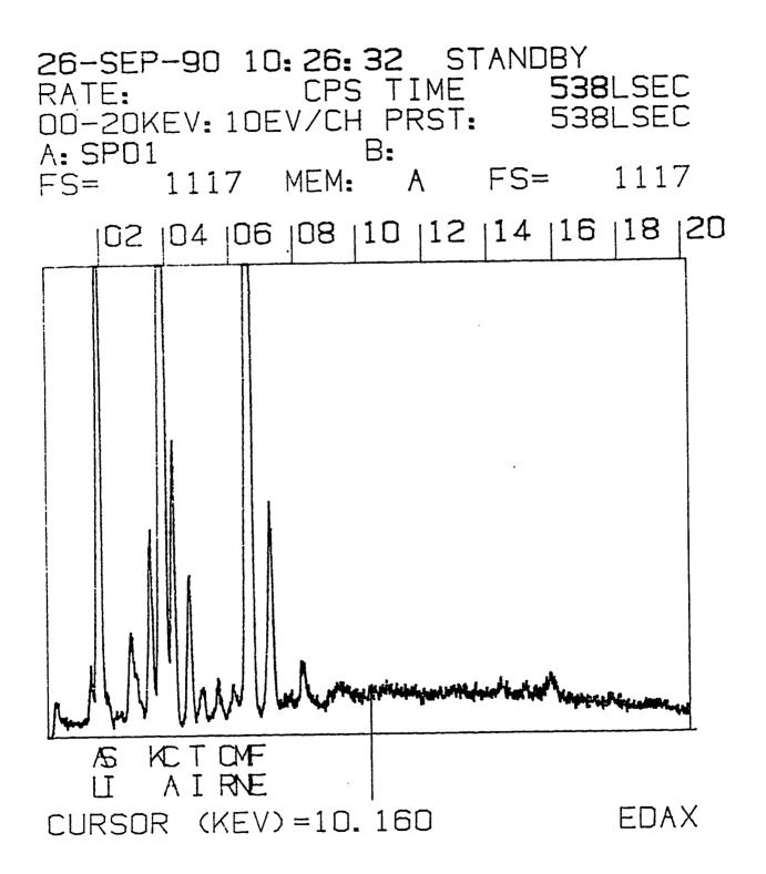
Fig.10: X-Ray Fluorescence Analysis of Sample #5 (Riyadh Sand)
