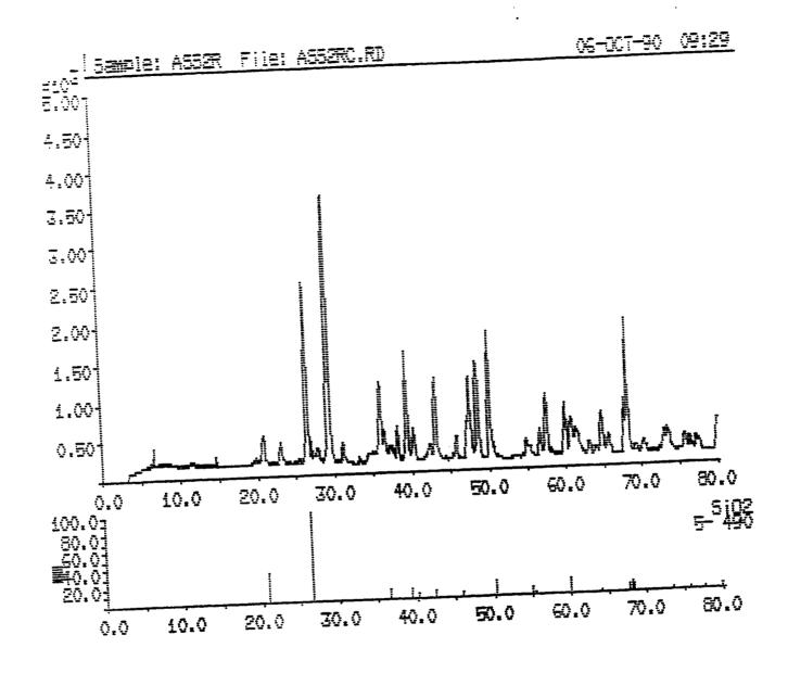
Fig. 5: X-Ray Diffraction Analysis of Sample #8 (Sandy Clay)
