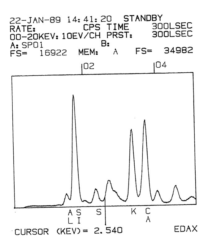
Fig.14: X-Ray Fluorescence Analysis of Sample #9 (Clay)
