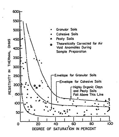
Fig. 2.1: Thermal Resistivity Data Showing the Effect of Soil Type and Moisture Content (Fisher, et al., 1975)
