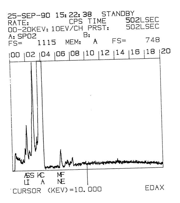
Fig.15: X-Ray Fluorescence Analysis of Limestone
