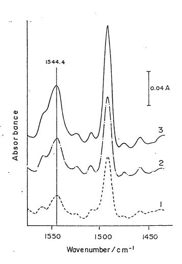
Figure 4.24 FTIR spectra of pyridine adsorbed on high-silica zeolite (H-form, Si/Al ratio 26), Steam treatment for 2 hrs,(1) at 500 °C, (2) at 350 °C, (3) untreated.
