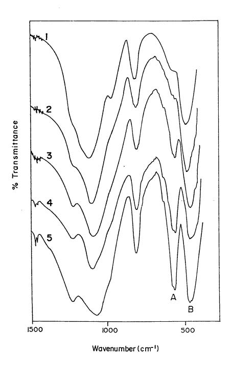
Figure 4.1 FTIR spectra of as-synthesized form of high-silica zeolites: (1) uncrystallized gel; (2) PB-1; (3) PB-5; (4) PB-8 and (5) PB-2 (Absorbance band A is at 550 cm<sup>-1</sup> and B at 450 cm<sup>-1</sup>).
