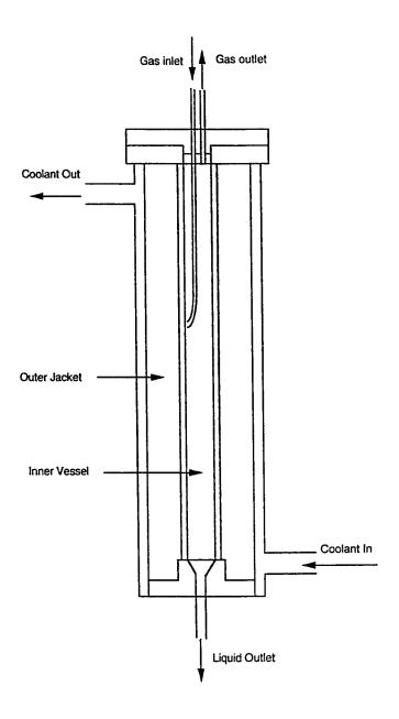
Figure 3.5 Gas Liquid Separator
