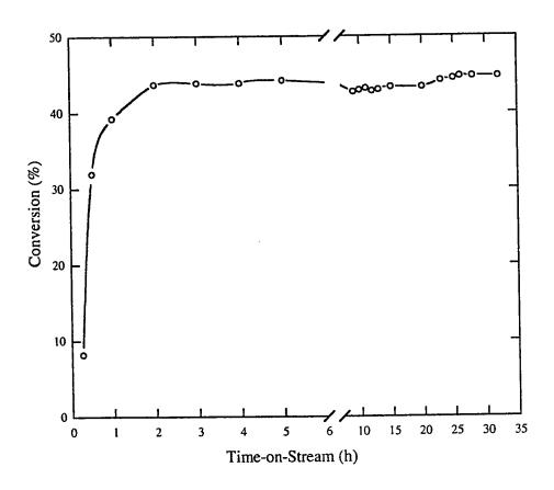
Figure 4.30 Conversion of isobutene vs. Time-on-Stream (catalyst, HSZ-25; temperature, 80  $^{\circ}$ C; m/i, 2.00; WHSV, 2.00 h<sup>-1</sup>).
