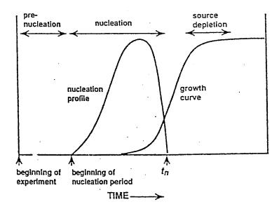
Figure 2.2 Schematic illustration of nucleation and growth curves for a hydrothermal zeolite synthesis [110].
