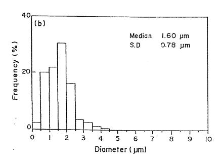
Figure 4.4 Particle size distribution of synthesized high-silica zeolites: (a) partially crystalline, (PB-11) and (b) crystalline, (PB-20).
