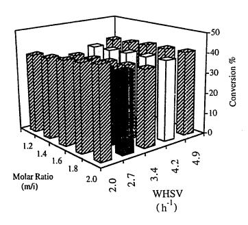
Figure 4.29 Effect of methanol to isobutene molar ratio and space velocity on conversion of isobutene (catalyst, HSZ-25; temp. 80 °C).
