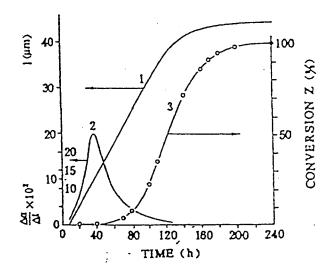
Figure 2.6 Nucleation kinetic curve (2) and the crystal mass growth curve (3) for Na-X zeolite calculated form data of Fig. 2.4 [43].
