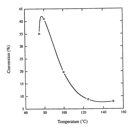
Figure 4.25 The effect of temperature on conversion of isobutene for HSZ-25, WHSV 4.87 h<sup>-1</sup>, m/i 1.70.
