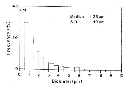
Figure 4.6 Particle size distribution of synthesized high-silica zeolites: (a) Rapid crystallization, time 2 h, (PB-20) and (b) Conventional crystallization, time 4 d, (HSZ-20N).
