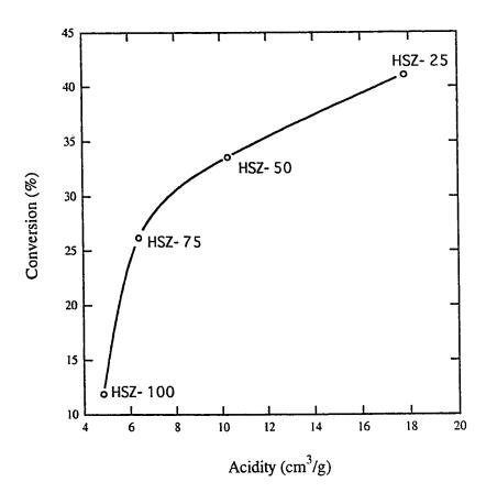
Figure 4.28 Total acidity measured by TPD of ammonia vs. conversion of isobutene (temperature  $80^{\circ}$  C, WHS  $4.87~h^{-1}$ , m/i 1.70).
