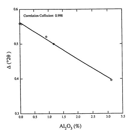
Figure 4.13 Correlation between peak spacing  $\Delta$  2 Theta (45.0°-45.5°) and Al<sub>2</sub>O<sub>3</sub> (Wt %) of H-form high-silica zeolites.
