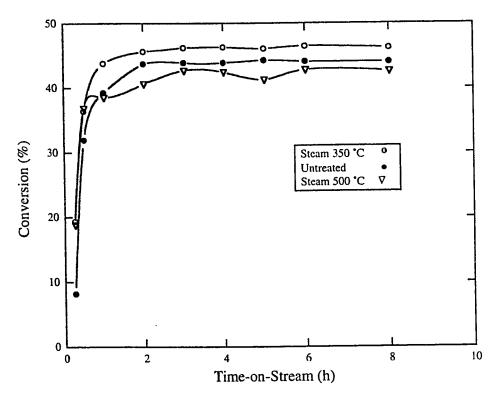
Figure 4.31 Effect of steaming on conversion of isobutene (catalyst HSZ-25, temp. 80 °C, WHSV 2.00 h<sup>-1</sup> and m/i 2.00).
