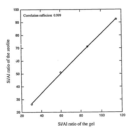
Figure 4.12 Chemical analysis data, plotted as Si/Al ratio of gel vs. Si/Al ratio of zeolite product.
