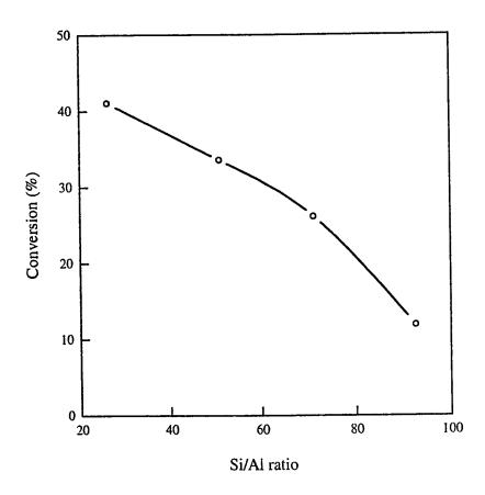
Figure 4.27 The effect of Si/Al ratio on the conversion of isobutene: WHSV 4.87 h-1, m/i 1.70, Temperature 80° C.
