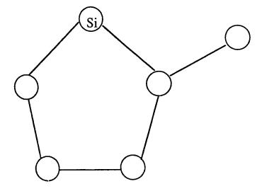
Figure 2.1 The secondary building unit of ZSM-5 zeolite.
