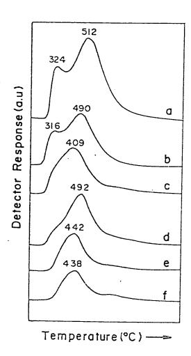
Figure 4.16 Temperature programmed desorption of ammonia for synthesized high-silica zeolites: (a) HSZ-25, (b) S-350, (c) S-500, (d) HSZ-50, (e) HSZ-75, (f) HSZ-100.
