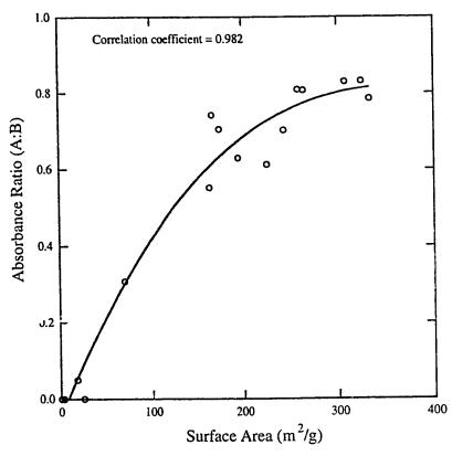
Figure 4.2 Correlation between BET Surface Area and Absorbance Ratio (I.R. Crystallinity) of synthesized High-Silica Zeolites.
