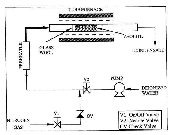
Figure 3.1 Flow diagram for steaming apparatus.
