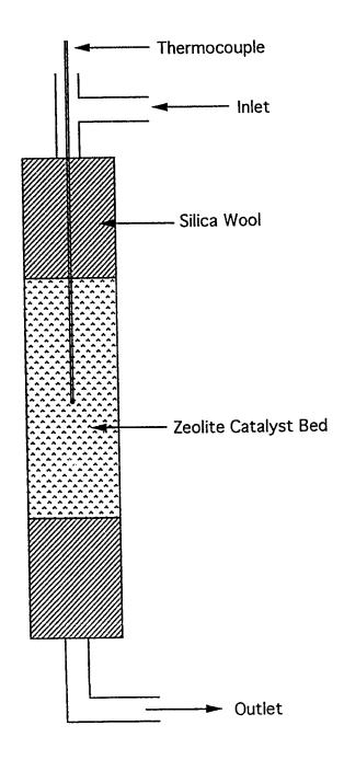
Figure 3.4 Schematic of Fixed Bed Tubular Reactor
