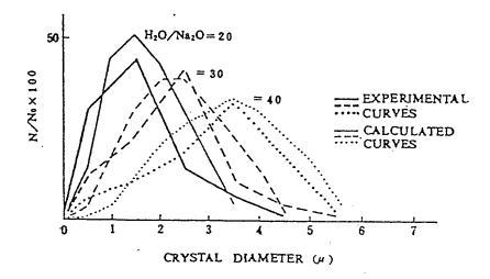
Figure 2.4 Influence of alkalinity on zeolite A crystallization (top) and on crystal size distribution (bottom), showing agreement between experimental and calculated values [107].
