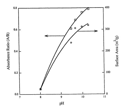
Figure 4.5 The effect of pH on IR crystallinity (Absorbance Ratio) and BET Surface Area.
