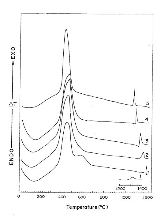
Figure 4.15 DTA curves for as-synthesized forms of high-silica zeolites: (1) HSZ-25, (2) HSZ-50, (3) HSZ-75, (4) HSZ-100 and (5) AF-HSZ.
