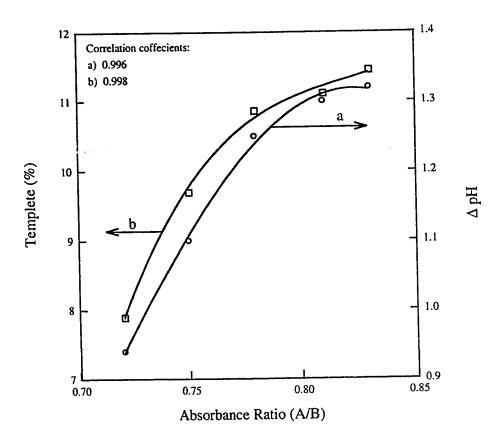
Figure 4.10 Correlation between IR crystallinity (Absorbance Ratio), Template (%) and difference of pH.
