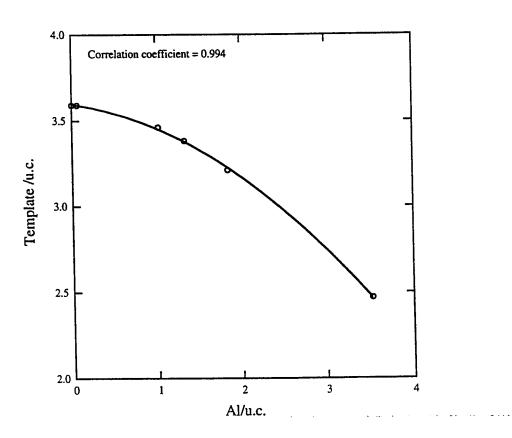
Figure 4.9 Correlation between Al content per unit cell and template content (TPA<sup>+</sup>) per unit cell.
