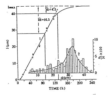
Figure 2.5 Crystal size growth of Na-X zeolite during crystallization of the gel (1) and the histogram of crystal size distribution in the final product (2) [43].
