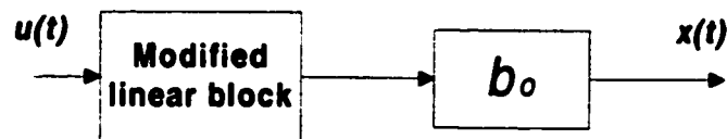
Figure 4.14: Modified linear block in the Wiener model with b_o factored out.
