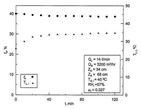
Figure 5.44:Time variation of concentration and inlet temperature for 40% LiCl solution in the dehumidifier while the hybrid system is running.
