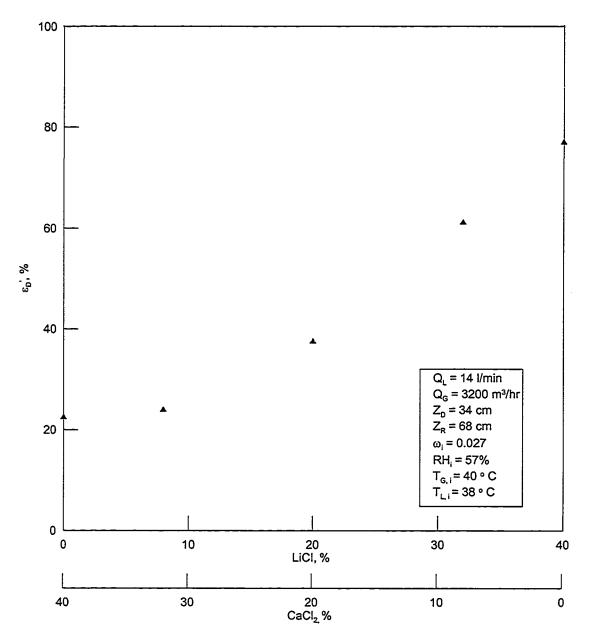
Figure 5.69: The effect of desiccant mixture composition on the average dehumidier effectiveness while the hybrid system is running.
