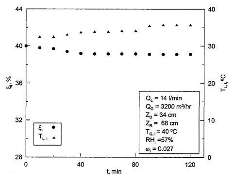
Figure 5.62:Time variation of concentration and inlet temperature for 8% CaCl<sub>2</sub> and 32% LiCl solution in the dehumidifier while the hybrid system is running.
