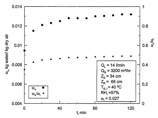
Figure 5.46: Time variation of outlet absolute humidity and ratio of outlet to inlet absolute humidity for 40% LiCl solution in the dehumidifier while the hybrid system is running.
