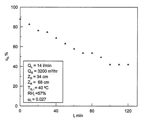
Figure 5.65: Effectiveness of the dehumidifier with time for 8% CaCl<sub>2</sub> and 32% LiCl solution while the hybrid system is running.
