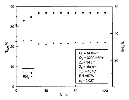
Figure 5.45:Time variation of outlet air temperature and humidity in the dehumidifier for 40% LiCl solution while the hybrid systemis running.
