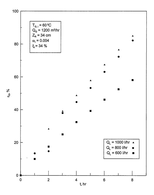
Figure 5.23: Effectiveness of the regenerator with time for  $T_{\rm G,\,i}$  = 60  $^{\rm o}$ C for different desiccant flow rates.
