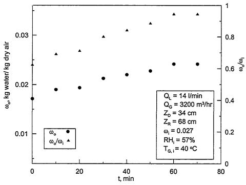
Figure 5.32: Time variation of outlet absolute humidity and ratio of outlet to inlet absolute humidity for 34 cm packing height in the dehumidifier and 68 cm in the regenerator while the hybrid system is running
