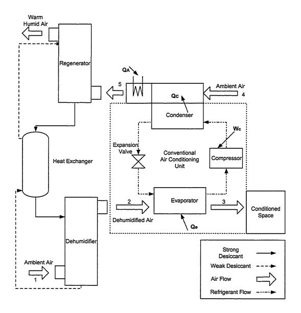
Figure 1.2: Schematic of the hybrid cooling system
