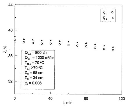
Figure 5.54: Time variation of inlet and outlet concentration for 32%  ${\rm CaCl_2}$  and 8% LiClsolution in the regenerator while the hybrid system is running.
