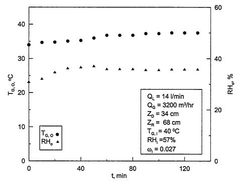
Figure 5.57:Time variation of outlet air temperature and humidity in the dehumidifier for 20% CaCl<sub>2</sub> and 20% LiCl solution while the hybrid system is running.
