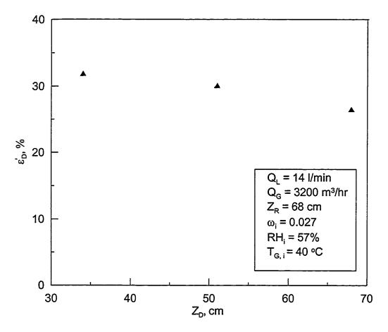
Figure 5.42: Average effectiveness of the dehumidifier with packing height while the hybrid system is running.
