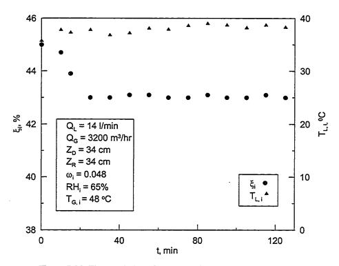
Figure 5.36: Time variation of concentration and desiccant temperature in the dehumidifier for humid condition in both towers while the hybrid system is running
