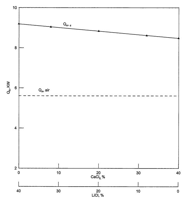
Figure 6.2: The amount of auxillary energy needed for regenerating the desiccant mixtures.
