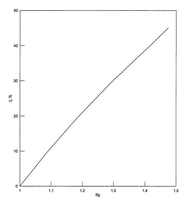
Figure 3.1: Calcium chloride desiccant calibration curve.
