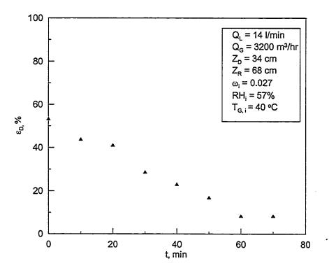
Figure 5.33: Effectiveness of dehumidifier with time for 34 cm packing height in the dehumidifier and 68 cm in the regenerator while the hybrid system is running
