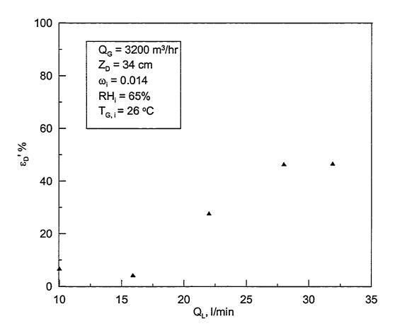
Figure 5.7: Average effectiveness of the dehumidifier with time for various flow rates.
