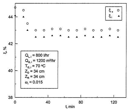
Figure 5.40: Time variation of inlet and outlet concentration in the regenerator for humid condition while the hybrid system is running.
