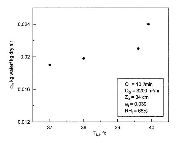
Figure 5.8: Effect of desiccant inlet temperature on the change in air absolute humidity in the dehumidifier.
