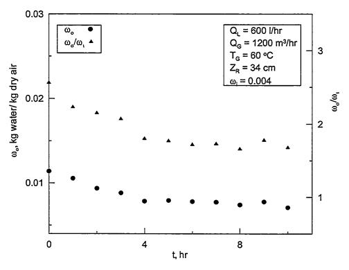
Figure 5.13: Time variation of outlet absolute humidity and ratio of outlet to inlet absolute humidity for  $Q_L$  = 600 l/hr and  $T_{G,\,i}$  = 60 °C in the regenerator.
