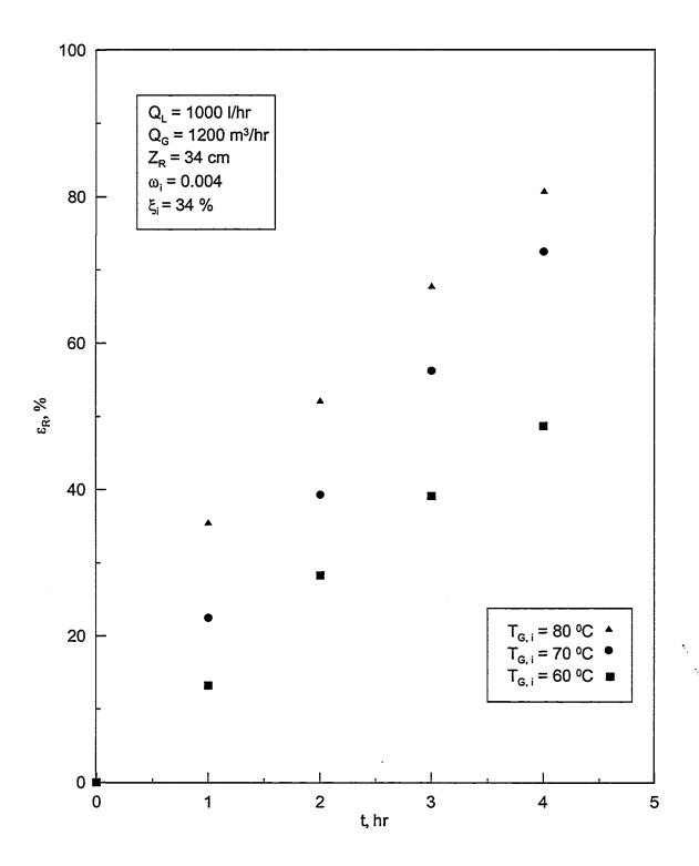
Figure 5.22: Effectiveness of the regenerator with time for  $Q_L$  = 1000 l/hr for different air temperatures.
