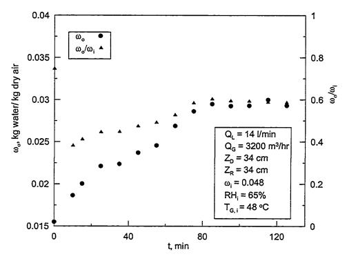
Figure 5.38: Time variation of outlet absolute humidity and ratio of outlet to inlet absolute humidity in the dehumidifier for 34 cm packing height in both towers while the hybrid system is running
