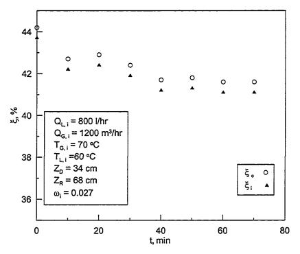
Figure 5.34: Time variation of inlet and outlet concentration for 68 cm packing height in the regenerator and 34 cm in the dehumidifier while the hybrid system is running.
