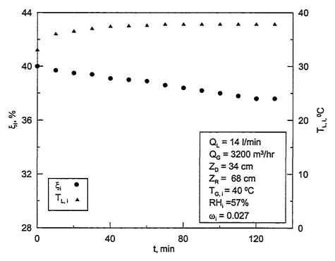
Figure 5.56:Time variation of concentration and inlet temperature for 20% CaCl<sub>2</sub> and 20% LiCl solution in the dehumidifier while the hybrid system is running.
