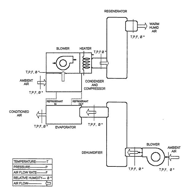
Figure 4.6: Schematic of the air loop for regeneration system
