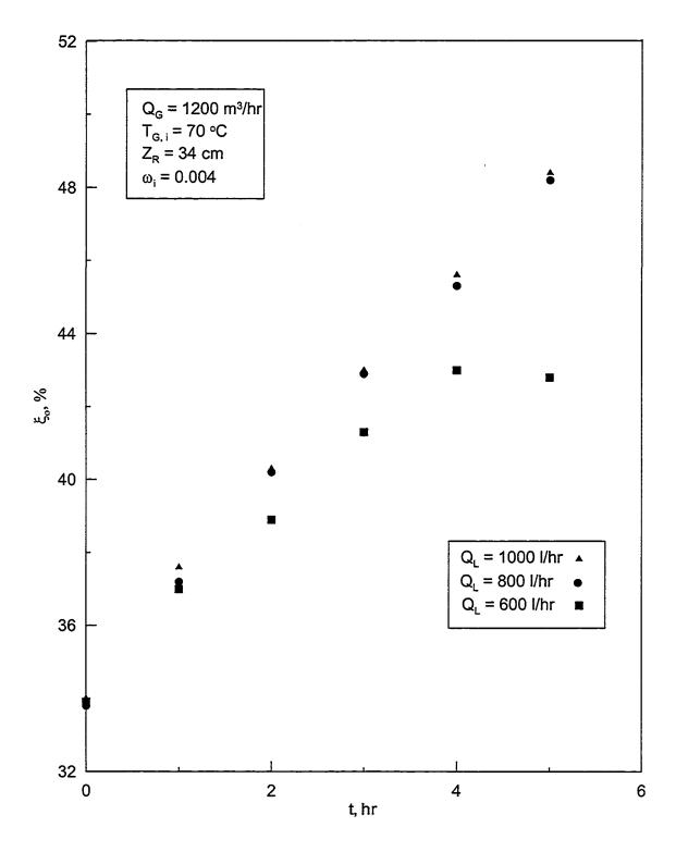
Figure 5.15: Variation of concentration with time for different desiccant flow rates at 70°C air inlet temperature in the regenerator.
