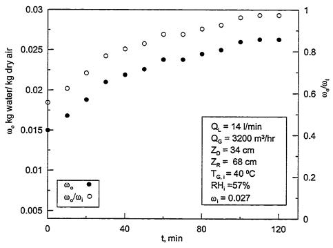
Figure 5.53: Time variation of outlet absolute humidity and ratio of outlet to inlet absolute humidity for 32% CaCl<sub>2</sub> and 8% LiCl solution in the dehumidifier while the hybrid system is running.
