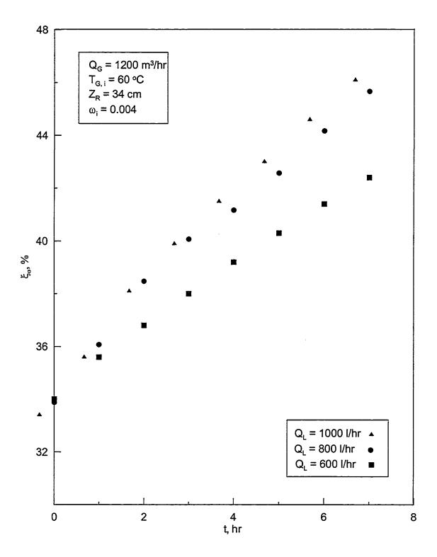
Figure 5.14: Variation of concentration with time for different desiccant flow rates at 60°C air inlet temperature in the regenerator.
