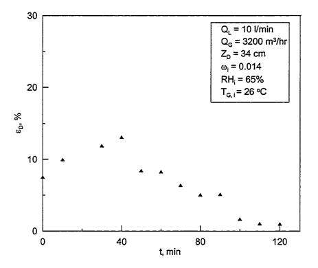
Figure 5.5: Effectiveness of the dehumidifier with time for  $Q_{\rm L}$ = 10l/min.
