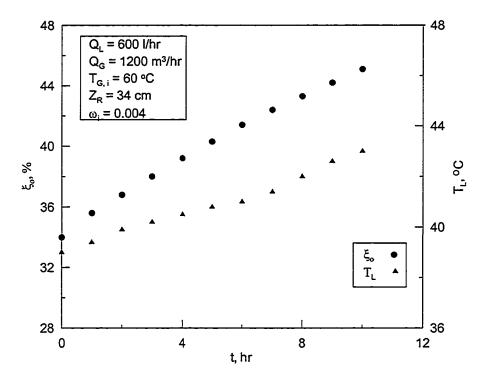
Figure 5.10: Time variation of concentration and desiccant temperature for  $\rm Q_L$  = 600 l/hr and  $\rm T_{G,i}$  = 60  $^{o}C$  in the regenerator.
