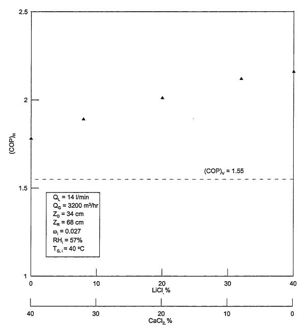
Figure 6.1: The effect of desiccant mixture composition on the coefficient of performance.
