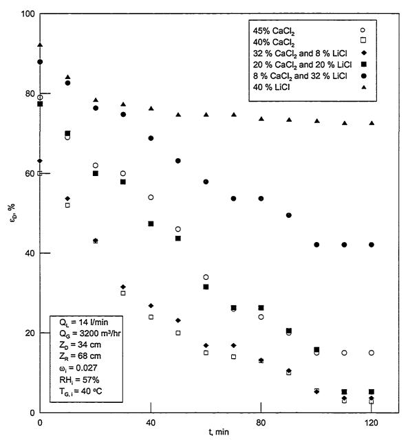
Figure 5.68: The effectiveness of the dehumidifier with time while the hybrid system is running.
