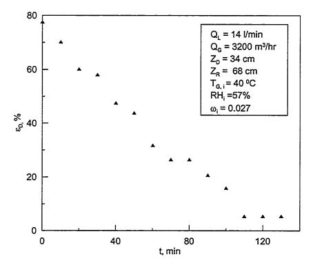
Figure 5.59: Effectiveness of the dehumidifier with time for 20%  ${\rm CaCl_2}$  and 20% LiCl solution while the hybrid system is running.
