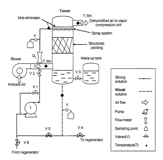
Fig 4.1: Schematic diagram of the experimental apparatus for air dehumidification.
