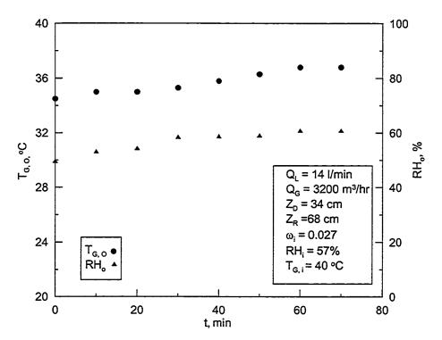
Figure 5.31: Time variation of outlet air temperature and humidity for 34 cm packing height in the dehumidifier and 68 cm in the regenerator while the hybrid system is running.
