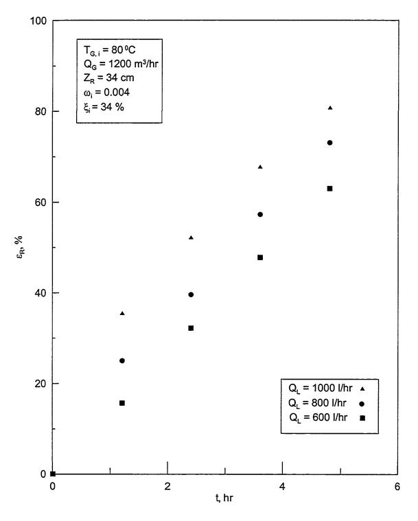
Figure 5.25: Effectiveness of the regenerator with time for  $T_{G,\,i}$  = 80 °C for different desiccant flow rates.
