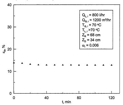
Figure 5.67: Effectiveness of the regenerator with time for 8% CaCl<sub>2</sub> chloride and 32% LiCl solution while the hybrid system is running.
