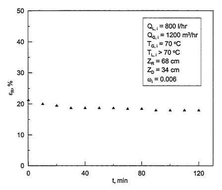
Figure 5.49: Effectiveness of the regenerator with time for 40% LiCl solution while the hybrid system is running.
