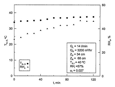
Figure 5.63:Time variation of outlet air temperature and humidity in the dehumidifier for 8% CaCl<sub>2</sub> and 32% LiCl solution while the hybrid system is running.
