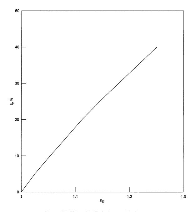
Figure 3.2: Lithium chloride desiccant calibration curve.
