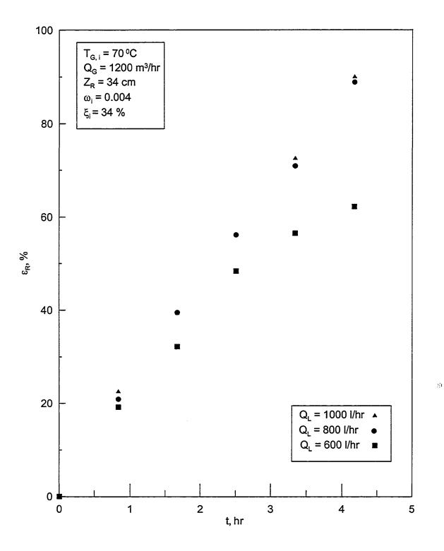
Figure 5.24: Effectiveness of the regenerator with time for  $T_{G,\,i}$  = 70 °C for different desiccant flow rates.
