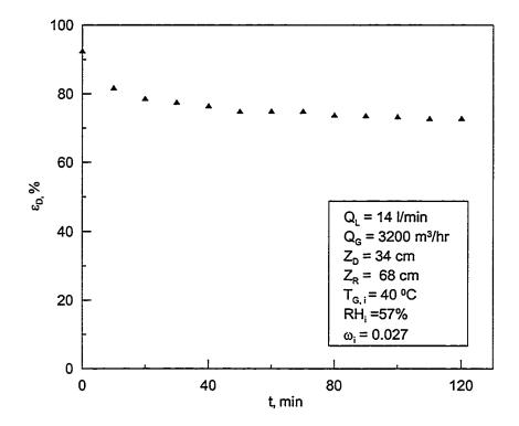
Figure 5.47: Effectiveness of the dehumidifier with time for 40% LiCl solution while the hybrid system is running.
