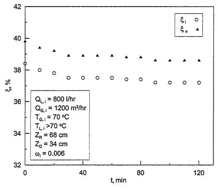
Figure 5.48: Time variation of inlet and outlet concentration for 40% LiCl solution in the regenerator while the hybrid system is running.
