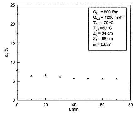
Figure 5.35: Effectiveness of regenerator with time for 68 cm packing height in the regenerator and 34 cm in the dehumidifier while the hybrid system is running.
