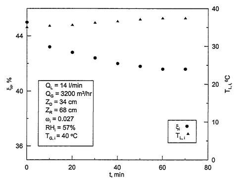
Figure 5.30: Time variation of concentration and desiccant temperature for 34 cm packing height in the dehumidifier and 68 cm in the regenerator while the hybrid system is running.
