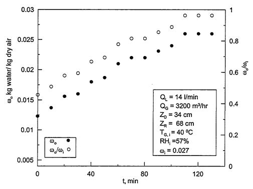
Figure 5.58: Time variation of outlet absolute humidity and ratio of outlet to inlet absolute humidity for 20% CaCl<sub>2</sub> and 20% LiCl solution in the dehumidifier while the hybrid system is running.
