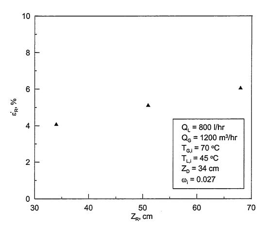
Figure 5.43: Average effectiveness of the regenerator with packing height while the hybrid system is running.
