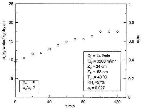
Figure 5.64: Time variation of outlet absolute humidity and ratio of outlet to inlet absolute humidity for 8% CaCl<sub>2</sub> and 32% LiCl solution in the dehumidifier while the hybrid system is running.
