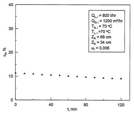
Figure 5.61: Effectiveness of the regenerator with time for 20% CaCl<sub>2</sub> chloride and 20% LiCl solution while the hybrid system is running.
