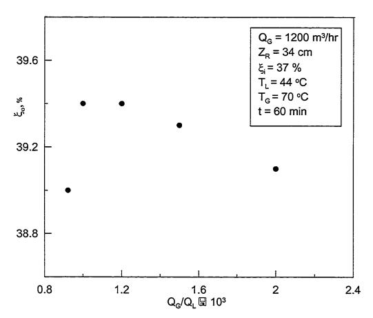
Figure 5.26: Effect of the ratio of air to desiccant flow rate on the outlet concentration in the regenerator.
