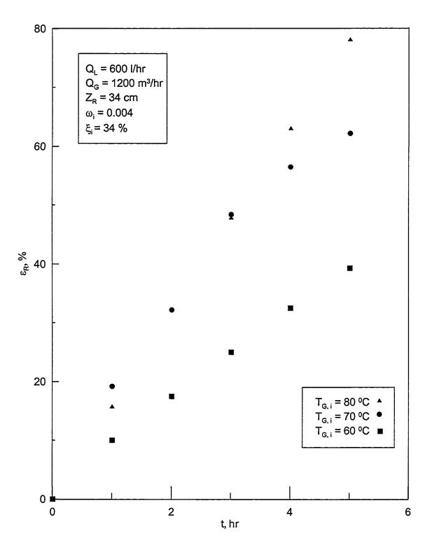
Figure 5.20: Effectiveness of the regenerator with time for  $Q_L$  = 600 l/hr for different air temperatures.
