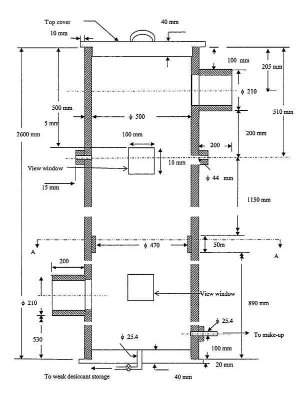
Fig. 4.2 Detailed dimensions of the dehumidfiier
