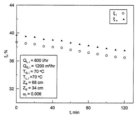
Figure 5.60: Time variation of inlet and outlet concentration for 20% CaCl<sub>2</sub> and 20%LiCl solution in the regenerator while the hybrid system is running.
