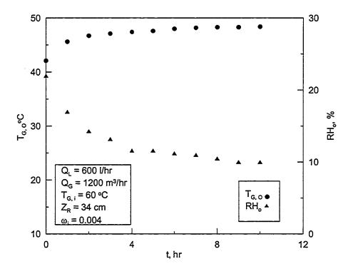
Figure 5.11: Time variation of outlet temperature and humidity for Q<sub>L</sub>= 600 l/hr and T<sub>G, i</sub>= 60  $^{\circ}$ C in the regenerator.
