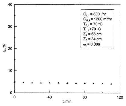
Figure 5.55: Effectiveness of the regenerator with time for 32% CaCl<sub>2</sub> and 8% LiCl chloride solution while the hybrid system is running.
