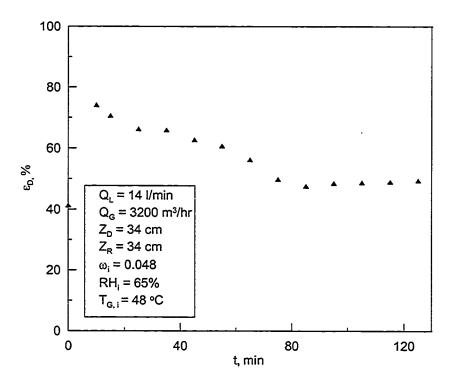
Figure 5.39: Effectiveness of dehumidifier with time for 34 cm packing height in both towers while the hybrid system is running
