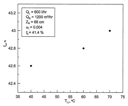
Figure 5.27: Effect of desiccant inlet temperature on the outlet concentration in the regenerator.
