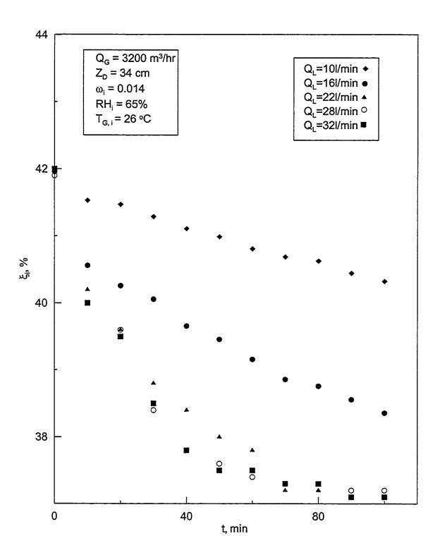
Figure 5.6: Variation of concentration with time for different desiccant flow rates in the dehumidifier.
