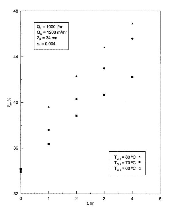
Figure 5.19: Variation of concentration with time for different air inlet temperatures at 1000l/hr desiccant flowrate in the regenerator.
