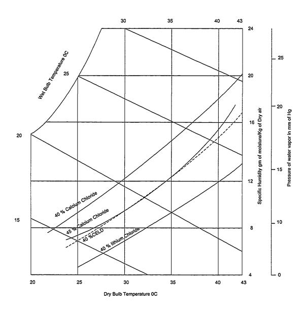
Figure 3.3: Calcium chloride, lithium chloride and CELD equilibrium curves plotted on a psychrometric chart
