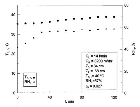
Figure 5.51:Time variation of outlet air temperature and humidity in the dehumidifier for 32% CaCl<sub>2</sub> and 8% LiCl solution while the hybrid system is running.
