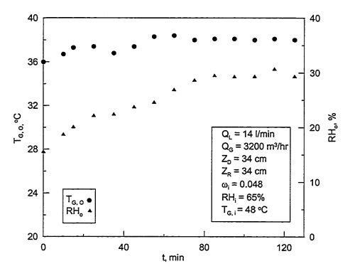
Figure 5.37: Time variation of outlet air temperature and humidity in the dehumidifier for humid condition while the hybrid system is running.
