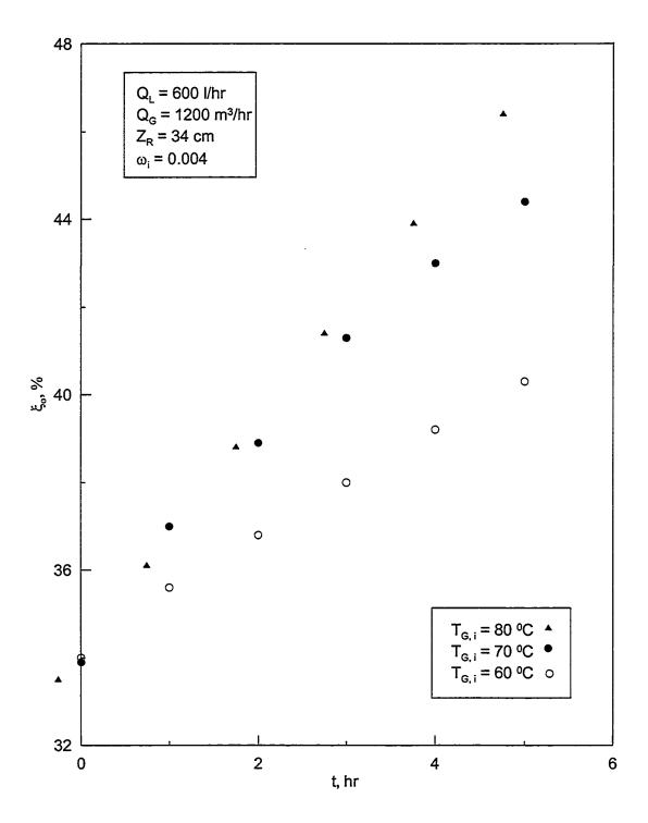
Figure 5.17: Variation of concentration with time for different air inlet temperatures at 600l/hr desiccant flowrate in the regenerator.
