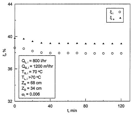
Figure 5.66: Time variation of inlet and outlet concentration for 8% CaCl<sub>2</sub> and 32% LiCl solution in the regenerator while the hybrid system is running.
