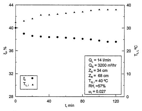
Figure 5.50:Time variation of concentration and inlet temperature for 32% CaCl<sub>2</sub> and 8% LiCl solution in the dehumidifier while the hybrid system is running.
