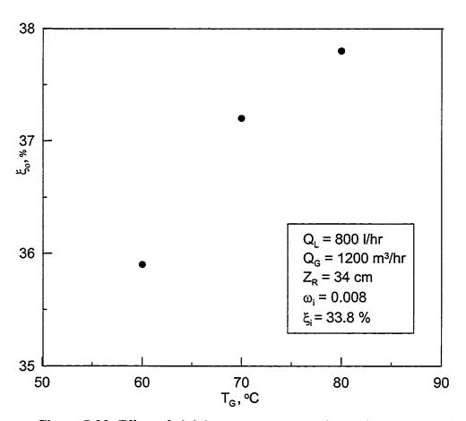
Figure 5.28: Effect of air inlet temperature on the outlet concentration in the regenerator.
