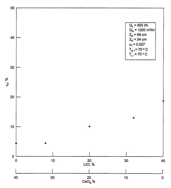
Figure 5.70: The effect of desiccant mixture composition on the average regenerator effectiveness while the hybrid system is running.
