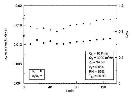
Figure 5.4: Time variation of outlet absolute humidty and ratio of outlet to inlet absolute humidty for  $Q_L$  = 10 l/min in the dehumidifier.
