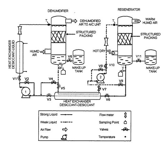
Fig.4.12: Schematic of the desiccant loop in the hybrid cooling system.
