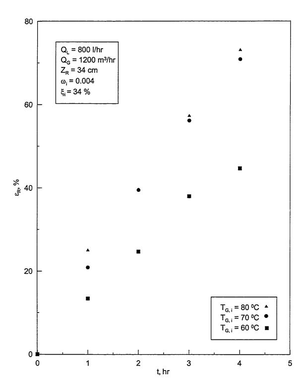
Figure 5.21: Effectiveness of the regenerator with time for  $Q_L$  = 800 l/hr for different air temperatures.
