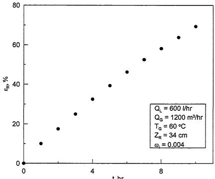
t, hr Figure 5.12: Effectiveness of the regenerator with time for  $\rm Q_L$  = 600 l/hr and  $\rm T_{G,\,i}$  = 60  $^{\rm 0}C$  in the regenerator.
