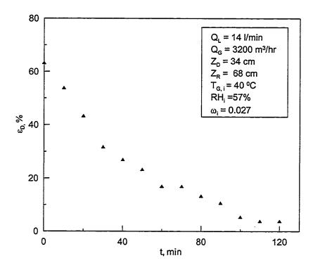
Figure 5.52: Effectiveness of the dehumidifier with time for 32% CaCl<sub>2</sub> and 8% LiCl solution while the hybrid system is running.
