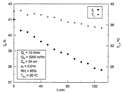
Figure 5.2: Time variation of concentration and desiccant temperature for  $\mathbf{Q}_{\mathbf{L}}$  = 10 l/min in the dehumidifier.
