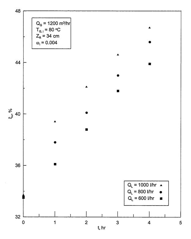
Figure 5.16: Variation of concentration with time for different desiccant flow rates at  $80^{\circ}$ C air inlet temperature in the regenerator.
