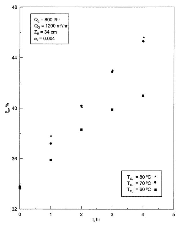
Figure 5.18: Variation of concentration with time for different air inlet temperatures at 800l/hr desiccant flowrate in the regenerator.
