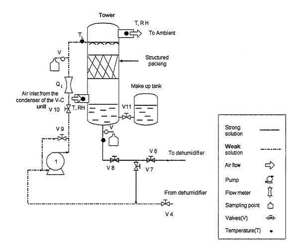
Figure 4.5: Schematic of the experimental apparatus for desiccant regeneration.
