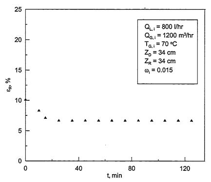
Figure 5.41: Effectiveness of regenerator with time humid condition in both towers while the hybrid system is running
