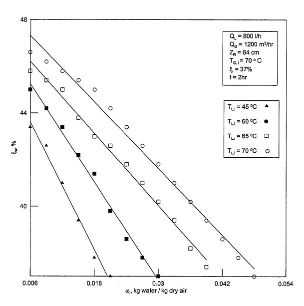
Figure 5.29: The effect of air inlet humidity ratio on the outlet desiccant concentration in the regenerator for various desiccant inlet temperature.
