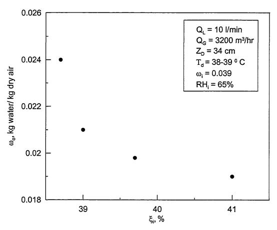
Figure 5.9: Effect of desiccant concentration on the dehumidifier performance in the dehumidifier.
