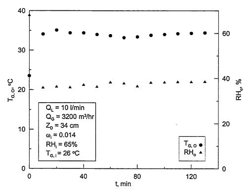
Figure 5.3: Time variation of outlet temperature and humidity for  $\mathbf{Q}_{L}$ = 10 l/min in the dehumidifier.
