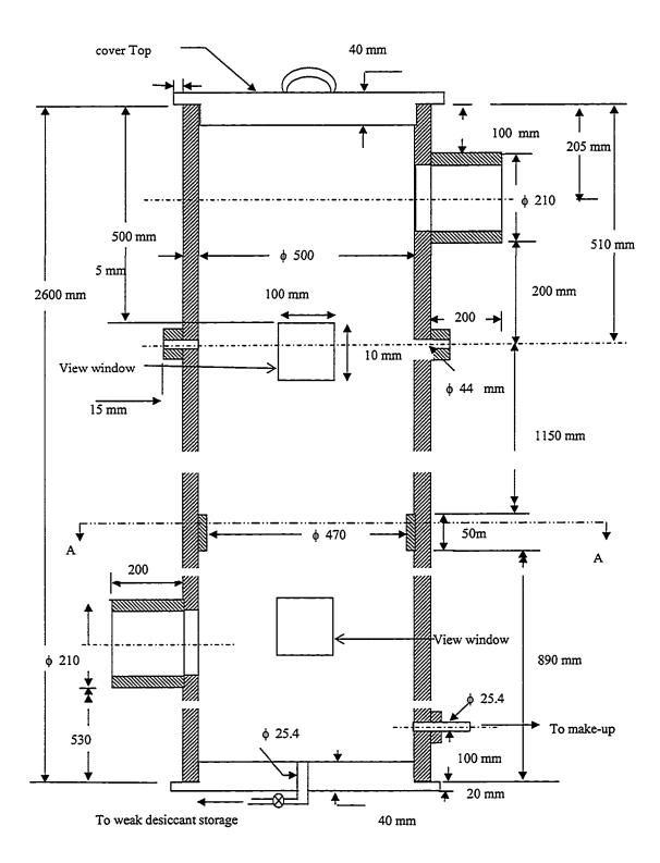
Fig. 4.7 Detailed dimensions of the regenerator
