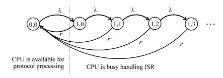
Figure 2. Markov state transition diagram for modeling CPU usage with DMA
