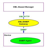
Fig. 1. An XML-based Network Management Architecture
