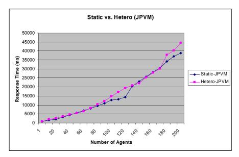
Fig. 6. Response Time for Heterogeneous Systems vs. Static Weighted Load Balancing
