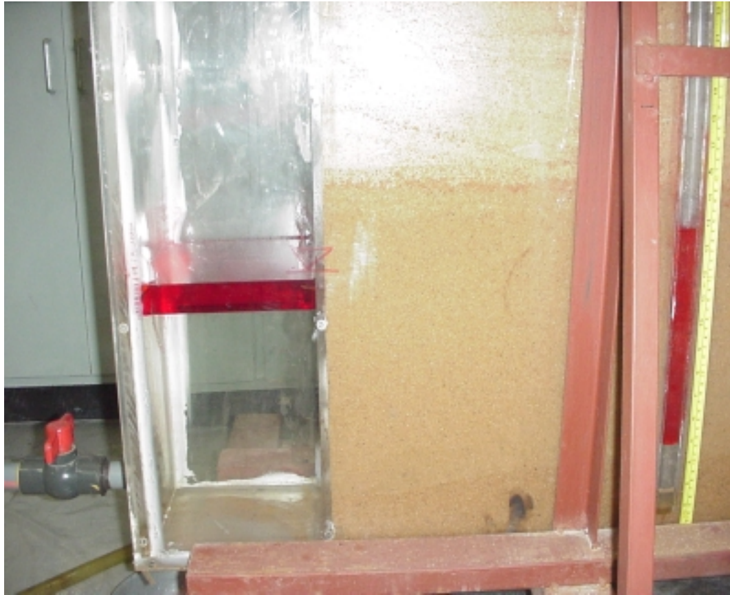
Plate 4.7 Accidental entrance of LNAPL into the water sump during preliminary run.
