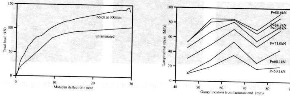
Figure 10. Load line deflection and strain gauge history for shear notched delamination specimen
