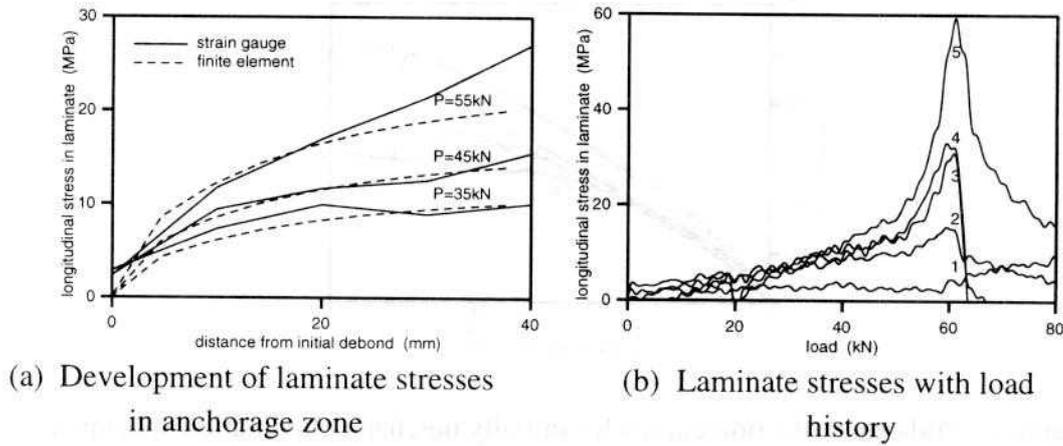
Figure 6. Results from the strain gauges on the beam with 1.4m bonded length
