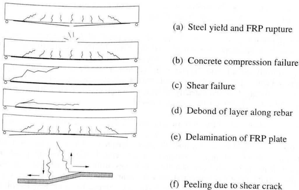
Figure 1. Failure modes in FRP retrofitted concrete beams
