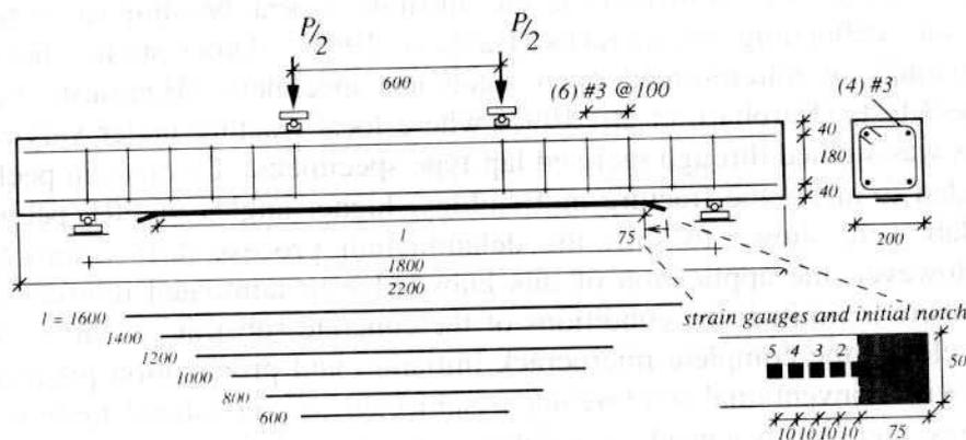
Figure 4. Specialized delamination test specimen
