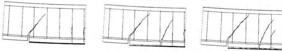
Figure 3. High speed video clips of plate end zone failures, after (Holzenkampfer, 1995)
