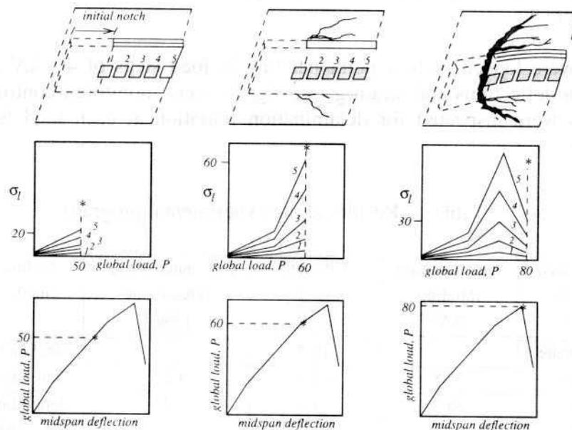
Figure 7. Delamination process zone development with idealizations of Figures 6(b) and 5 for the 1.4 m laminate length beam
