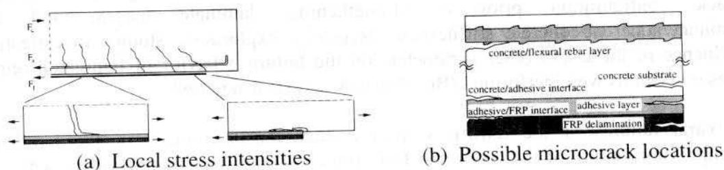
Figure 2. Local stress intensities and microcrack initiation scenarios
