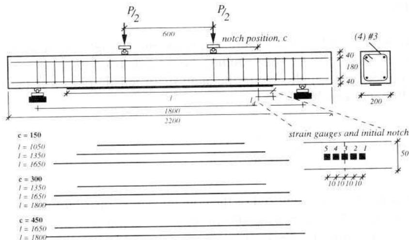
Figure 9. Delamination specimen with initial shear notches
