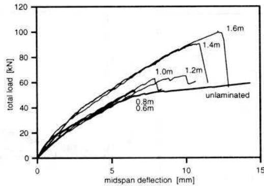
Figure 5. Midspan deflection curves for initially notched delamination specimen
