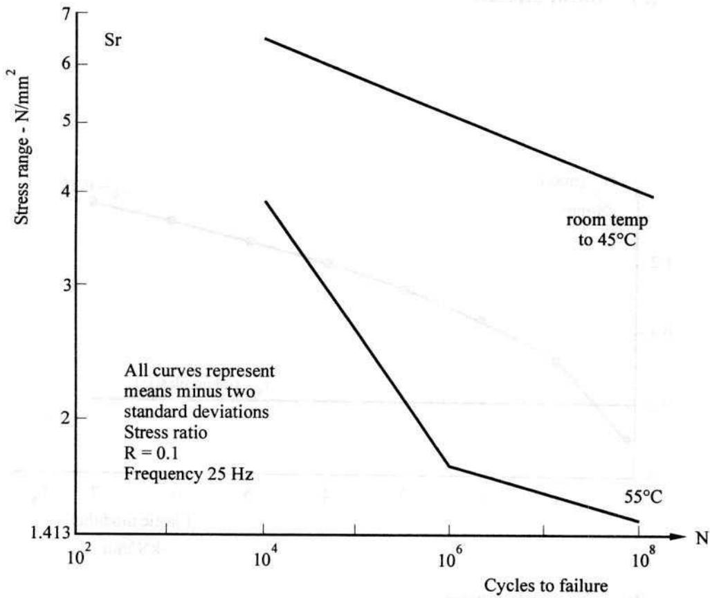
**Figure 4** Typical fatigue curves for bonded lap joints
