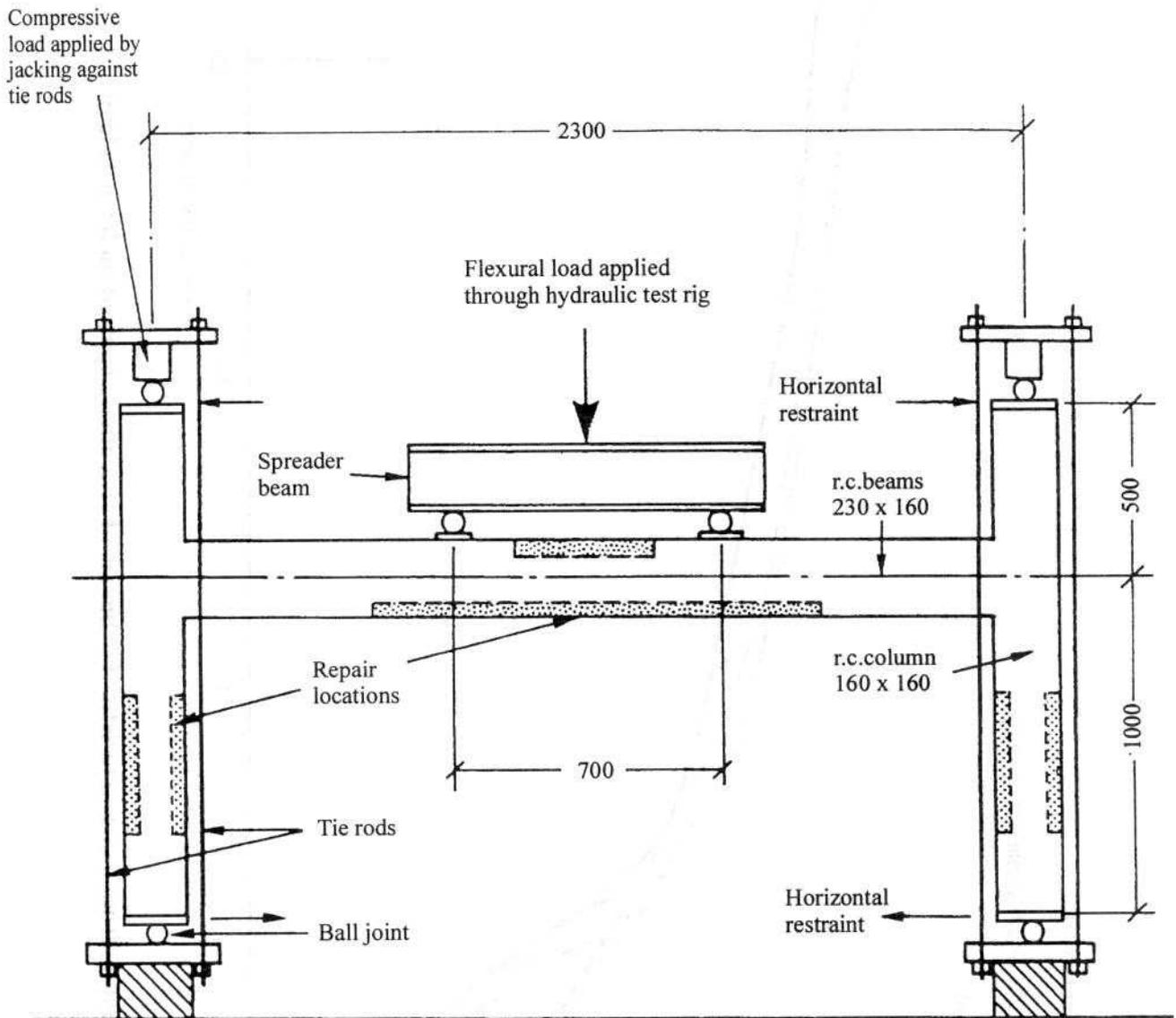
Figure 9 Schematic test arrangement for H-frames
