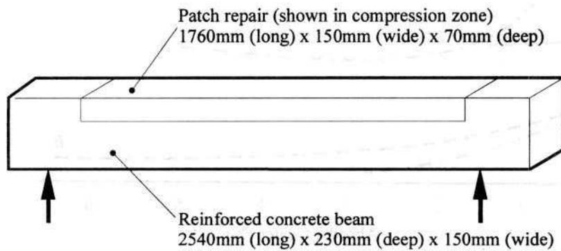
**Figure 8 Patch repair in beam element**
