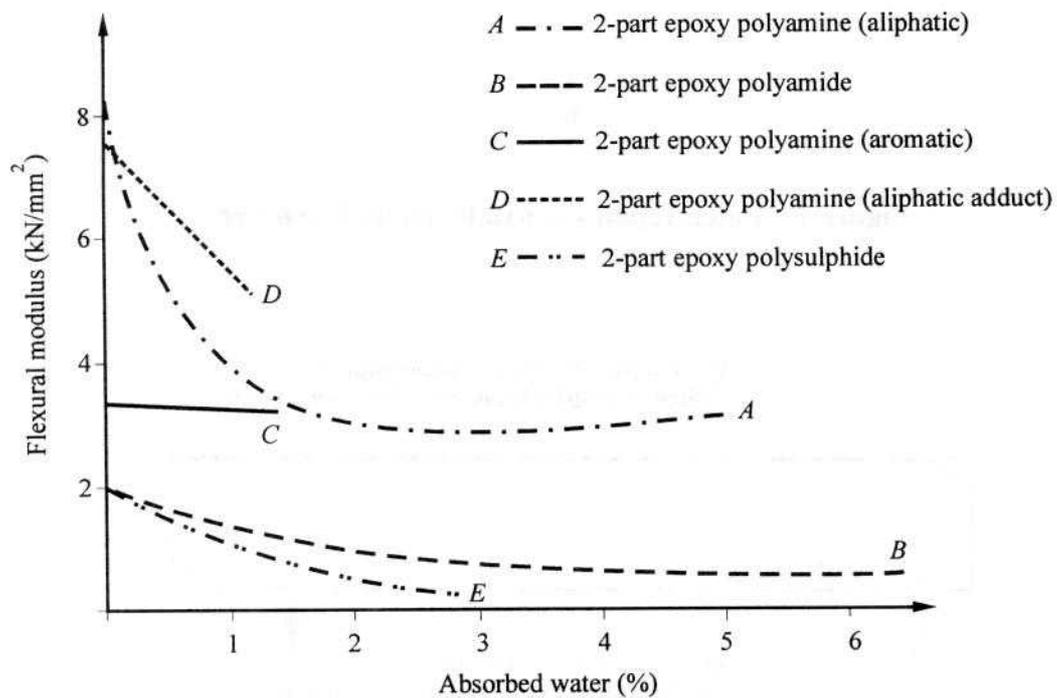
**Figure 6** Moisture dependence of bulk adhesive flexural modulus
