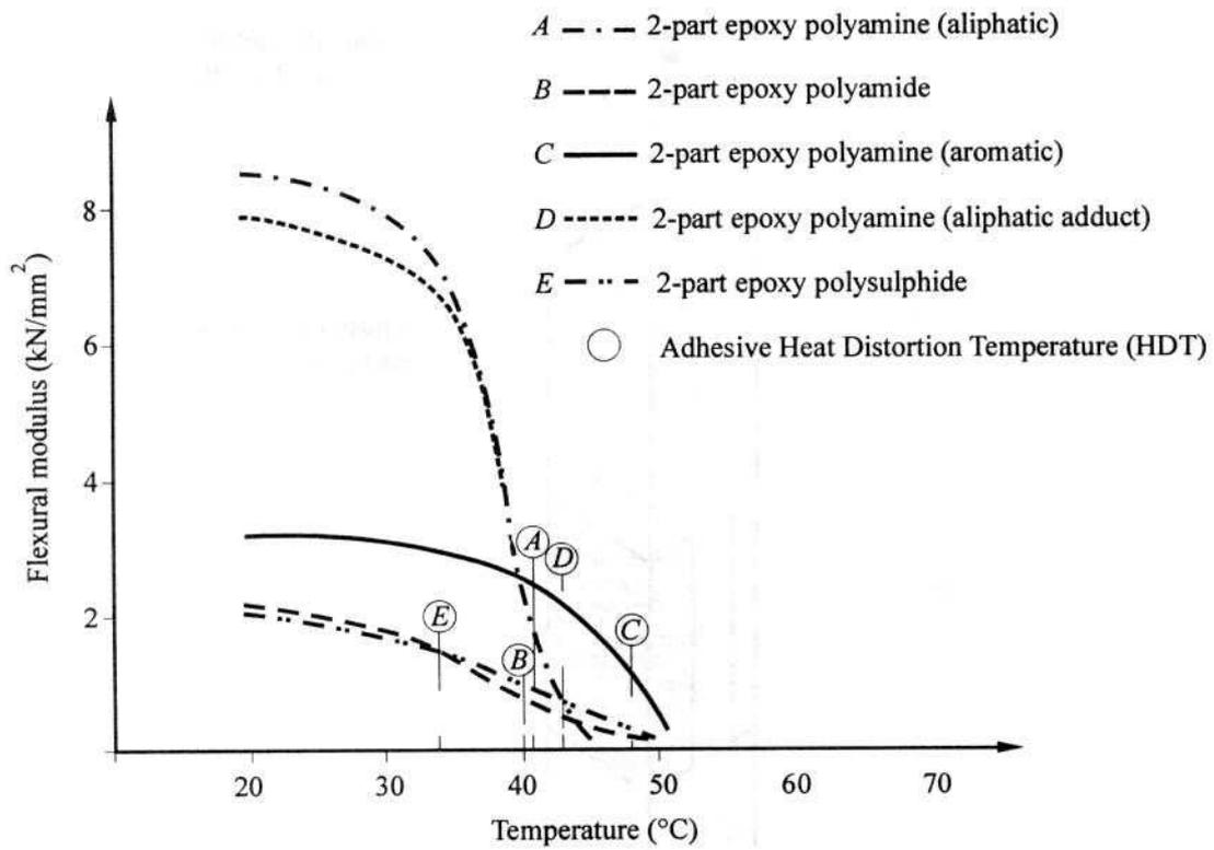
**Figure 5** Temperature dependence of bulk adhesive flexural modulus
