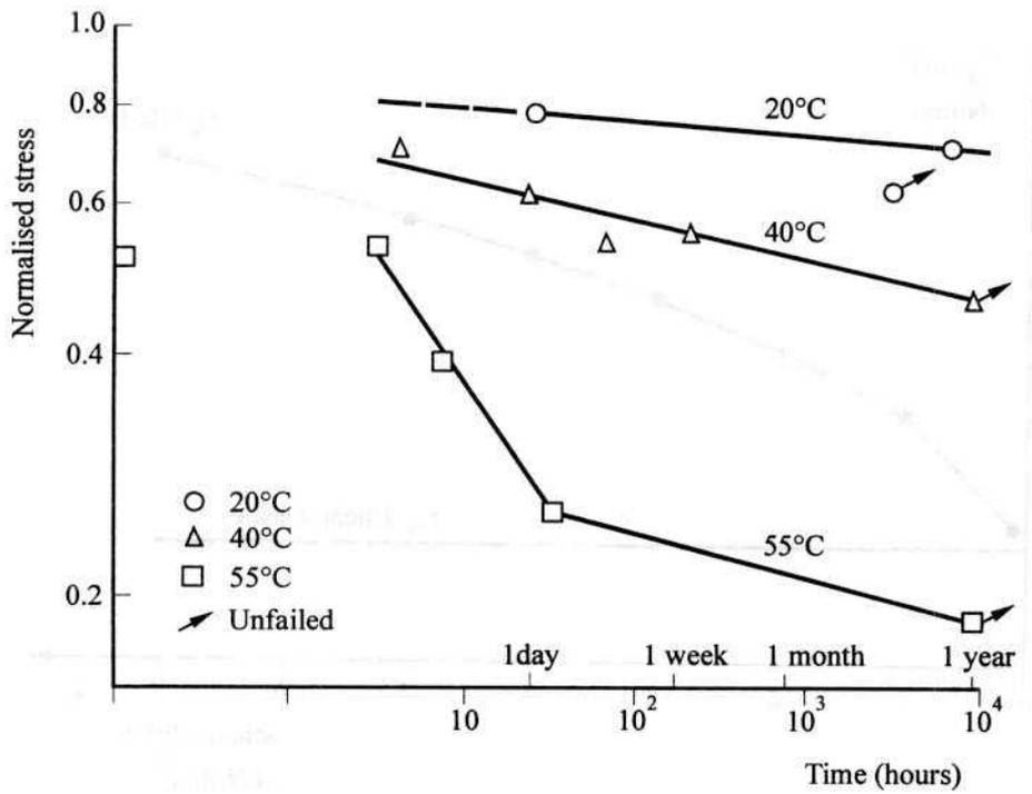
**Figure 3** Typical creep curves for bonded lap joints
