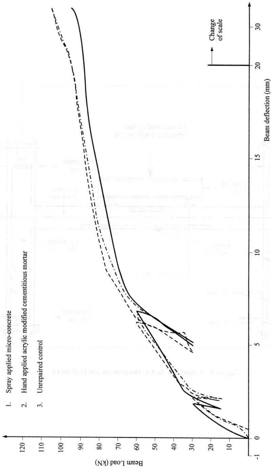
Figure 10 Load deflection characteristics for beams of H-frames repaired under zero load
