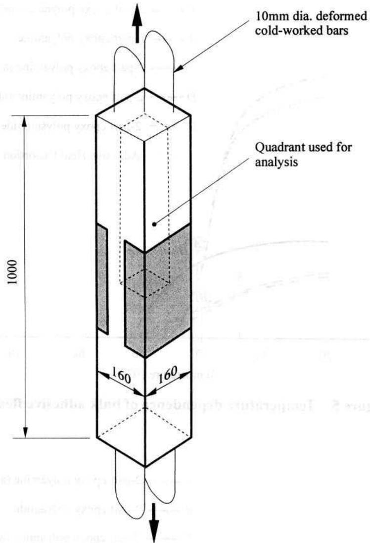
**Figure 7 Patch repairs in axially loaded member**
