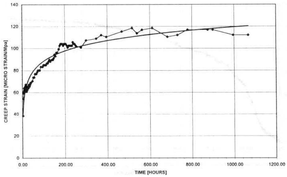
Fig. 4. Specific tensile creep  $\epsilon_{cr}$  vs.  $t$  for material FRM
