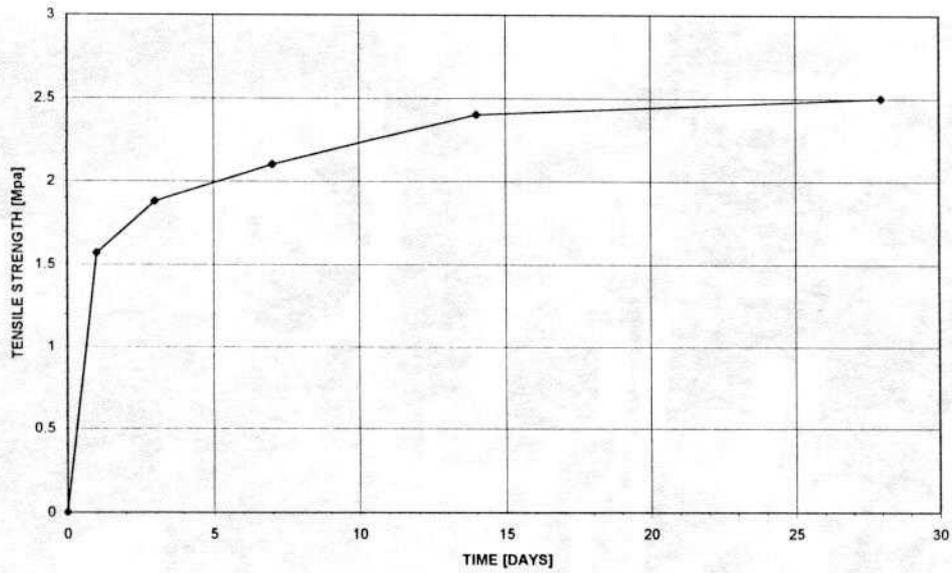
Fig. 5. Evolution of tensile strength for PMC
