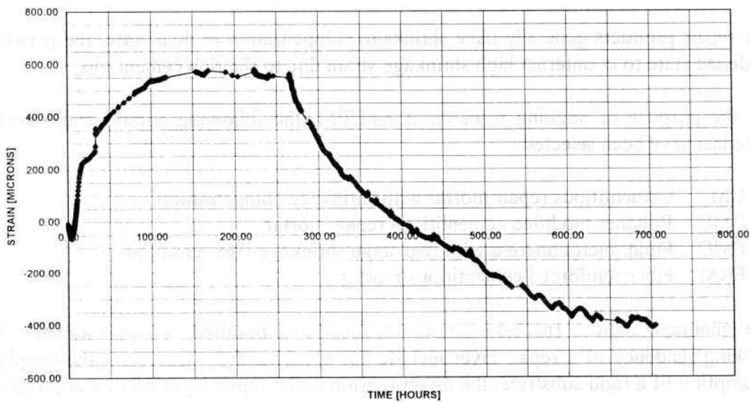
Fig. 3b.  $\epsilon_{sh}$  vs.  $t$  for material PMC (40\*40 mm)
