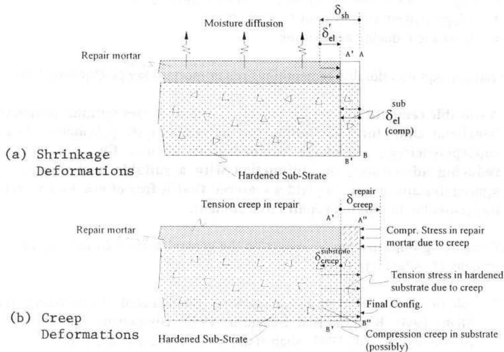
Fig. 1. Restrained shrinkage and creep in patch repair
