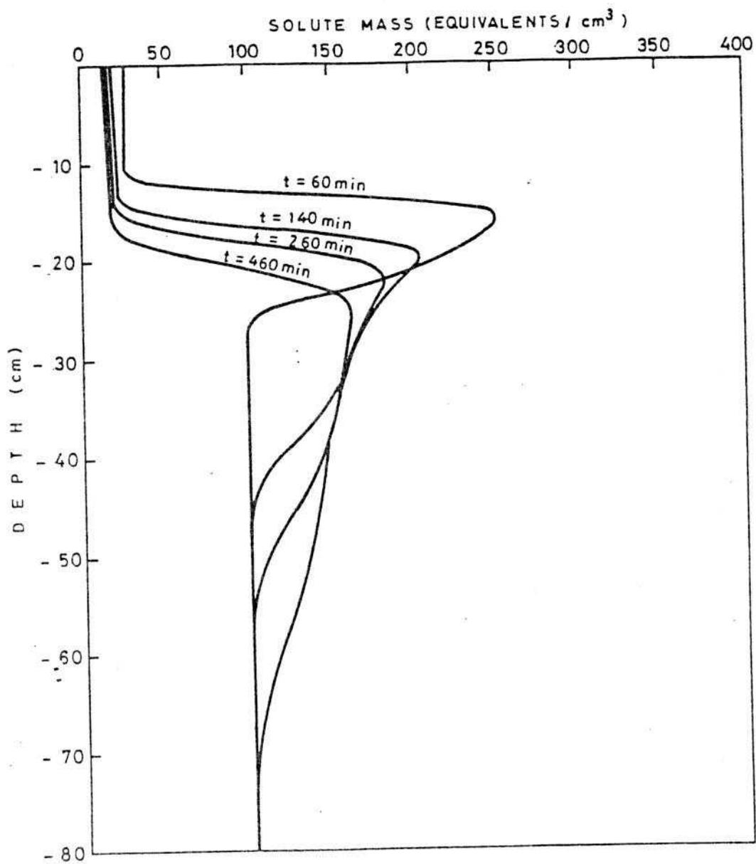
Fig. 6. Numerical solute mass profiles for constant flux vertical infiltration followed by redistribution
