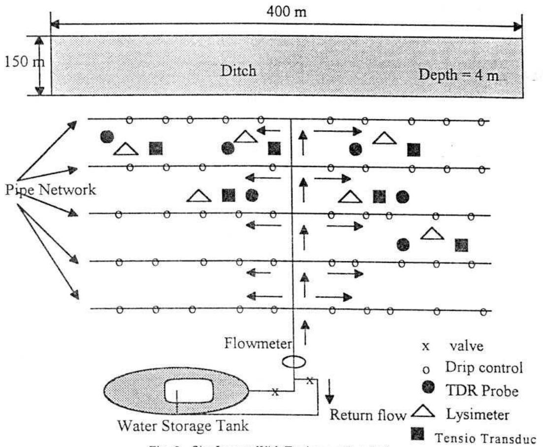
Fig. 2 Site Layout With Equipment Instulation
