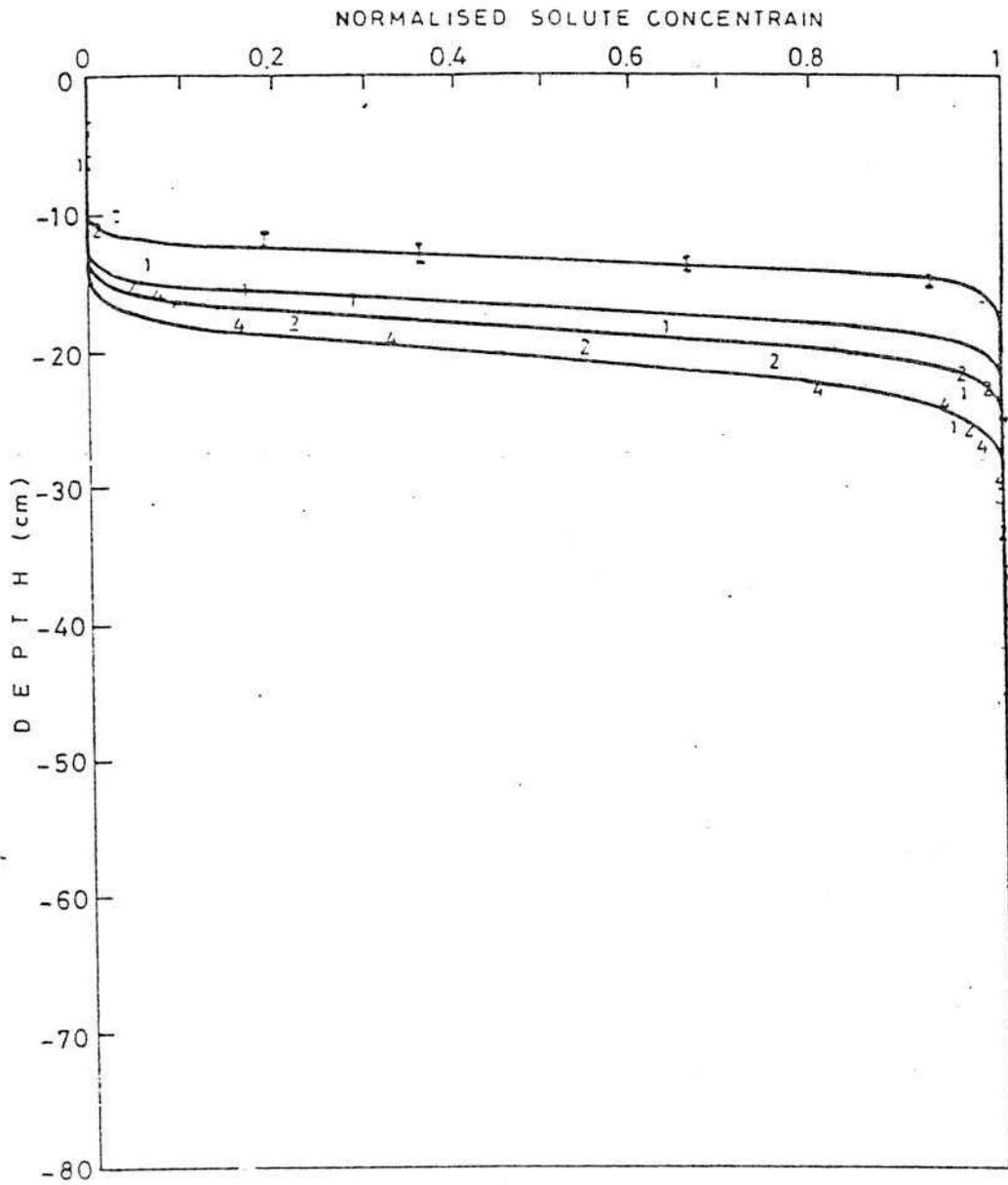
Fig. 4. Experimental and numerical  $\bar{c}(z)$  profiles for constant flux vertical infiltration followed by redistribution (symbols are defined in the text)
