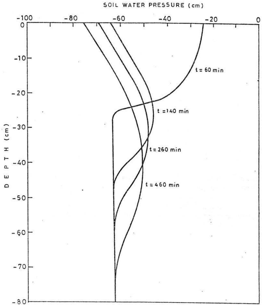
Fig. 5. Numerical  $h(z)$  profiles constant flux vertical infiltration followed by redistribution
