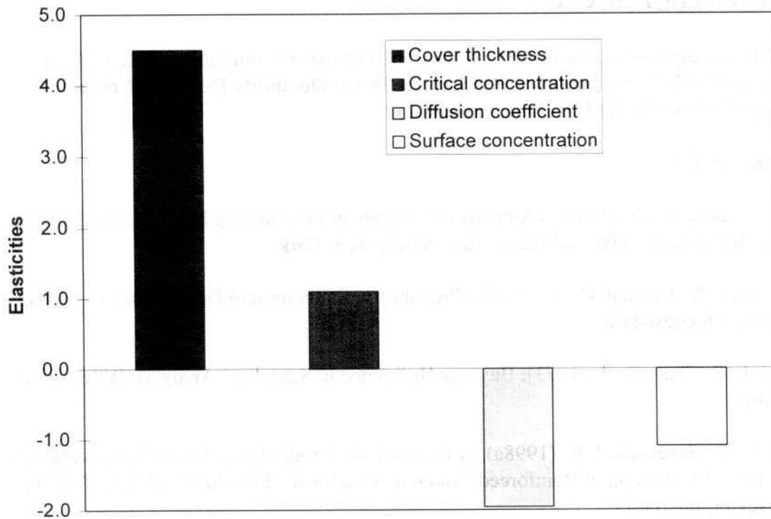
Figure 4: Elasticity of the reliability index with respect to the mean values.
