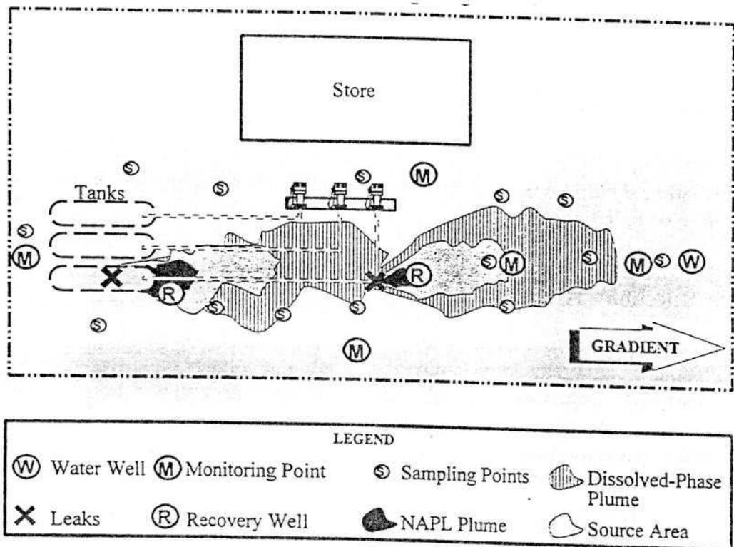
Figure 3. Placement of sampling points. (modified after TNRCC, 1995)
