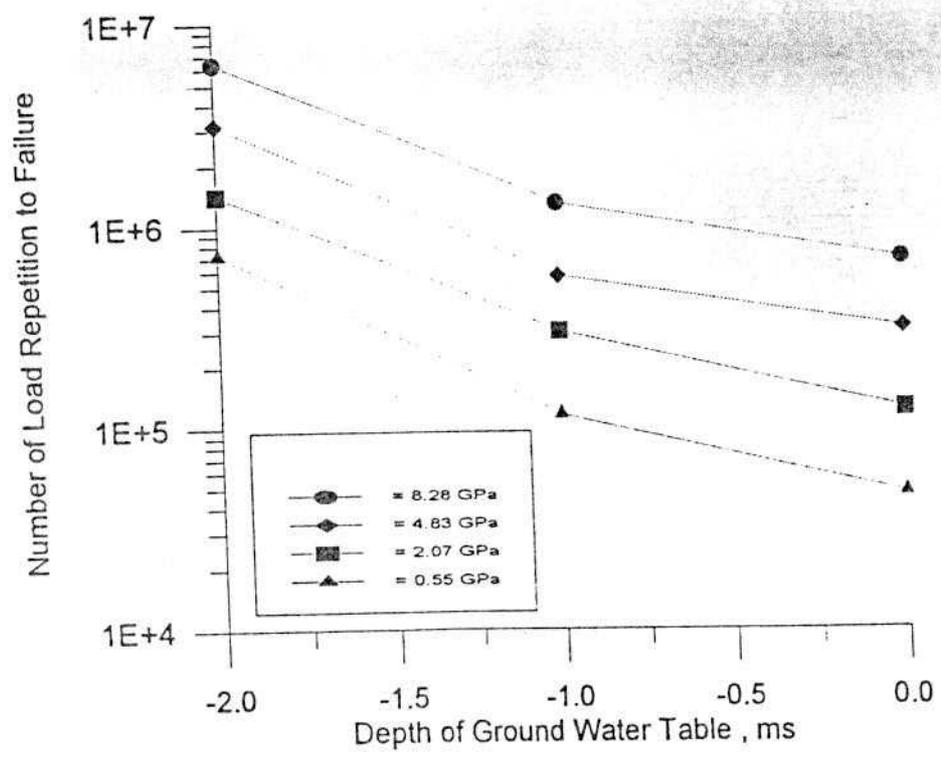
Fig. 11. Relation between  $N_d$  (Rutting) and depth of ground water table for different values of  $|E_1^*|$
