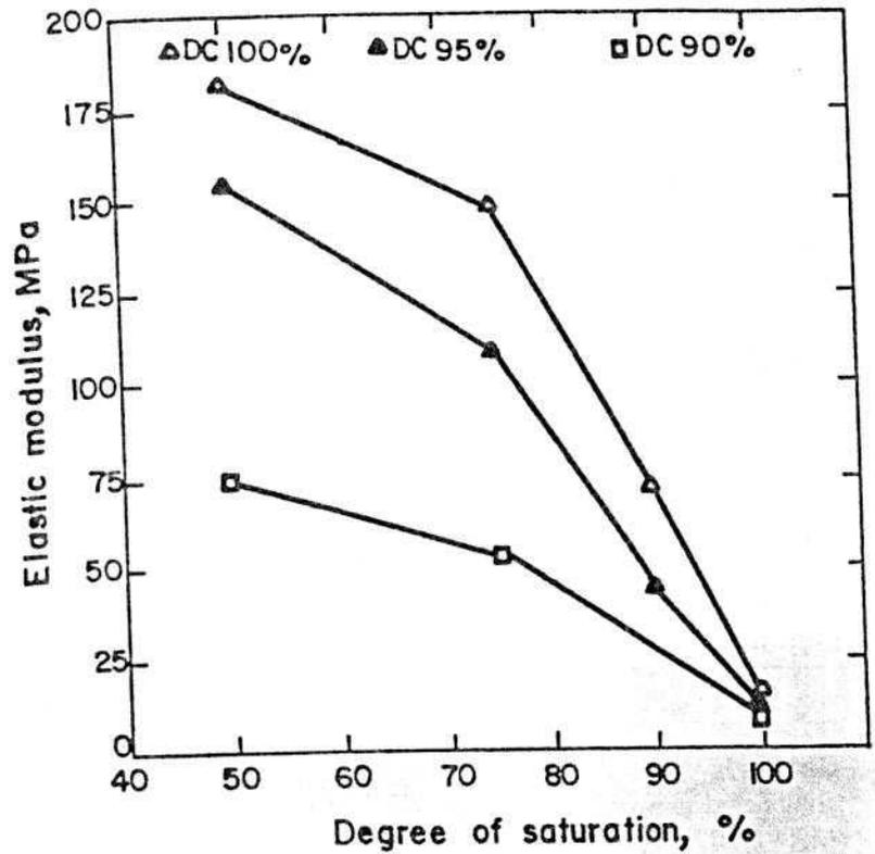
Fig. 7. Effect of degree of saturation on elastic modulus for different degrees of compaction and confining pressures.
