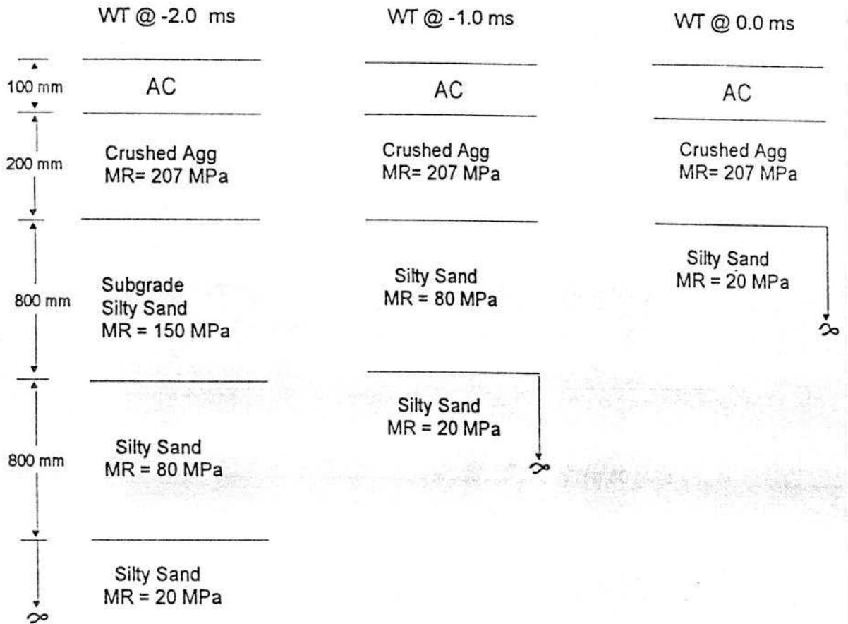
Fig. 9. Details of the pavement cross-sections for different depths to ground water table.
