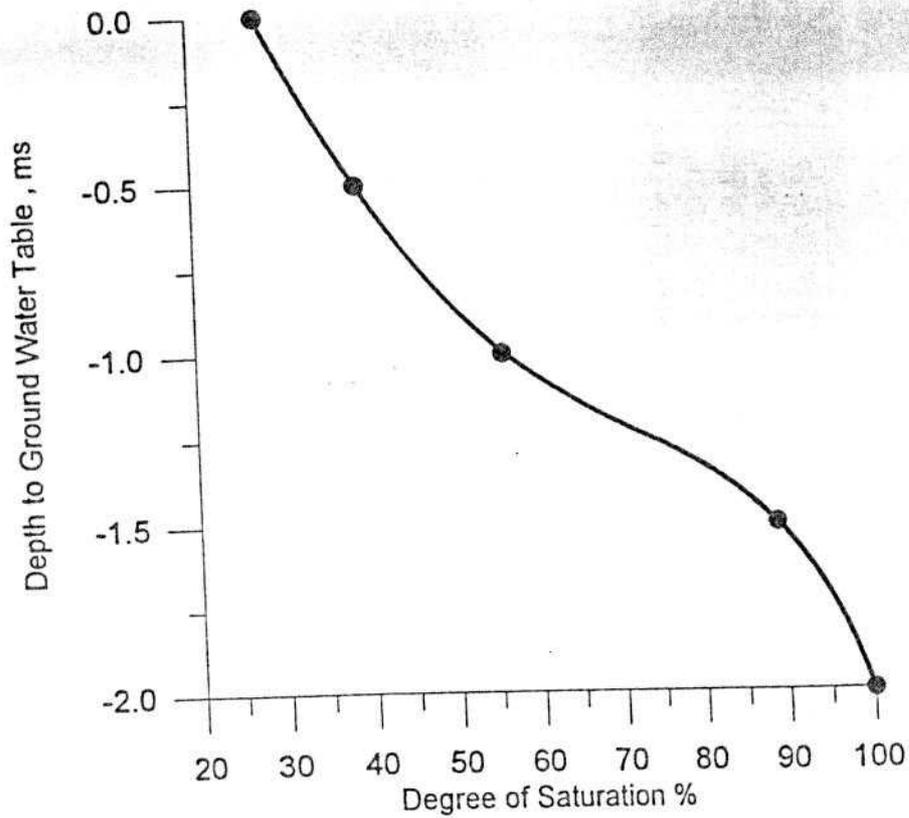
Fig. 8. Distribution of degree of saturation with depth
