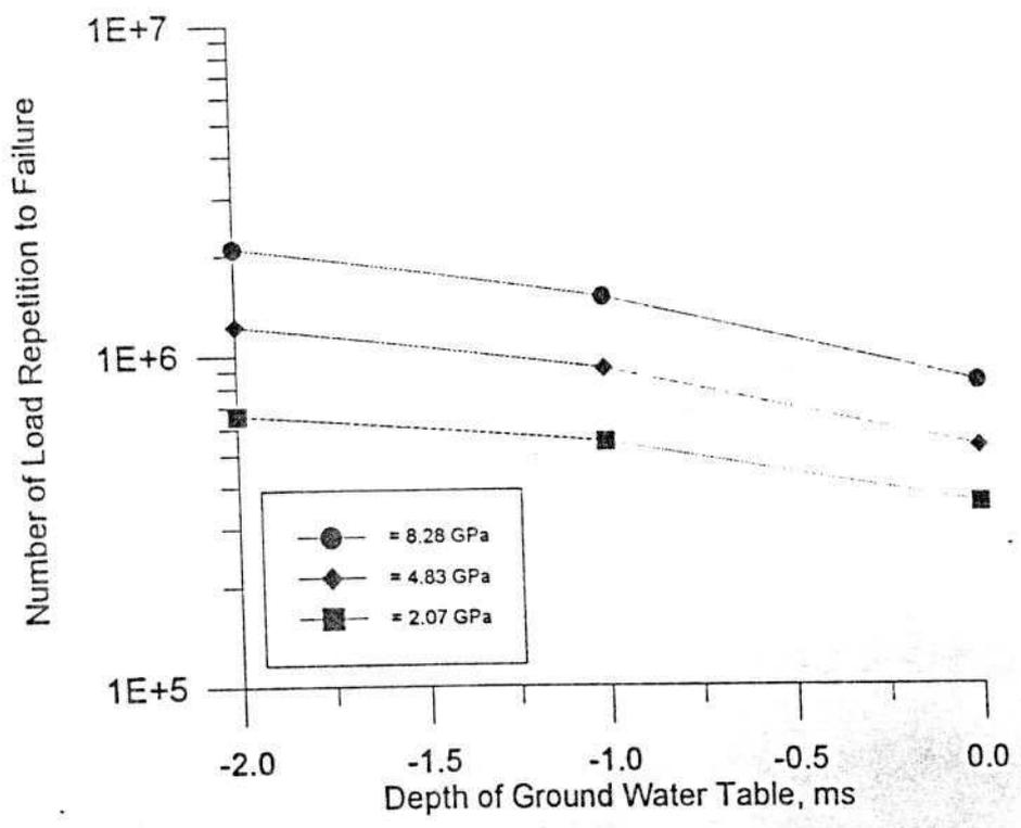
Fig. 10. Relationship between  $N_f$  (fatigue cracking) and depth of ground water table for different values of  $|E_1^*|$
