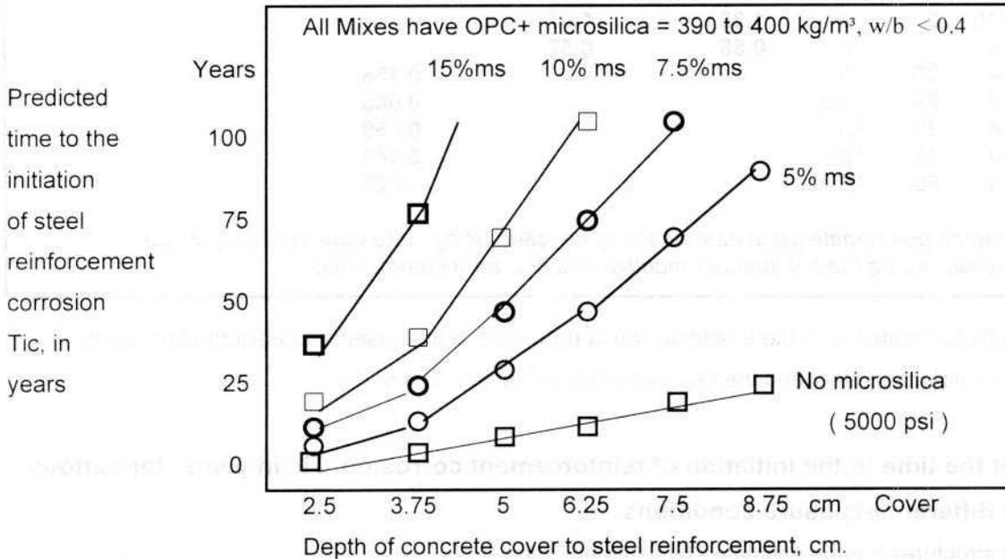
Figure 5. Predicted time to the initiation of corrosion of steel reinforcement, at various covers in concrete under extreme chloride exposure in hot climates, using equations 6, 7, 10 and 11.
