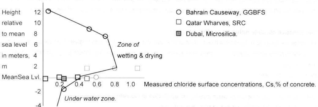
Figure 3. Relation between the location of exposure, and the measured Surface Chloride Level,  $C_s$ , of the concrete in hot marine climates – Extreme exposure [ 16, 17, 18, 19 ].
