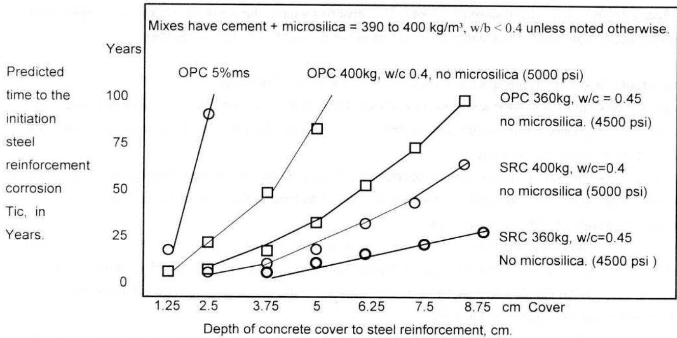
Figure 7. Predicted time to the initiation of corrosion of steel reinforcement, at various covers in concrete under low chloride exposure in hot climates, using equations 6, 7, 10 and 11.
