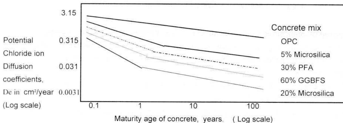
Figure 4. Time related reduction in the chloride-ion diffusion coefficients for concrete containing pozzolans over the design life of a concrete structure [ 12,24 ].
