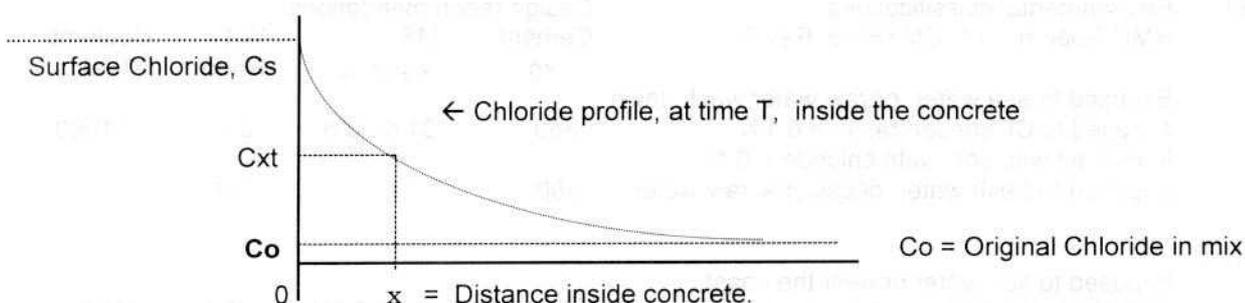
Figure 2. Relation between Chloride concentration and distance from concrete surface, The chloride profile calculated using Fick's Second Law [ 15].
