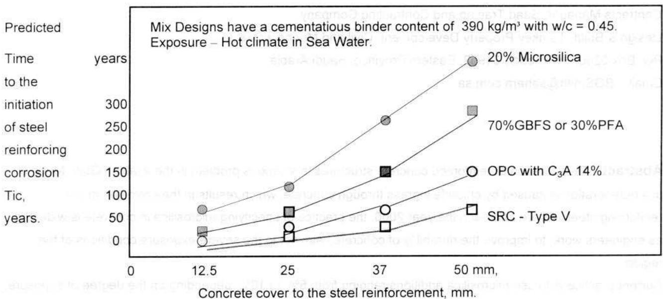
Figure 1. Predicted time to the initiation of reinforcement corrosion, at various covers for concrete made with SRC, OPC, and OPC modified with PFA, GGBFS and microsilica under severe chloride exposure [2].
