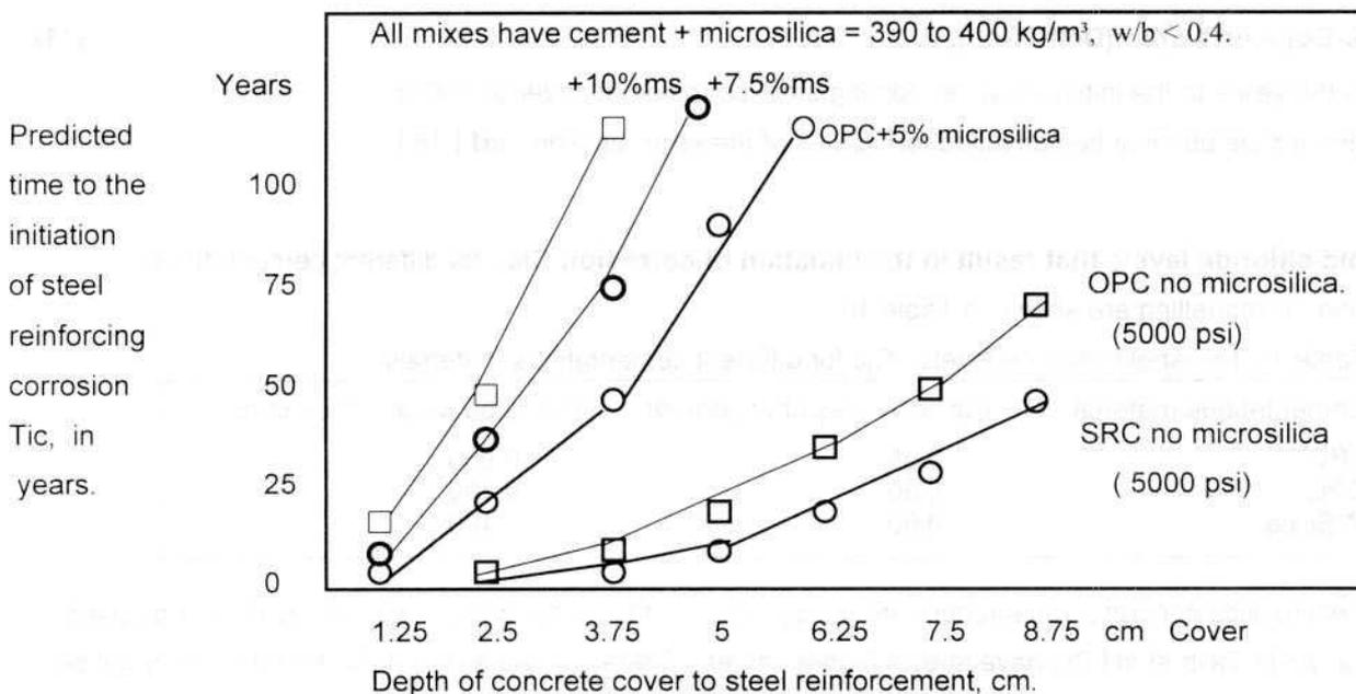
Figure 6 Predicted time to the initiation of corrosion of steel reinforcement, at various covers in concrete, under moderate chloride exposure in hot climates, using equations 6, 7, 10 and 11.
