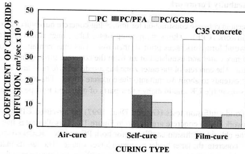
Fig. 8. Chloride diffusion of self-cure concrete
