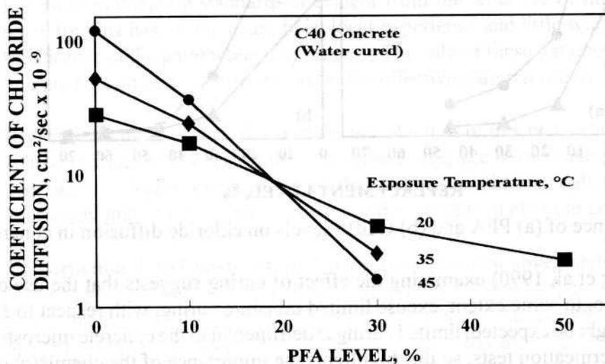
Fig. 4. Influence of exposure temperature on chloride diffusion in concrete
