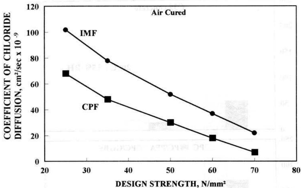
Fig.10. Influence of CPF on chloride diffusion in concrete
