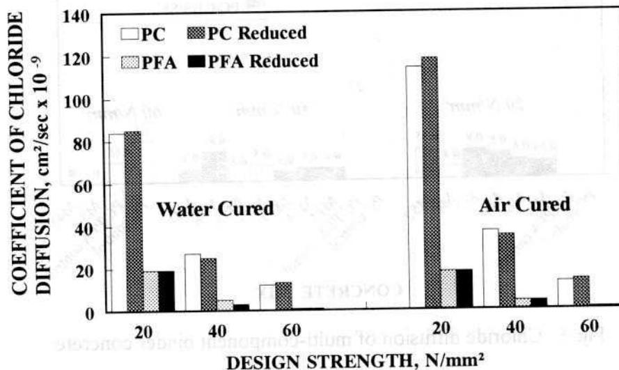
Fig.6. Chloride diffusion coefficients of binder reduced concrete
