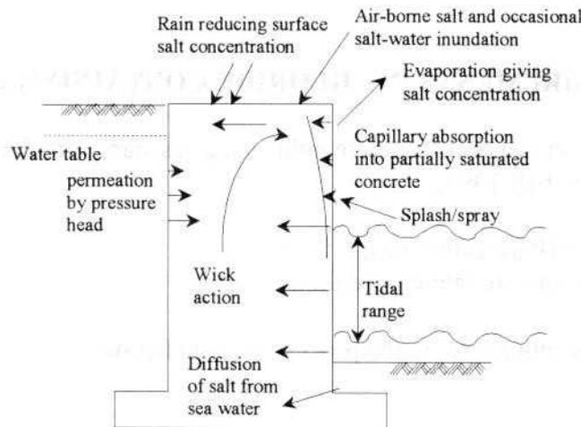
Fig 1. Mechanisms of chloride ingress into concrete (Concrete Society, 1996)
