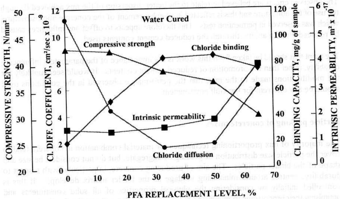
Fig. 7. Influence of various factors on chloride diffusion in PFA concrete proportioned using particle packing method
