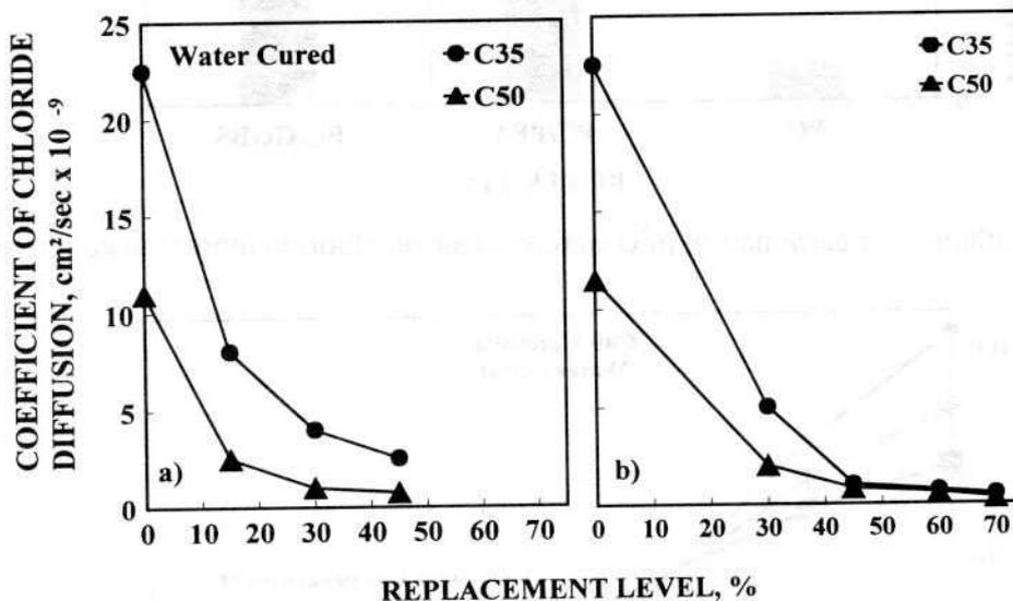
Fig.2. Influence of (a) PFA and (b) GGBS levels on chloride diffusion in concrete
