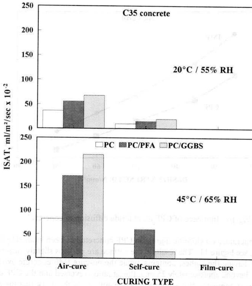
Fig.9. Effect of temperature on ISA of self-cure concrete
