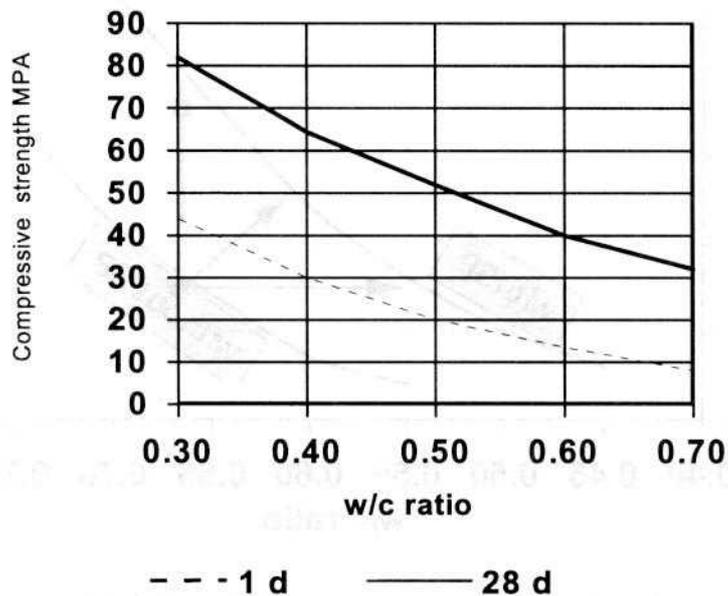
Figure 3. Correlation between w/c and compressive strength
