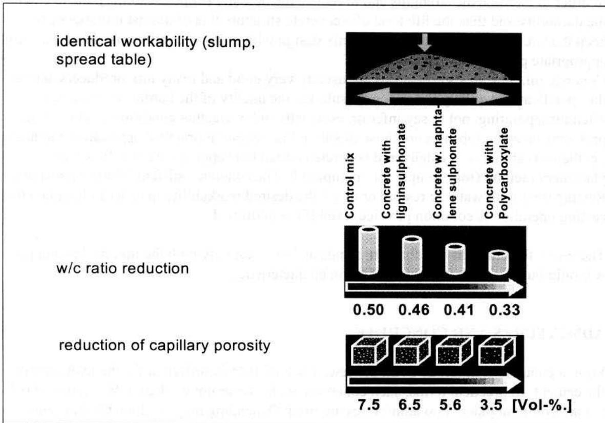
Figure 2. Correlation between w/c and porosity
