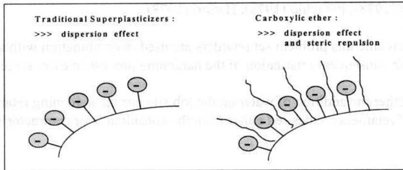
Figure 5. Mechanism of action of superplasticizers molecules
