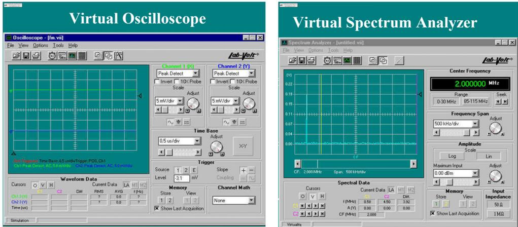
Figure 3(a): Front panel of a virtual Oscilloscope & Spectrum Analyzer used in EE labs.
