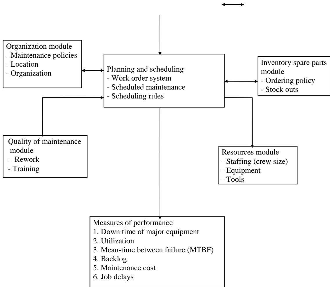
Figure 3. Elements of an Integrated Simulation Model for Maintenance
