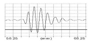
Figure 4: A snapshot of the flaw detector screen showing one HTHA defect
