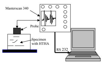
Figure 2: Data acquisition system used
