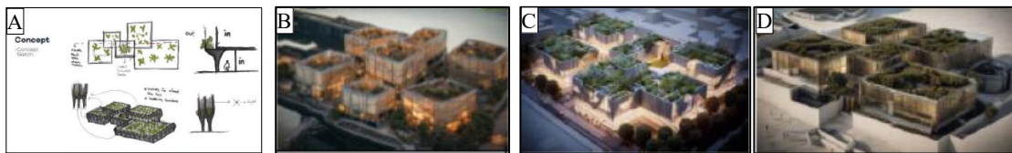
Figure 2.20: A. Initial concept: Sketches develop into a conceptual model; B. Development: The concept evolves into a detailed 3D model; C. Enhancement: The model is refined with realistic textures and lighting; D. Final rendering: The completed design features sustainable elements like green roofs.
