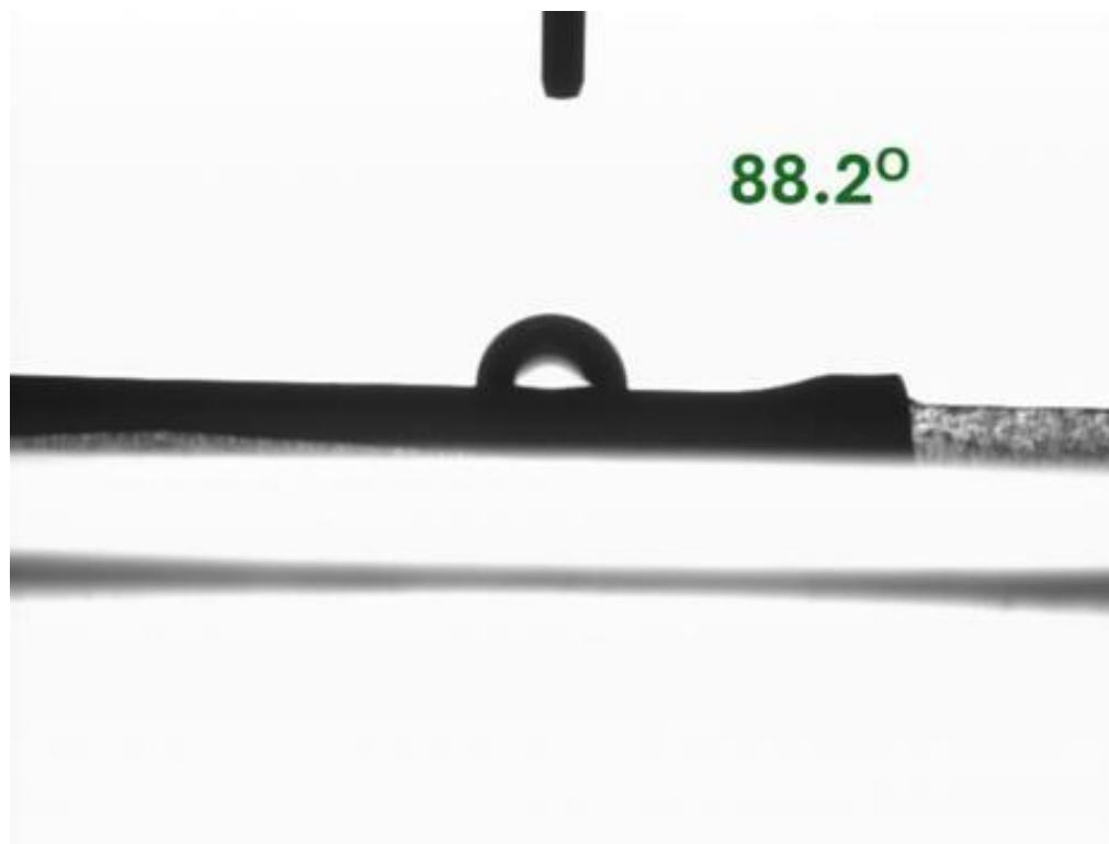
Figure 5.6: WCA obtained from glass substrate cast PVDF membrane.
