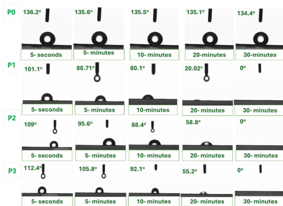
Figure 3.8: Surface wettability analysis of pristine membrane P0 and Janus membranes P1, P2 and P3.
