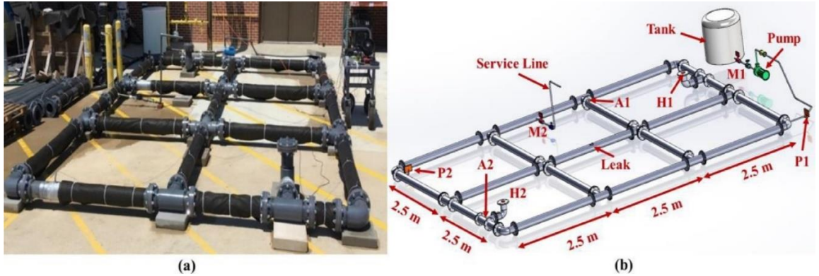
Figure 3.1: Experimental layout of looped WDS topology in the laboratory where (a) real-time perspective view (b) schematic view.
