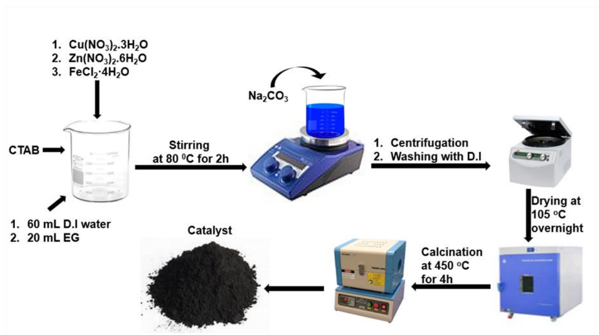
Figure 4 Schematic representation of the catalyst preparation
