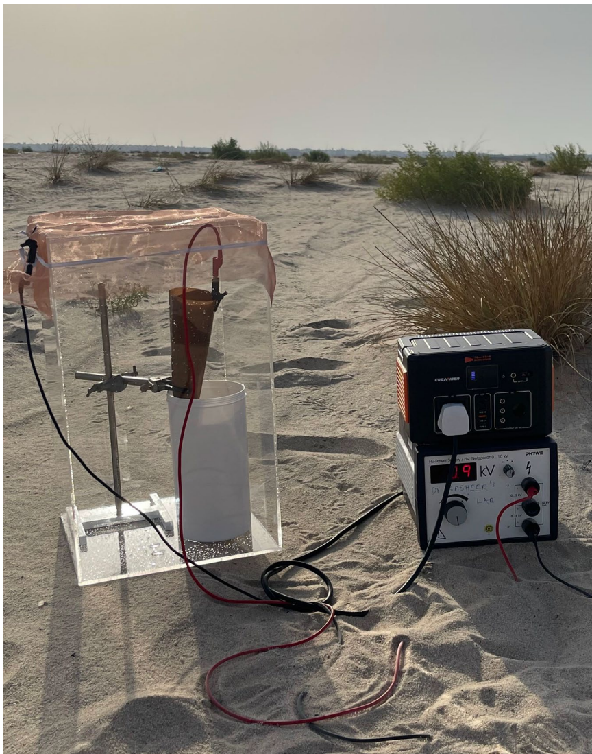
Figure 28. Experimental setup of the electrostatic fog harvesting system deployed in an arid field environment. The apparatus features a high-voltage power supply connected to an electrode within a transparent acrylic chamber, which is designed to isolate the system and direct charged fog droplets toward the collection vessel.
