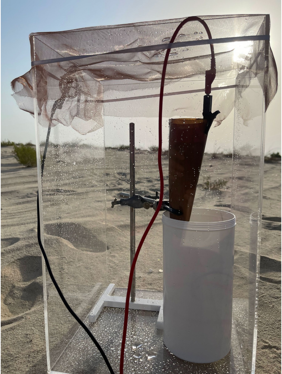
Figure 29. Collected fog droplets condensing on the inner chamber surface and beginning to accumulate in the collection vessel.
