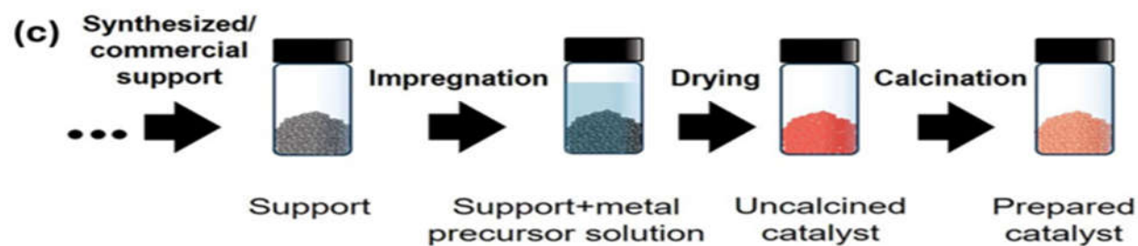
Figure 2.7: Different catalyst synthesis method (a) Sol-gel method adapted from [70] (b) Co-precipitation [67] (c) Impregnation[49].
