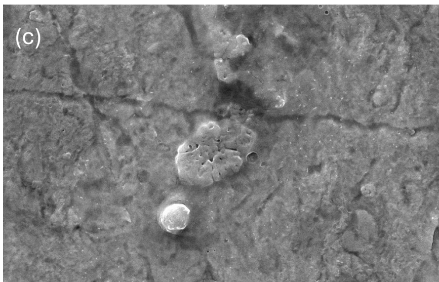
Figure 3. 15 SEM images of the bare carbon steel (a) after 24h immersion in 1m HCl-3.5% NaCl solutions in the absence (b) and presence of 30 ppm PAS/N-ACs (c)
