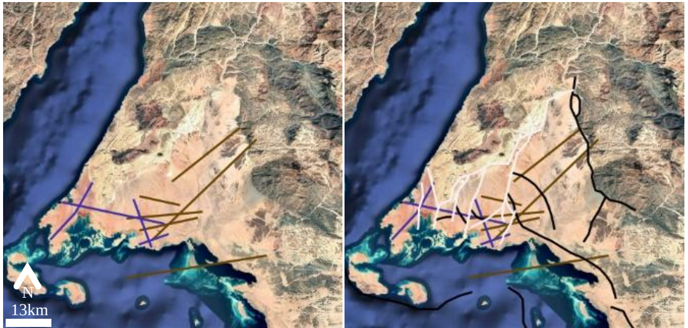
[Figure 35 (left) all the available seismic we used. (right) picked faults in map view incorporating interpretation from seismic, outcrop, and satellite image. Strike-slip faults were picked in white, and rift faults are picked in black.]
