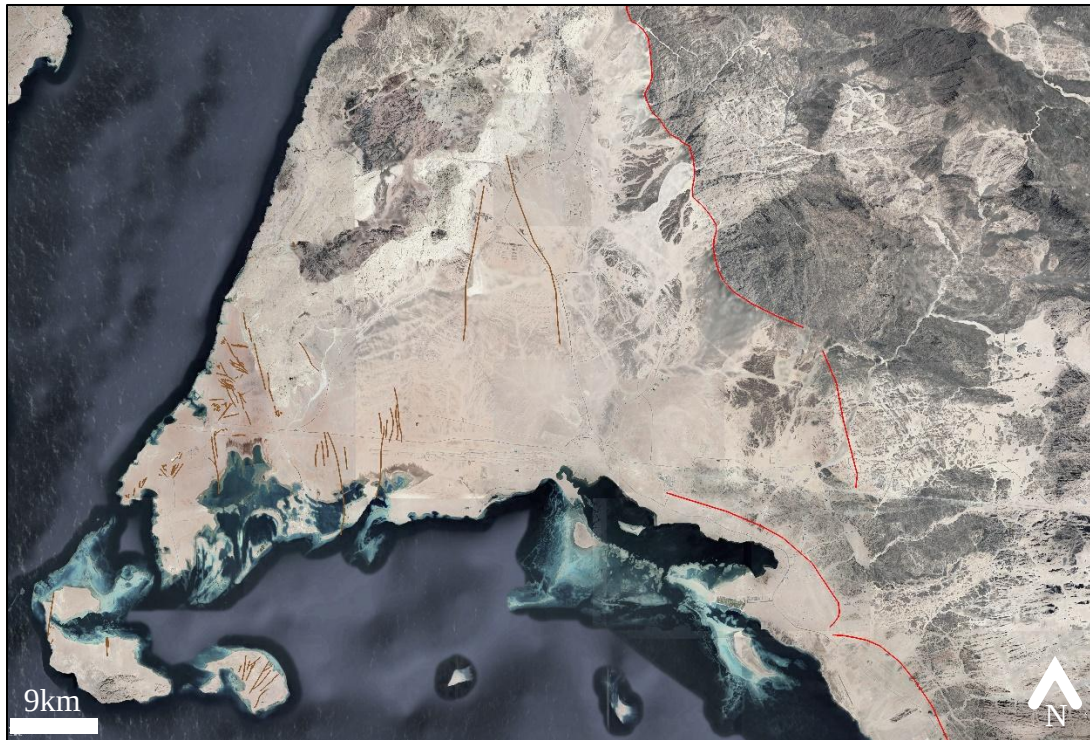
Figure 12 satellite image with rift faults in red, and strike-slip faults in brown
