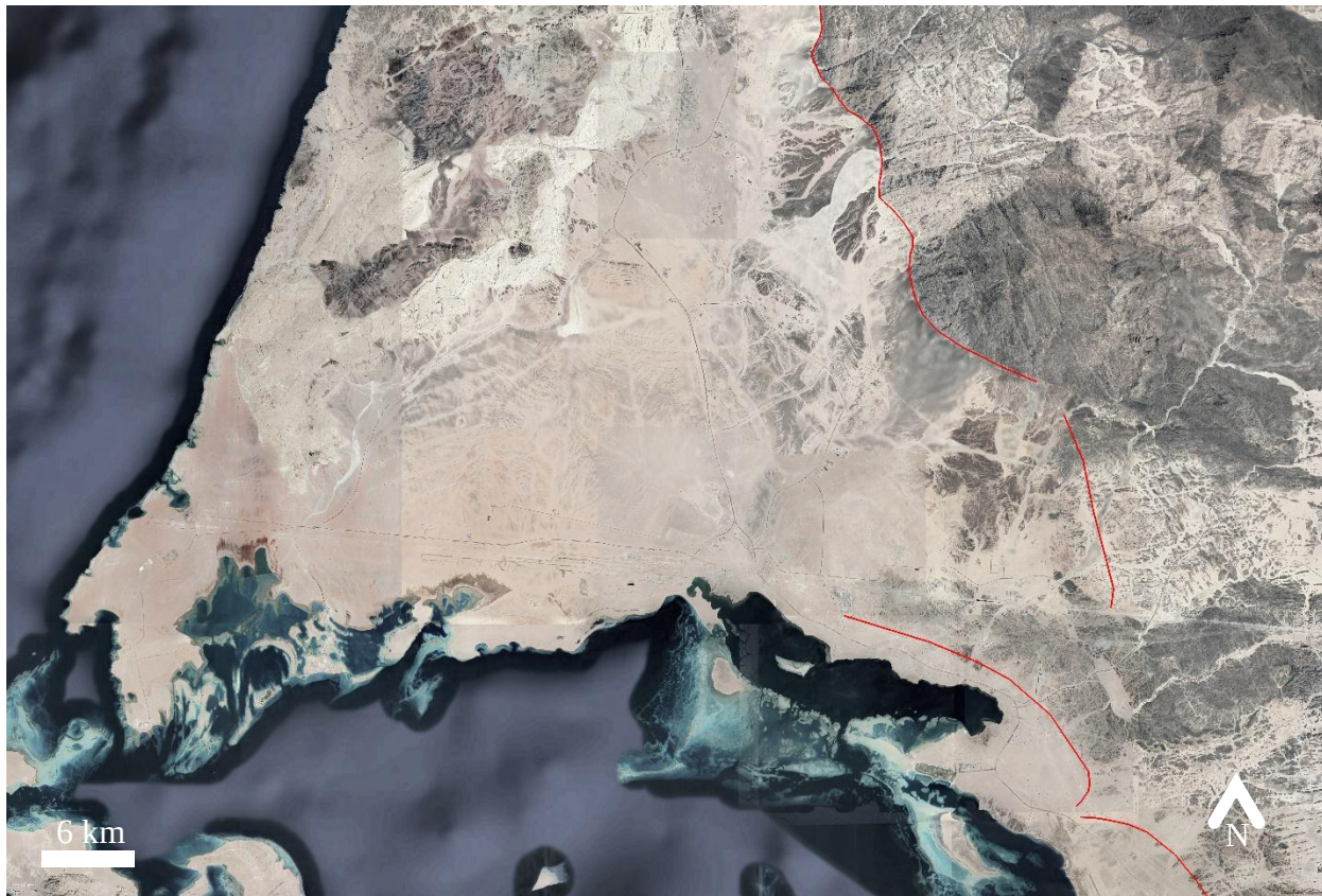
Figure 8 Satellite image with picked rift faults in red
