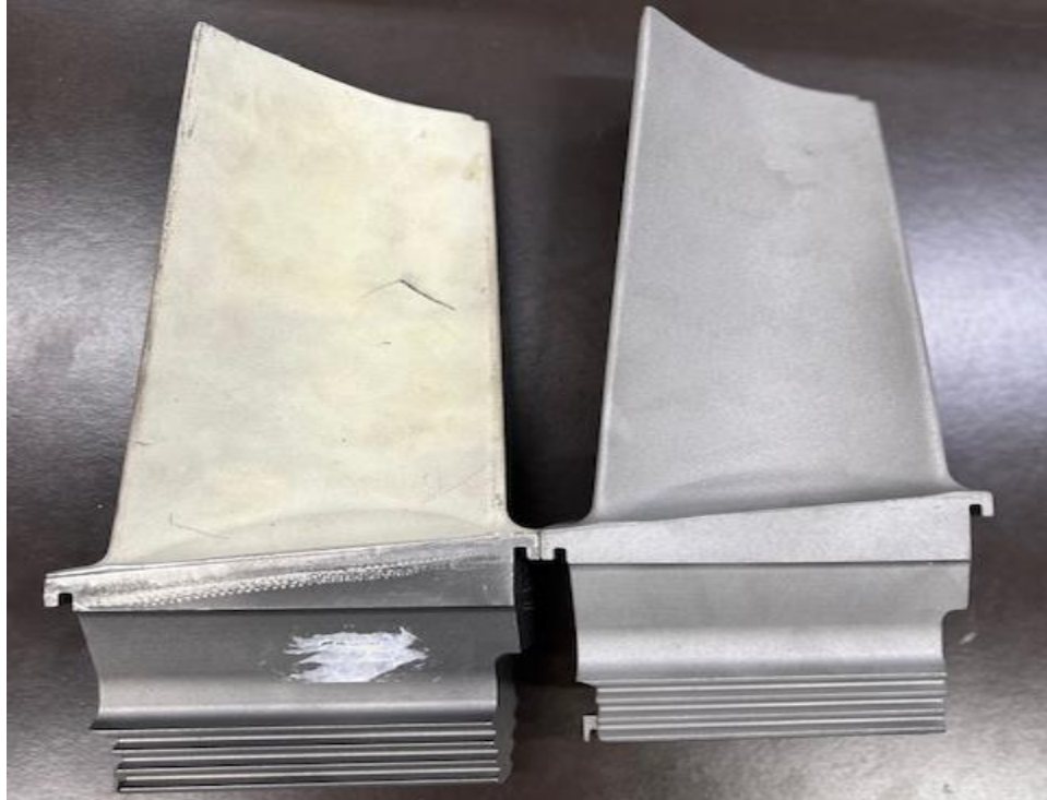
Fig. 28. IN738 base metal - Gas turbine blades.
