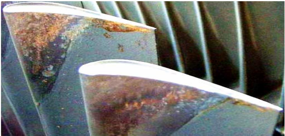
Fig.6. Turbine blades experiencing erosion-induced damage[19].
