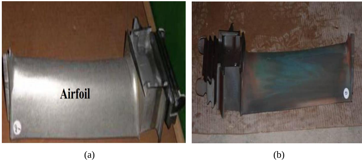
Fig. 4. (a) Healthy blade and (b) Same blade after 24K EOH.[14]
