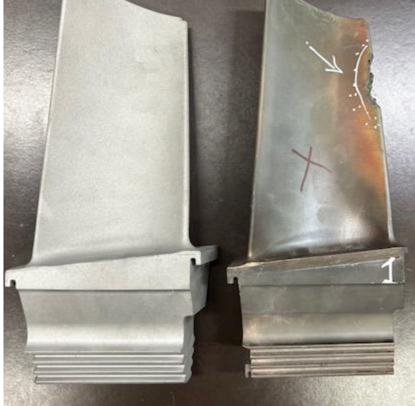
Fig. 32. Healthy and Cracked -IN738 base metal - Gas turbine blades.
