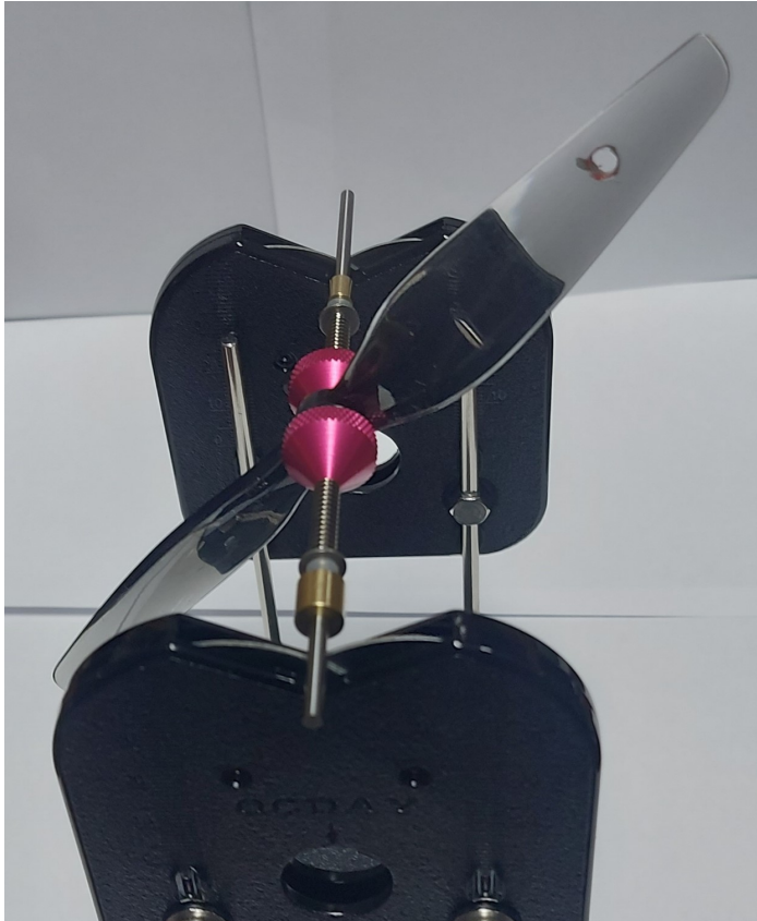
Figure 3.10: An unbalanced propeller tilts towards the heavier side when placed on the Hobby Fans Tru-Spin propeller balancer, revealing mass asymmetry that must be corrected.
