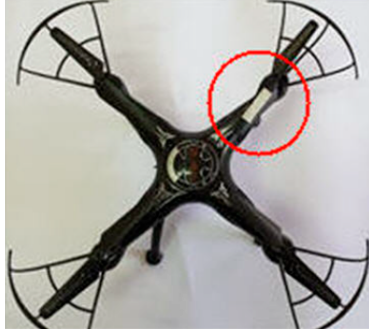
(c) Texture addition using tape [41].
