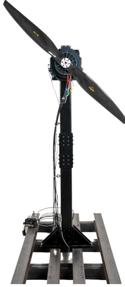
Figure 3.13: Tytorobotics Flight Stand 15, a precision measurement system for UAV propulsion testing [74].
