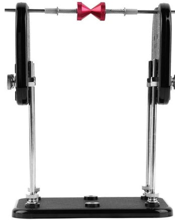
Figure 3.8: The Hobby Fans Tru-Spin Propeller Balancer used to assess and correct propeller balance. The low-friction pivot system allows precise detection of mass asymmetry.
