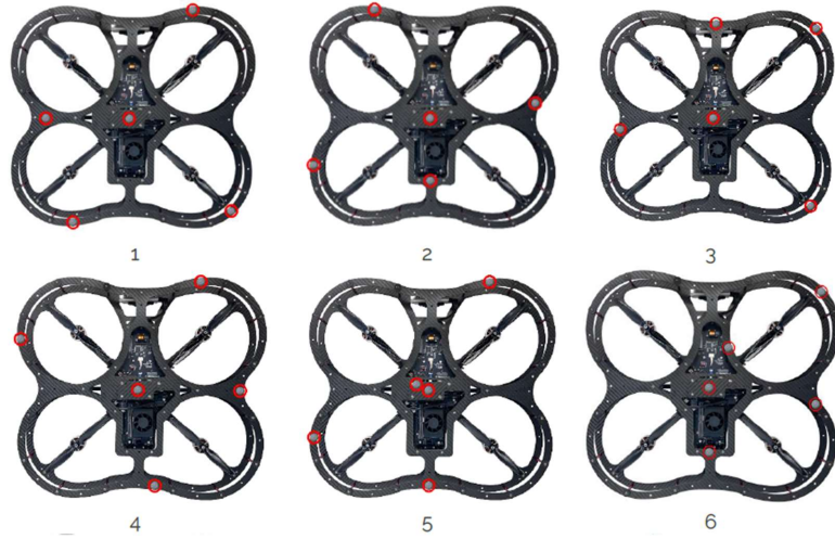
Figure 2.2: Sample unique marker configurations on QDrone 2 used to avoid symmetrical ambiguities, ensuring accurate pose estimation.
