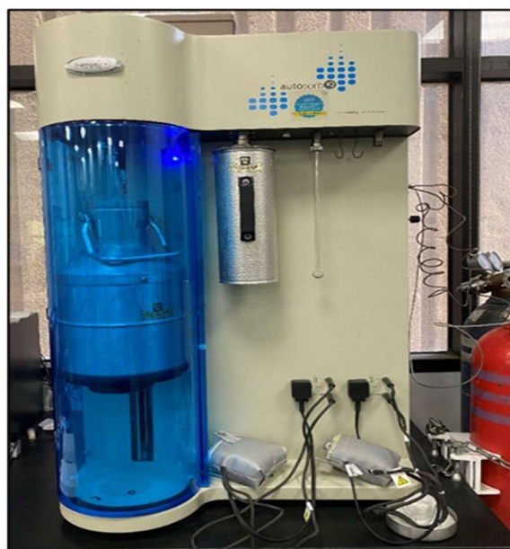
Figure 6- Quantachrome Aquasorb iQ BET instrument.
