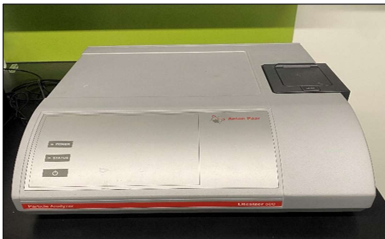
Figure 3- Zeta potential instrument used in the study.
