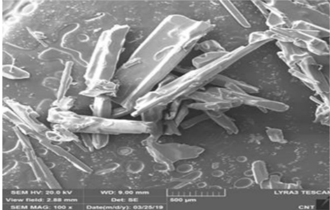
Figure 4.2: SEM image of \text{KNO}_3 crystals grown conventionally without laser after 12 min [1].
