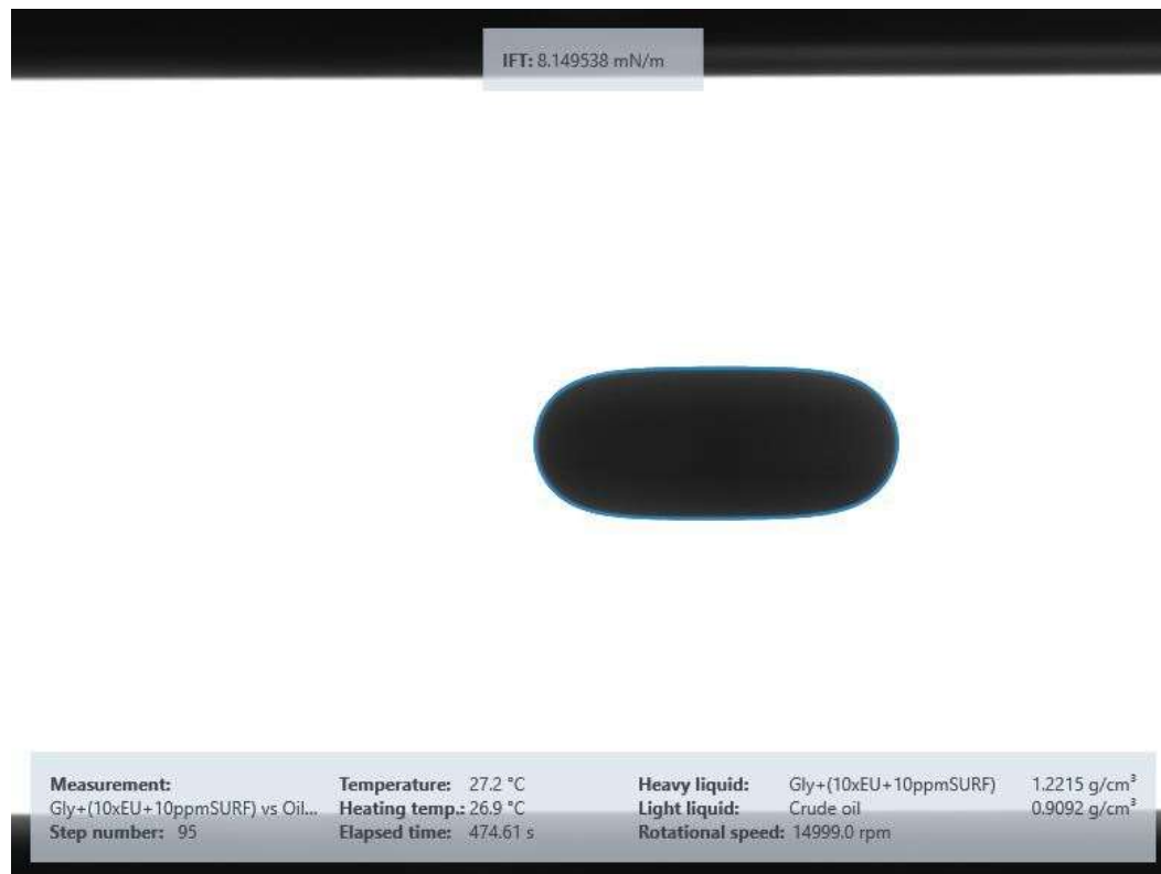
Figure 17: IFT Measurement and Observation for Surfactant Glycerol solution
