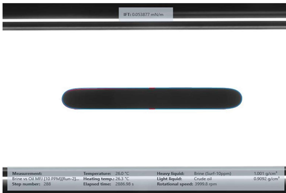
Figure 14: IFT Measurement and Observation for EU Brine at 10ppm Surfactant
