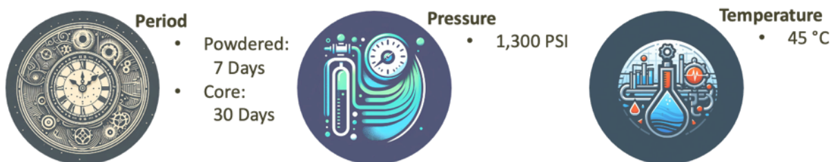
Figure 11. CO 2 Treatment Conditions for both the powdered and core sample
