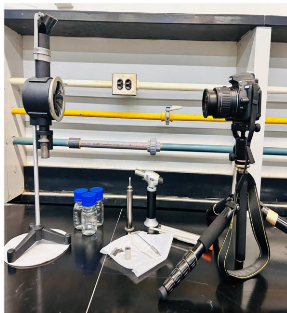
Figure 3.2: Apparatus setup for SP Measurement, ASTM D1322
