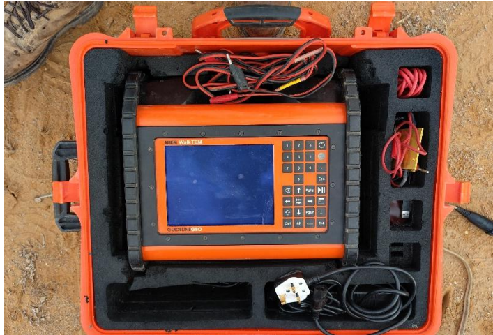
Figure 4.3 Showing TEM device that use the conducting the measurement
