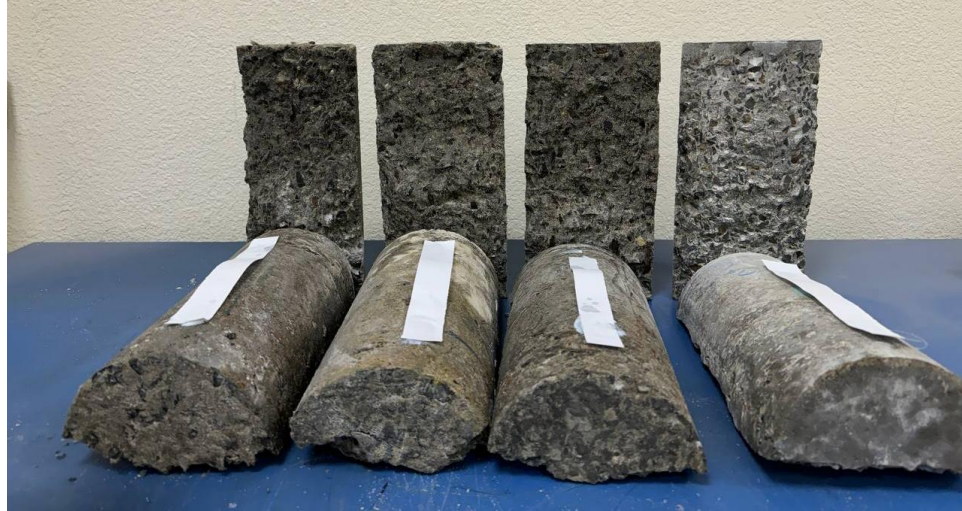
Figure 50 Tested BFR-SSSC specimens with different BF content.
