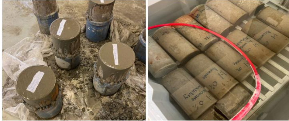
Figure 26 Casted concrete in the molds (left). Submerged concrete specimens in tap water (right).
