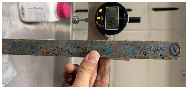
Figure 25 BFR-SSSM drying shrinkage specimen.
