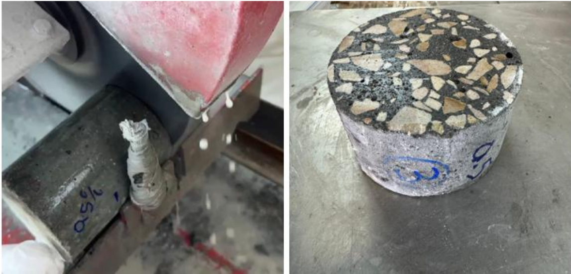
Figure 36 Water absorption BFR-SSSC specimens' discs preparation.
