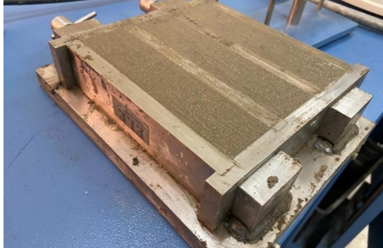
Figure 24 Molded mortar specimens for flexural strength test.
