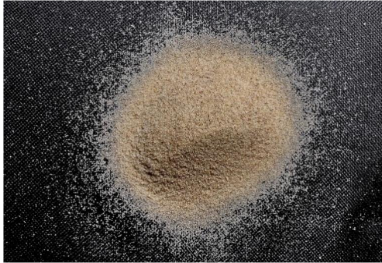
Figure 18 Sea sand is used in the mix as fine aggregate.
