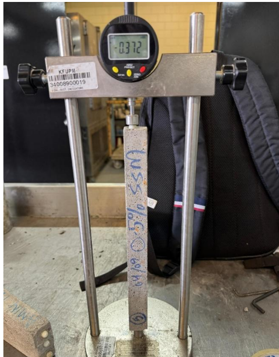
Figure 38 Measurement of drying shrinkage of BFR-SSSM.
