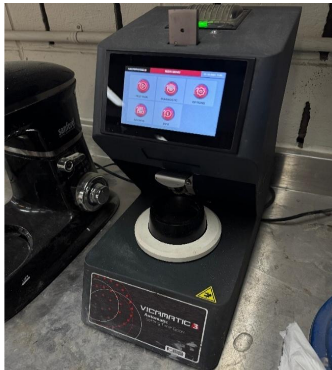
Figure 28 Automatic Vicat apparatus device used to measure initial and final setting time.
