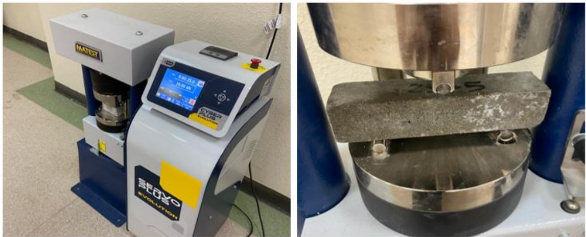
Figure 33 BFR-SSSM specimen placed in a three-point loading machine according to ASTM C348.
