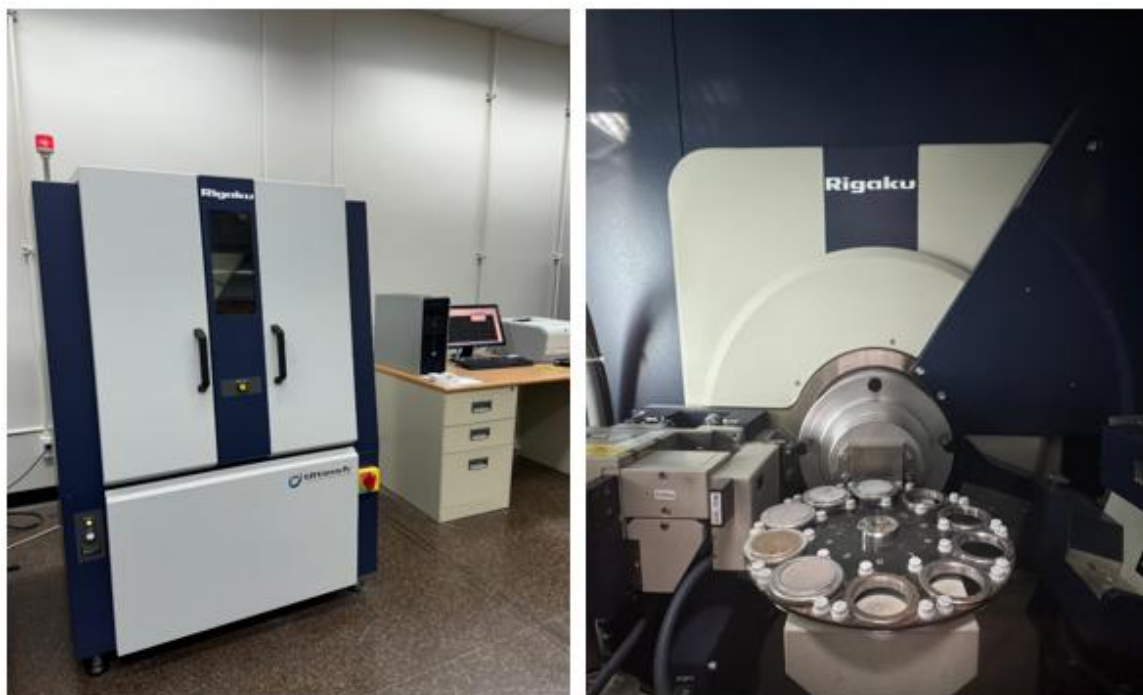
Figure 40 XRD instrument (left). SSSC and SSSM sample placement inside XRD analysis instrument (right).
