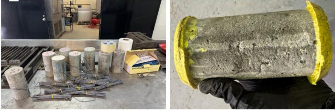
Figure 29 Strain gauges attaching to the cylindrical concrete samples (left). Capping of the samples (right).
