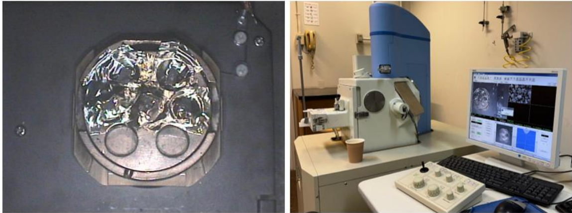
Figure 39 Placement of specimens plated with gold sheets in SEM-EDS instrument (left). SEM-EDS instrument (right).
