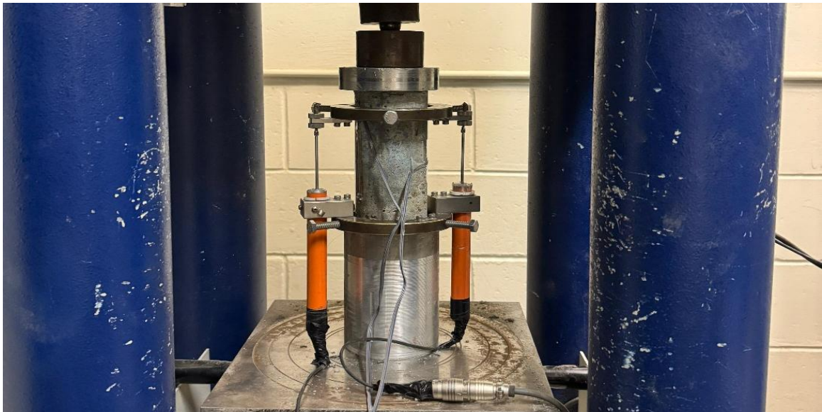
Figure 30 BFR-SSSC cylindrical sample under compression testing.
