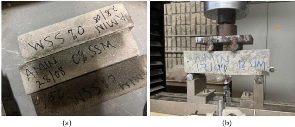
Figure 31 BFR-SSSC beam surface-dried specimens (a). BFR-SSSC beam specimen under loading (b).
