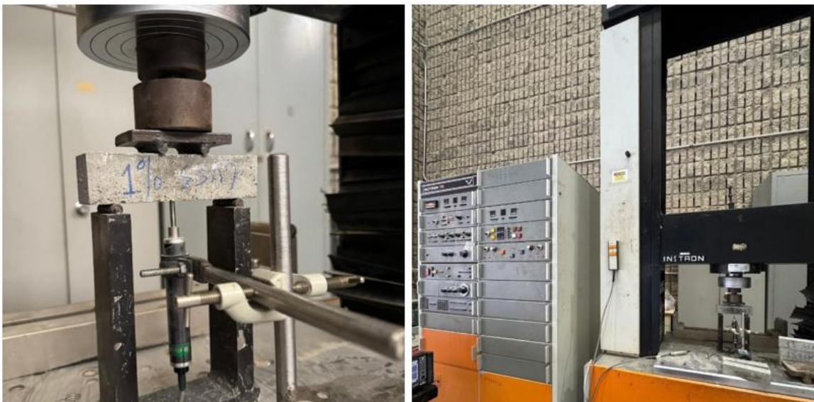
Figure 34 BFR-SSSM specimen placed in a four-point loading machine according to ASTM C78.
