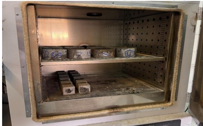
Figure 37 BFR-SSSC water absorption specimens placed in oven for 72 hours.
