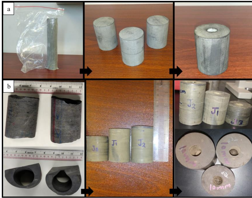
Figure 4 Preparation of (a) Shale samples and (b) Organic-rich Jordan Carbonate
