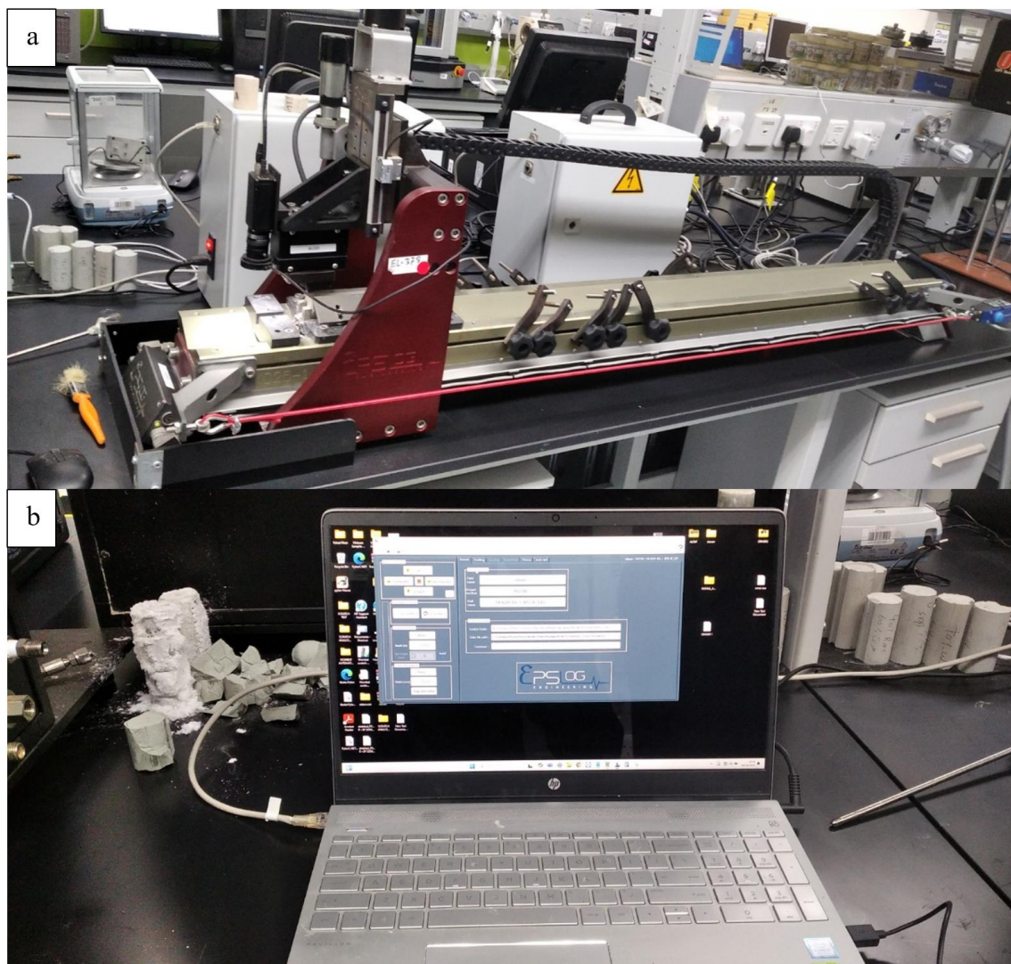
Figure 12 (a) scratch test equipment and (b) Scratch analysis computer device
