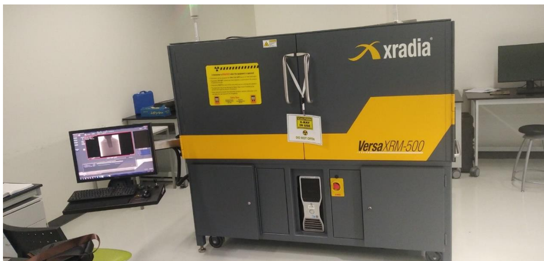
Figure 6 Micro-CT scan device setup
