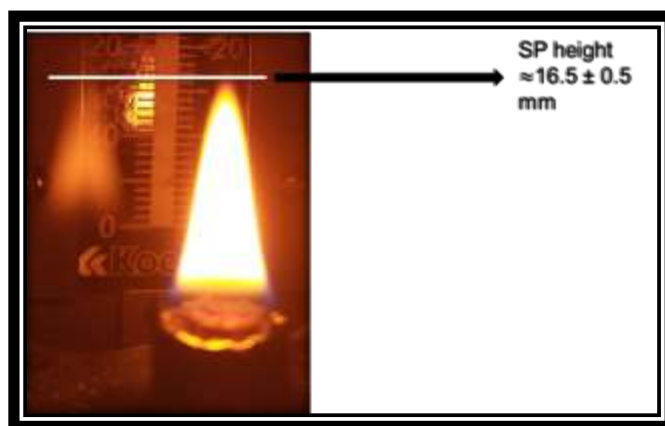
Fig. 2. SP measurement of fuel blend consisting of diphenyl ether (20%) and diesel (80%) by volume.
