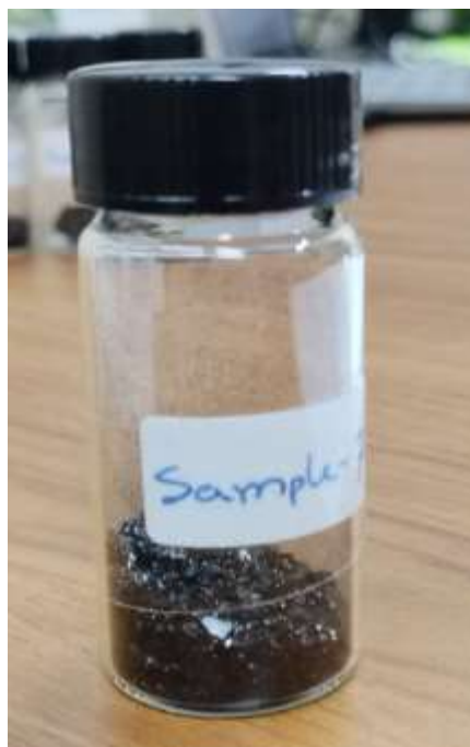
Figure 43. Asphaltenes from Oxidized HVGO + 5 % tetralin, 190°C.
