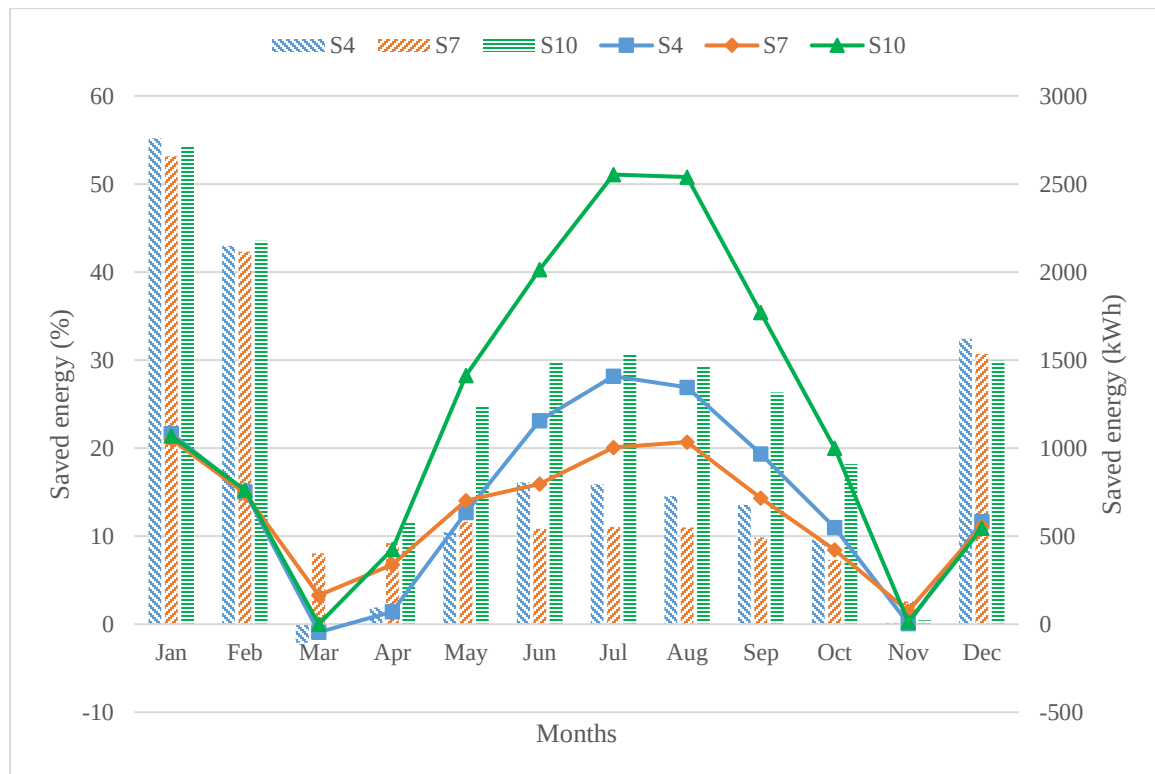
Figure 15: Energy savings from external insulation scenarios with inclusion of window glazing upgrades only
