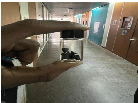
Figure 13. GO synthesized by modified Hummer's method
