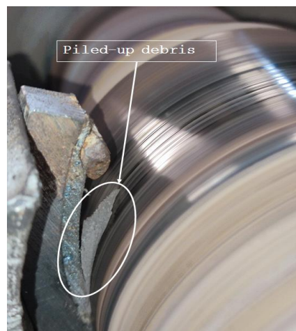
Figure 34: Photograph of the debris accumulated during the dry friction test.
