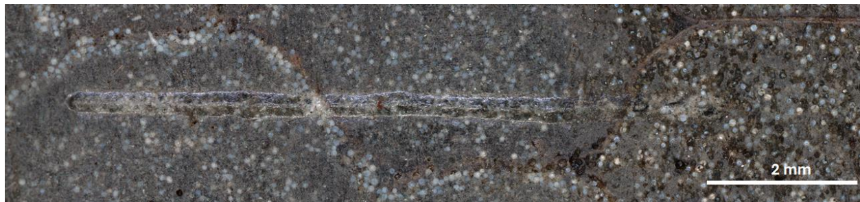
Figure 13: Digital microscopic image for constant load scratch test.
