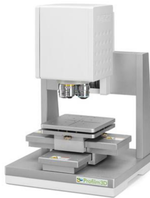
Figure 3: Profilm 3D optical profilometer.
