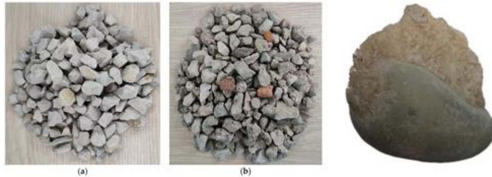
Figure 2. (a) Virgin aggregate (b) Recycled concrete aggregate (c) Typical RAC. [9]
