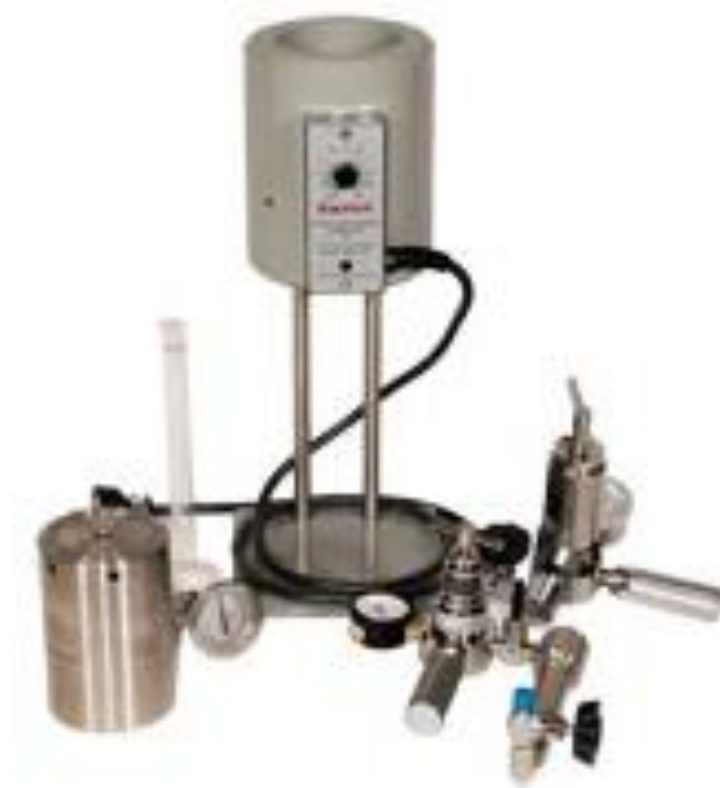
Figure 3.2: A high-temperature high pressure fluid loss system using filter paper
