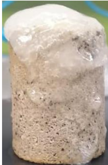
Figure 4.4: An example of poor filter cake during filtration experiment due to absence of particle additives
