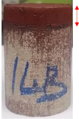
Figure 4.15: The high permeable sample with the filter cake formed after the filtration experiment
