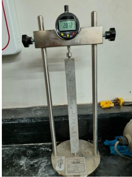
Fig. 15. Length comparator setup for drying shrinkage
