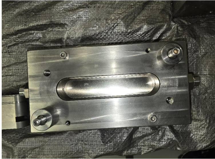
Figure 18. Metal sheet placed in API cell
