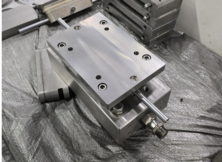
Figure 16. Assembled bottom part of API cell
