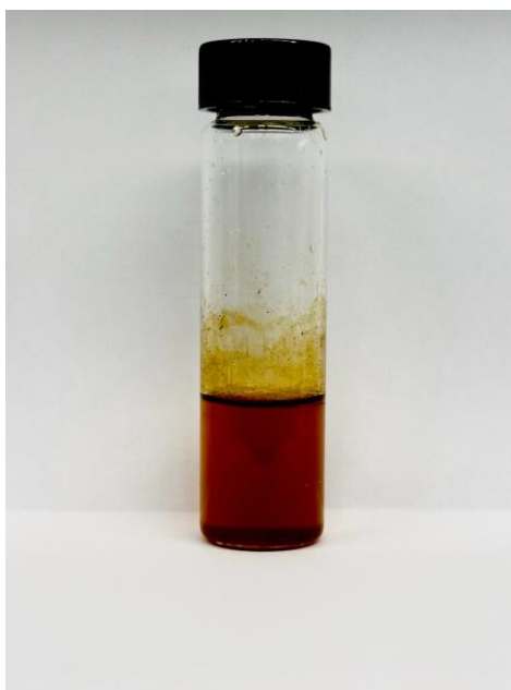
Figure 21: Sample of the collected effluents of core flooding following TCF treatment.
